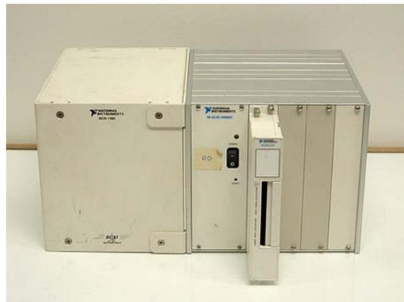
Figure 6.11 Data acquisition chassis configuration used on barge
