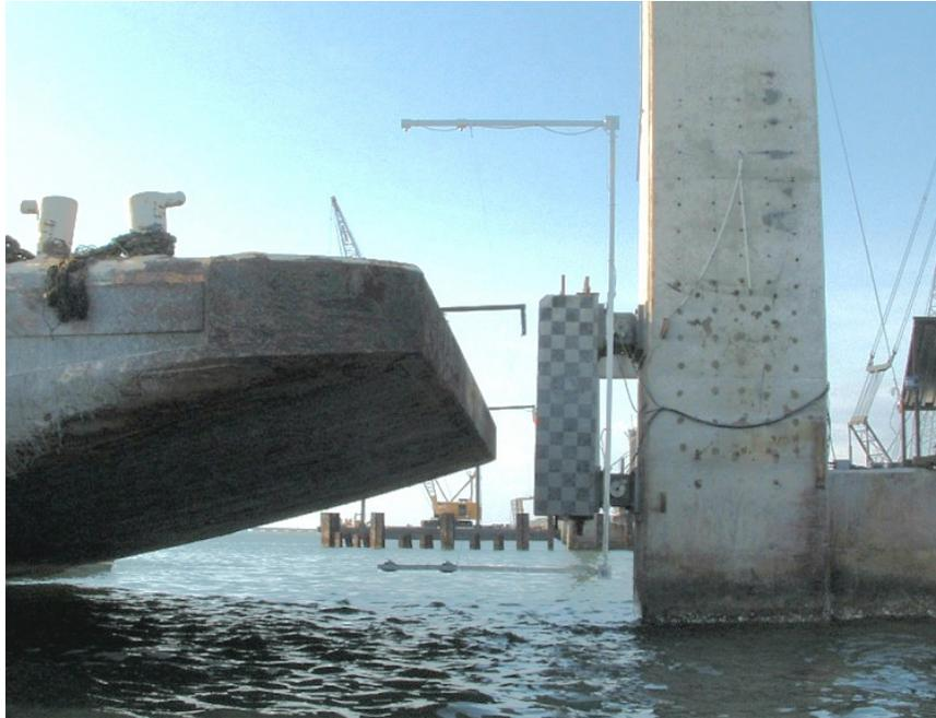
Figure 6.22 Test barge nearing contact with impact block
