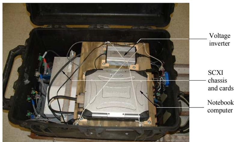
Figure 6.14 Data acquisition (DAQ) case
