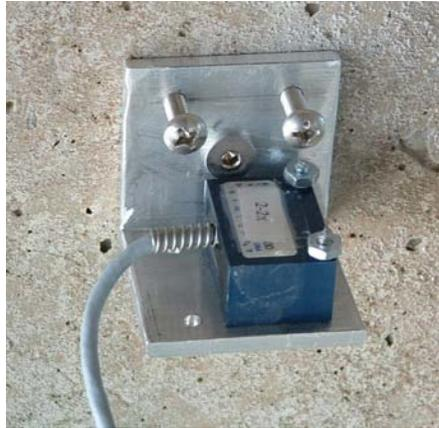
Figure 6.28 Accelerometer mounted to vertical concrete pier surface
