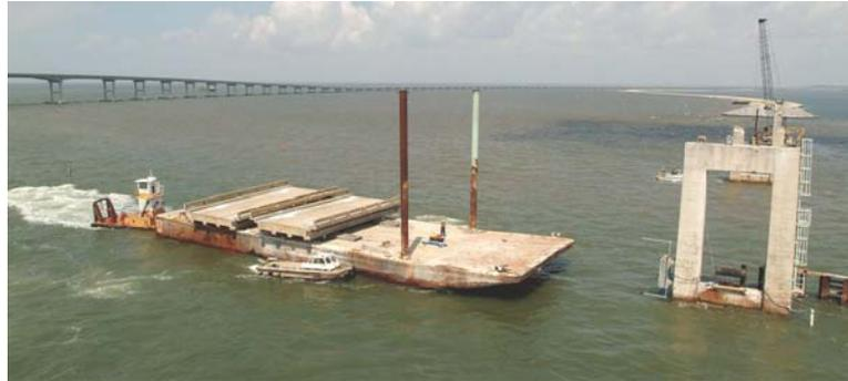
a) Test barge with payload consisting of two 55 ft. long bridge spans
