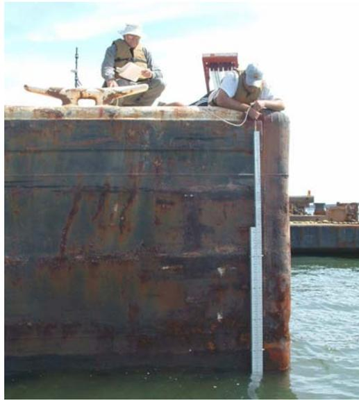
Figure 4.9 Measurement of barge draft
