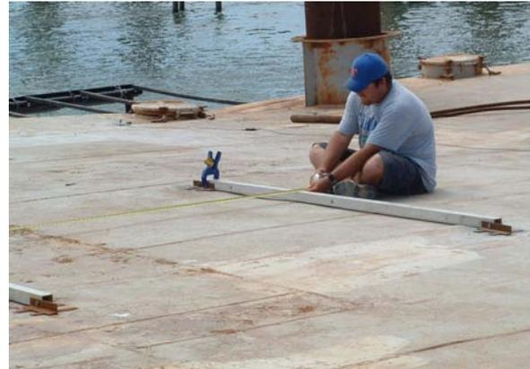
b) Recording distance measurements at datum beam
