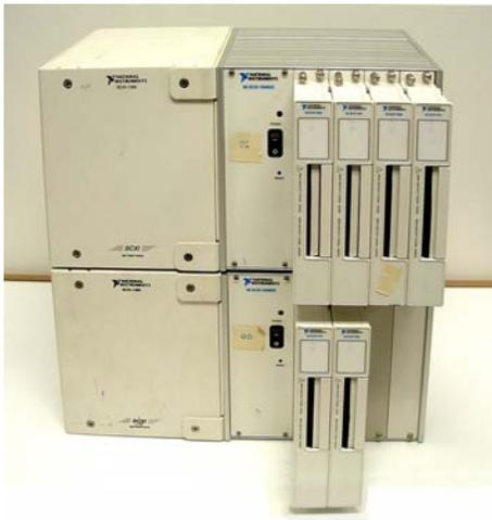
Figure 6.10 Data acquisition chassis configuration used on piers
