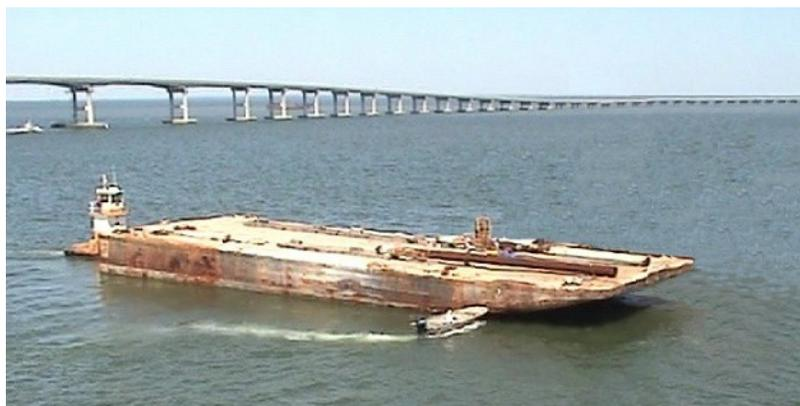
Figure 4.7 Empty-barge condition used during tests on Pier-3
