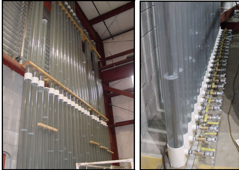
Figure 3 - Wick Bleed Test Setup. Note strand bundle inside pipe with centering device.
