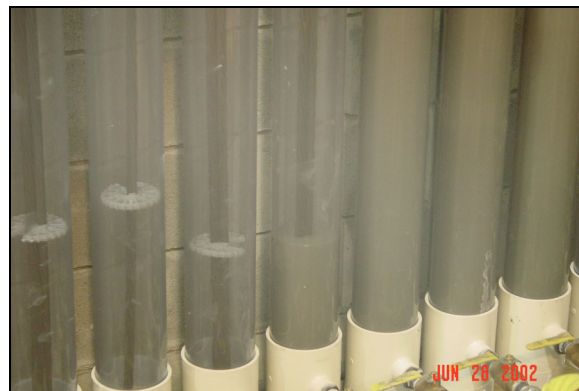
Figure 4 – Wick Induced Bleed Test Specimens During Grout Injection.
