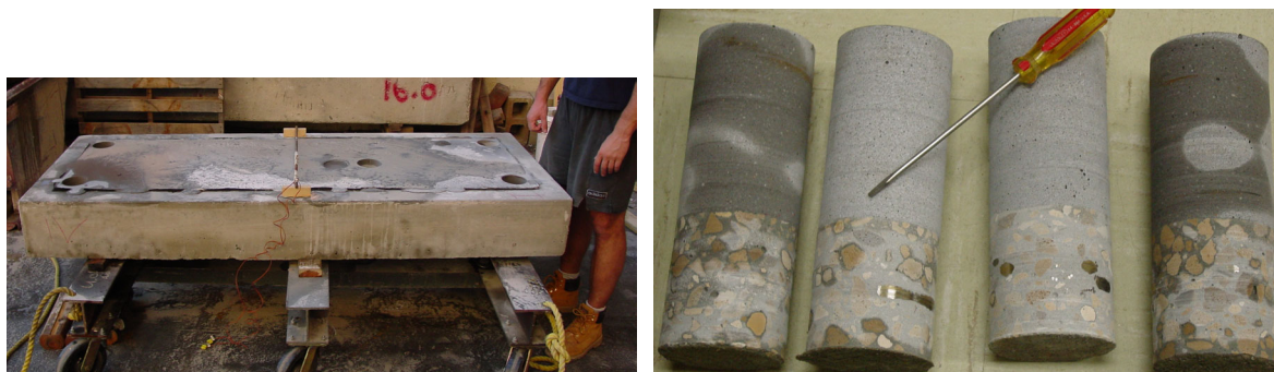
Figure 28 - Cores taken from epoxy pour-back.
