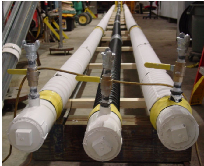
Figure 7 - Corrugated Duct Test Setup.
