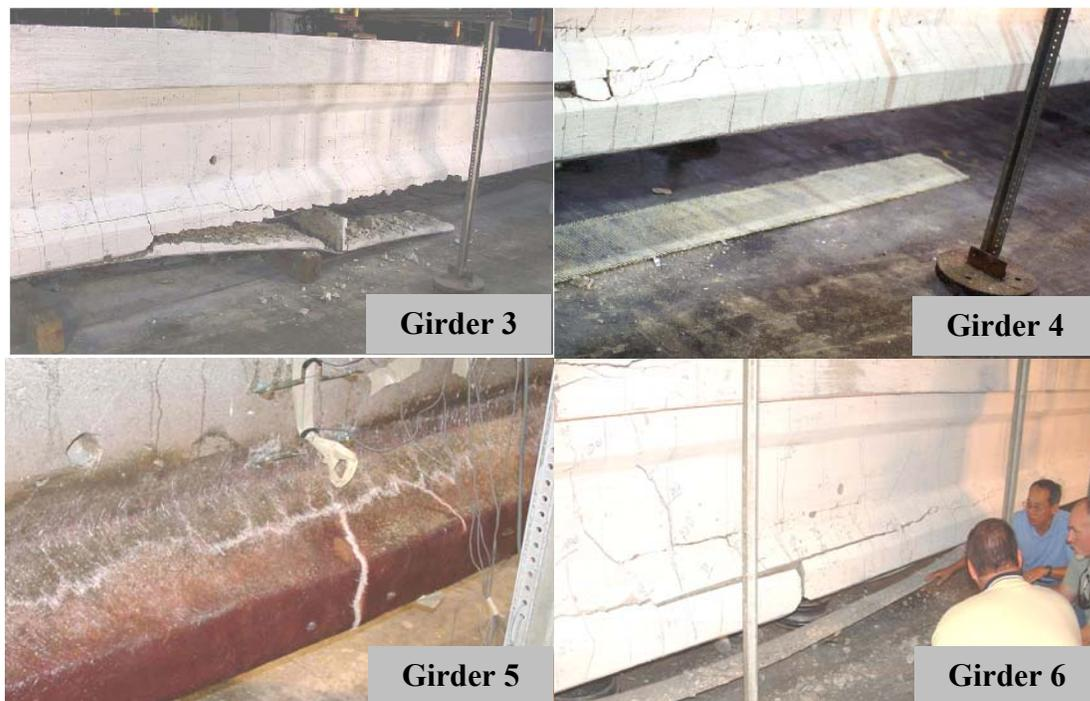
**Figure 9: Girder failure modes**
