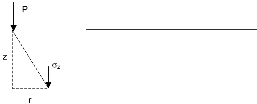
Figure 2-3. Boussinesq point load
