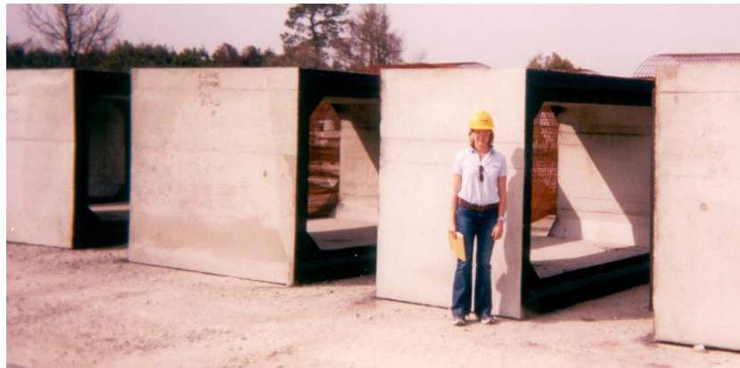
Figure 3.10: Series of 10' x 5' Precast Box Culvert Sections
