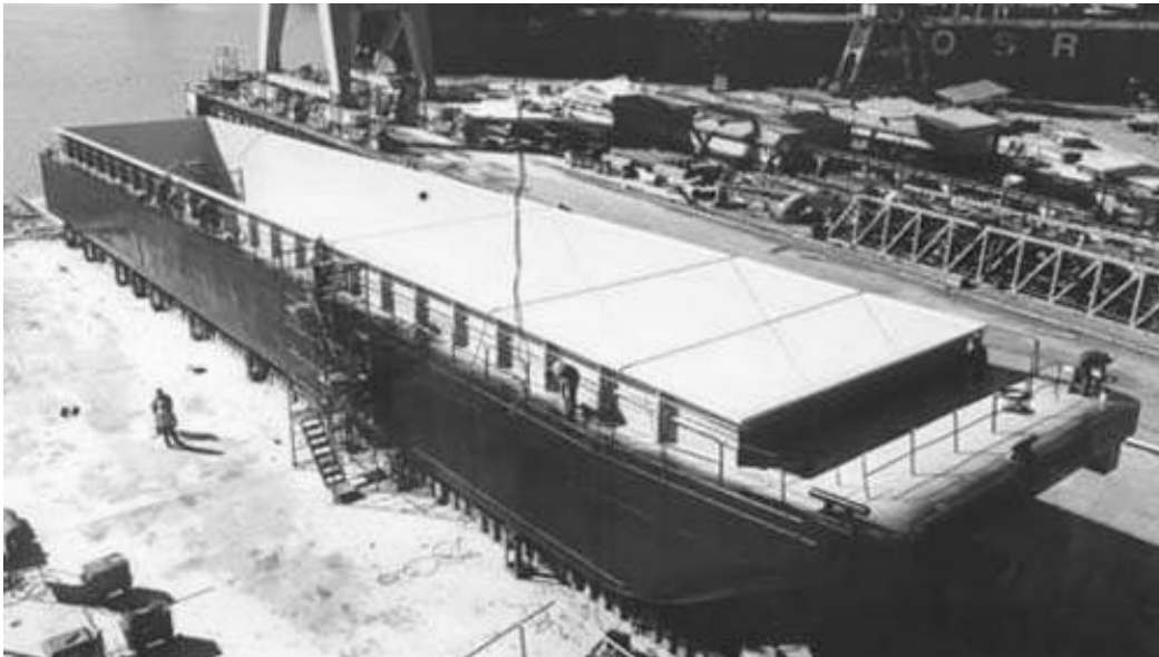
Figure 5-1 Side view of new jumbo hopper barge
