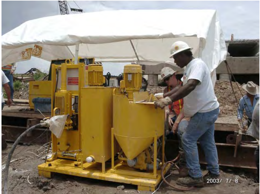
Figure 4-152 FM 507: Grout pump.
