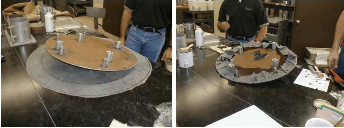
Figure 4-3 PGA Blvd: Installation of rubber membrane onto grout plate.
