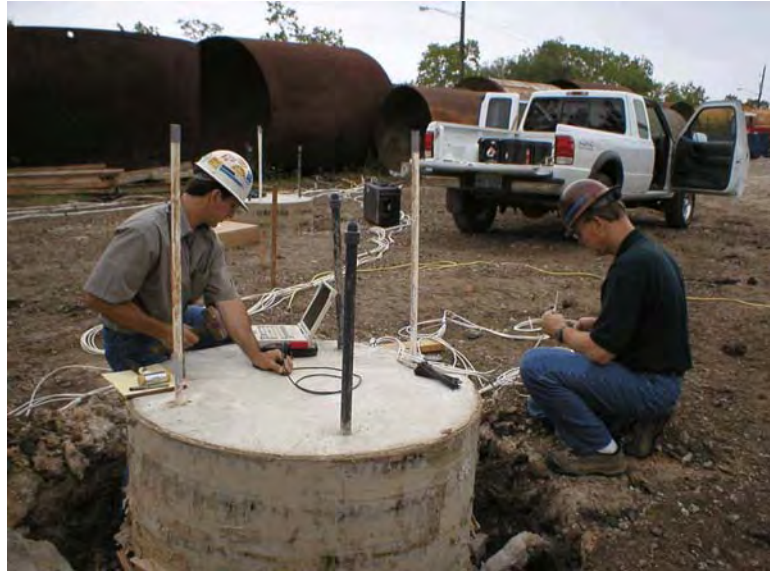
Figure 4-93 TexDOT Demo: SIT testing.
