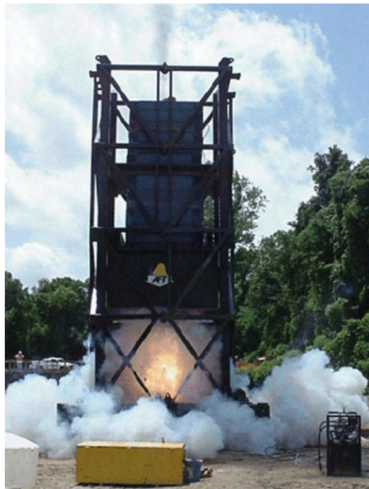
Figure 4-132 Natchez: Statnamic load testing.
