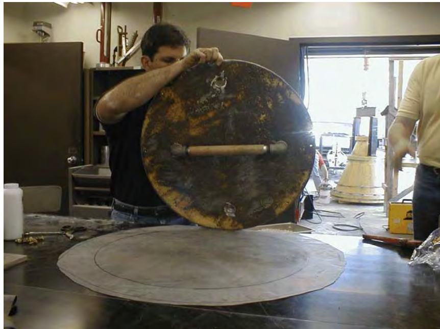
Figure 4-2 PGA Blvd: Grout plate construction with backup system.
