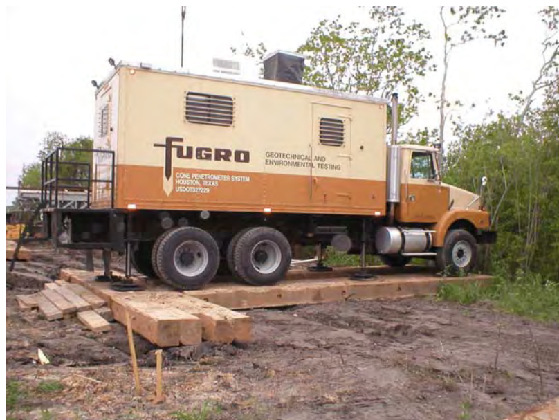
Figure 4-82 TexDOT Demo: CPT testing performed by Fugro.
