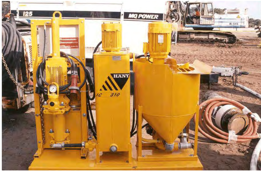
Figure 4-13 PGA Blvd: Grout pump.
