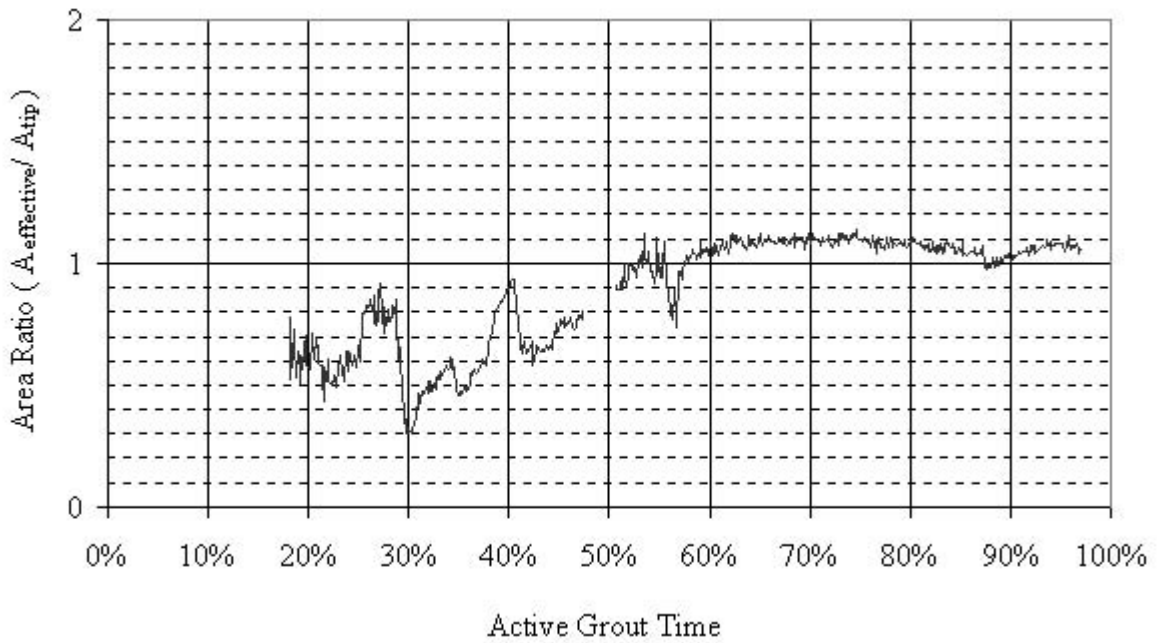
Figure B-20. Site II Flat-Jack grouting area ratio vs. active grout time.
