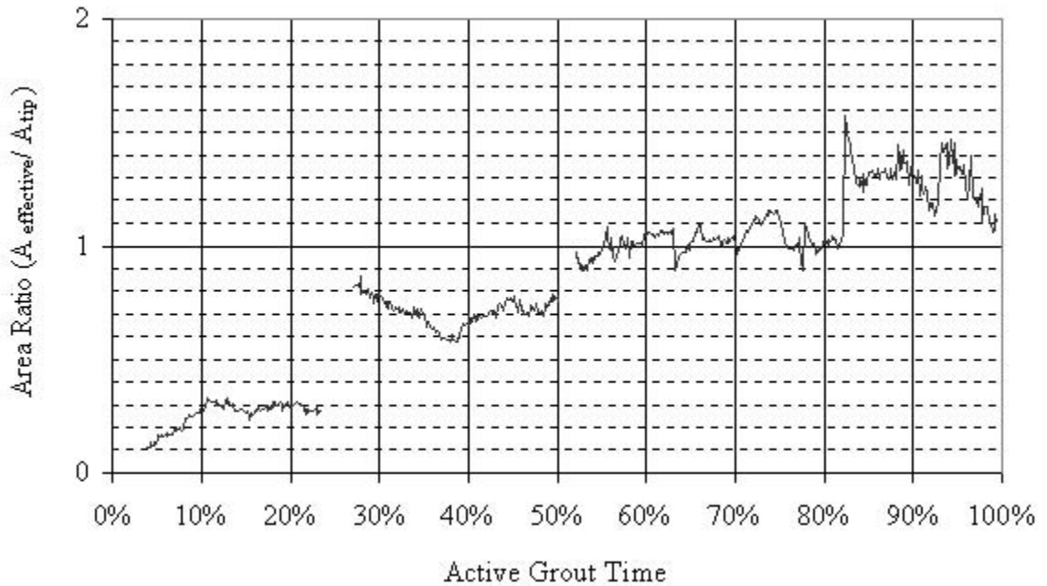
Figure B-24. Site II Sleeve-Port grouting area ratio vs. active grout time.
