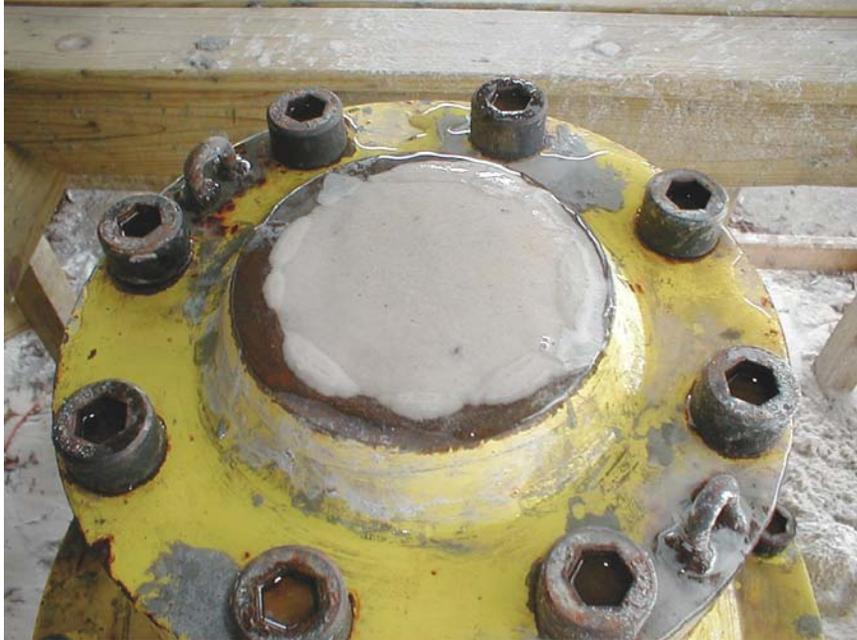
Figure 3-12 Expulsion of sand from quick pressurization.
