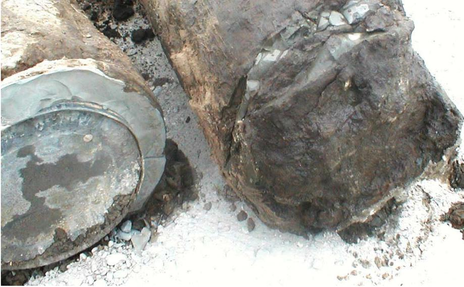
Figure 4-35. Site II exhumed flat-jack (left), sleeve-port (right) tips.
