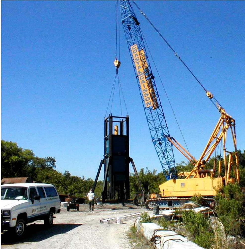
Figure 4-45. 500 ton Statnamic device being moved at Site I.
