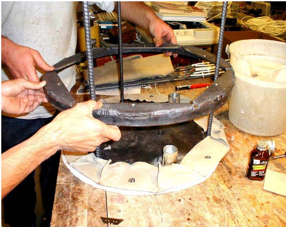
Figure 4-17. Small flat-jack during fabrication (used at Site I and Site II).
