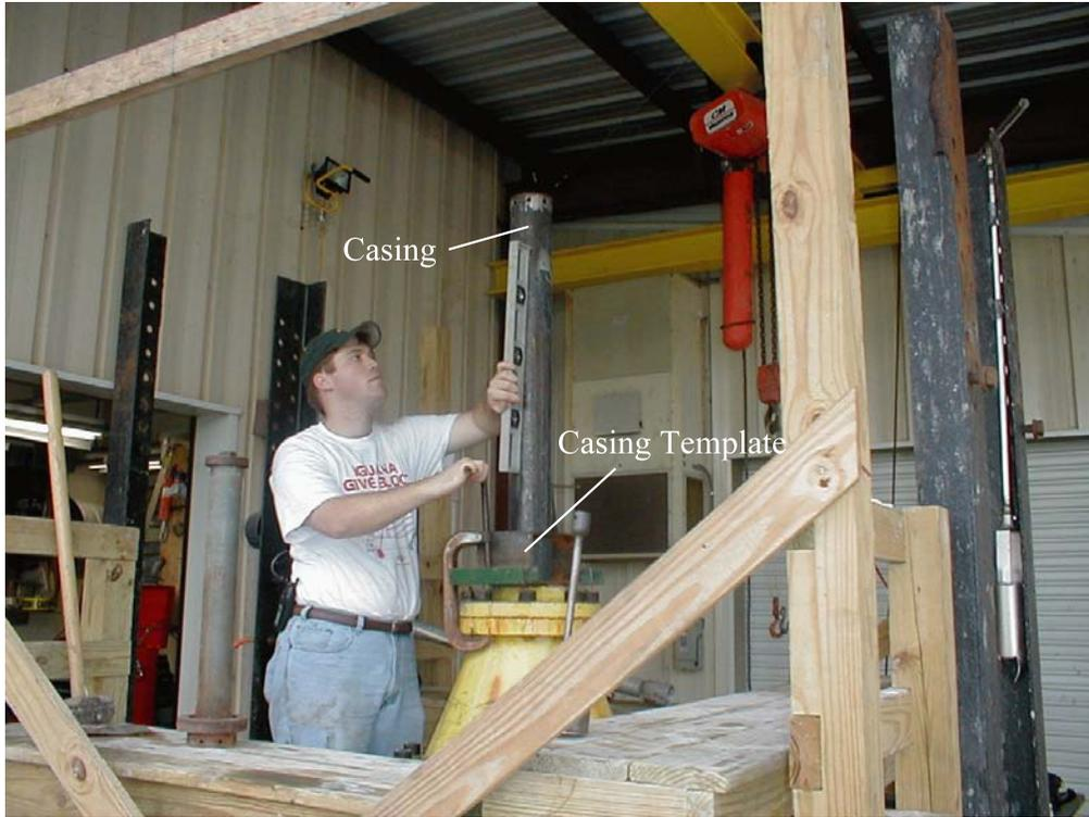
Figure 3-14 Casing driver and template.
