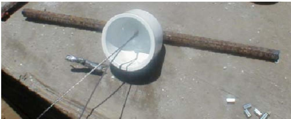
Figure 4-26. Site III tension telltale fabrication.
