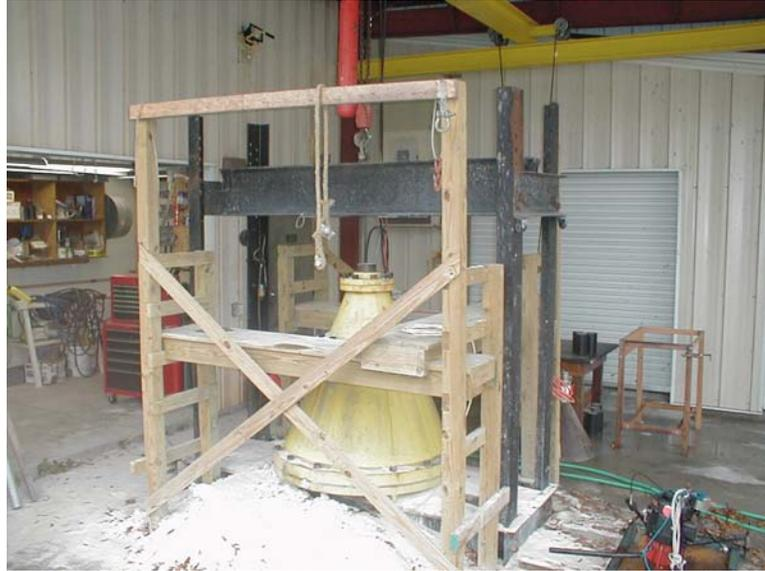
Figure 3-5 Load testing frame and scaffolding.
