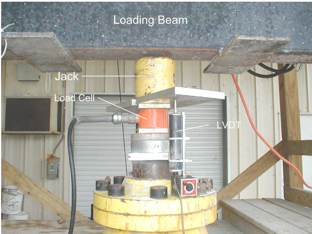
Figure 3-22 Load testing apparatus.
