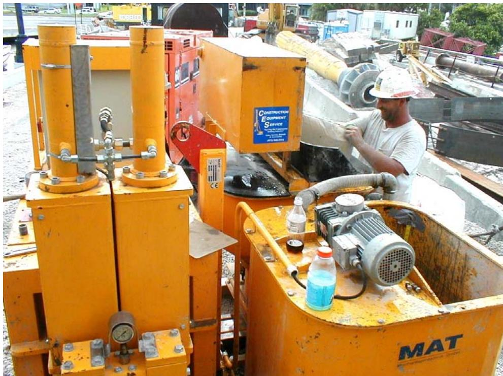
Figure 4-46. Dual-piston (ram-style) grout pump used on Site III.
