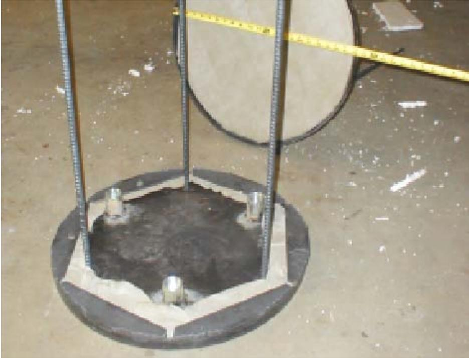
Figure 4-18. Small flat-jack completed (used in Sites I and II).
