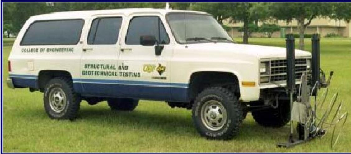
Figure 4-5. University of South Florida's mini-cone penetrometer (MCPT).
