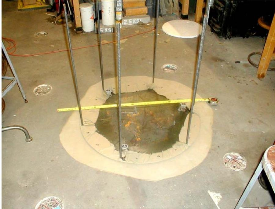
Figure 4-16. Large flat-jack during fabrication (used at Site III).
