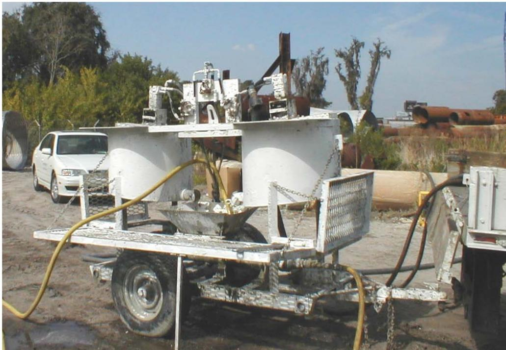
Figure 4-44. Helical-style grout pump used for Sites I and II.
