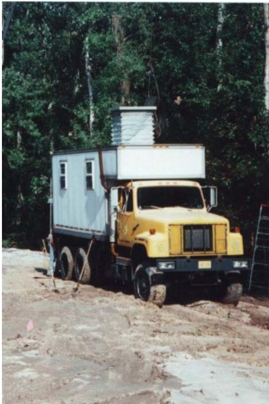
Figure 4-6. FDOT Dist.1 cone penetrometer.
