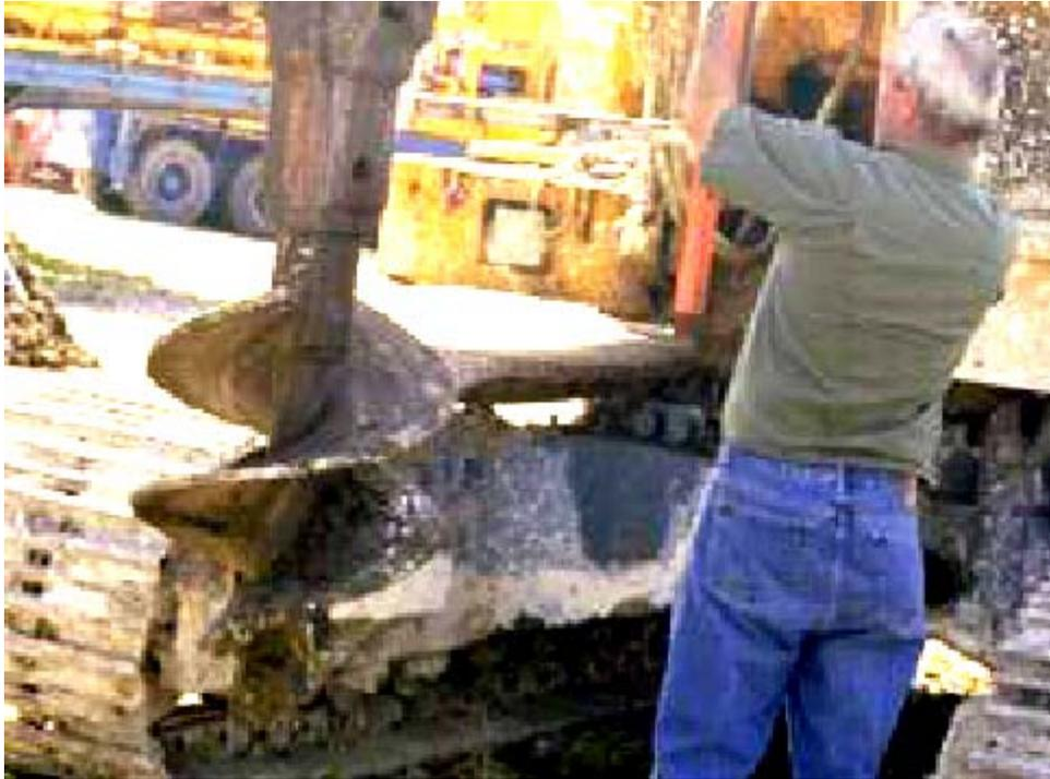
Figure 4-32. Auger used to excavate Sites I and II.
