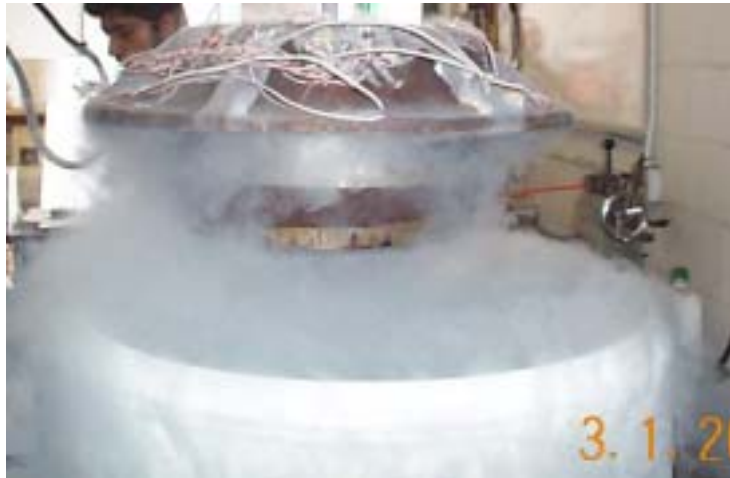
Figure 7.18 Cooled hub pulled out of the dewar.
