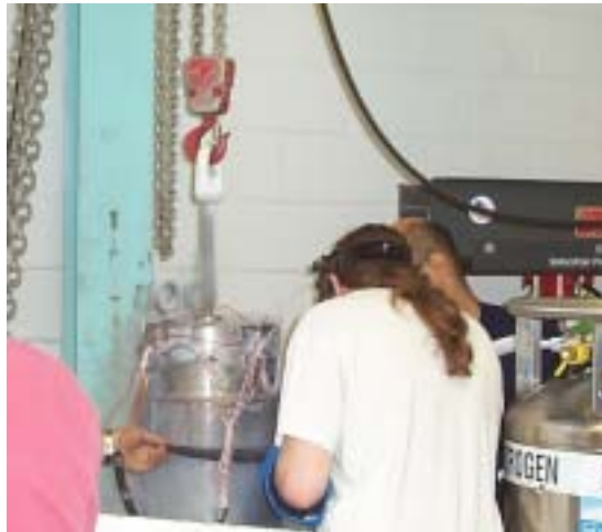
Figure 7.7 Measurement of shrunk diameter of cold trunnion with a micrometer.
