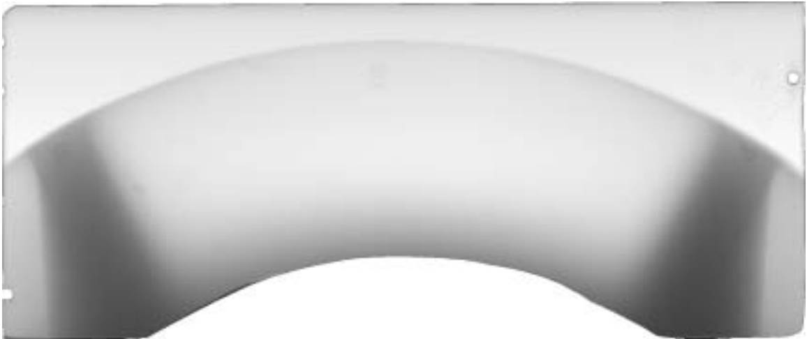
Figure D.2e X-ray of the hub from the web view (4-5).
