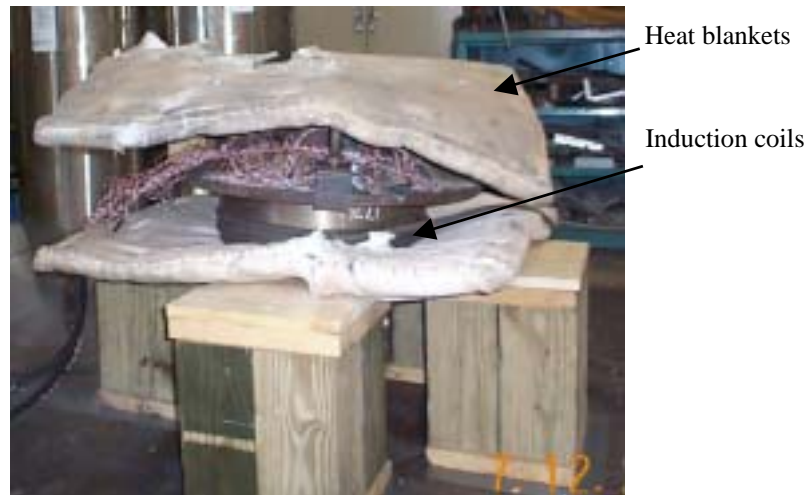
Figure 7.5 Hub heated with induction coils.
