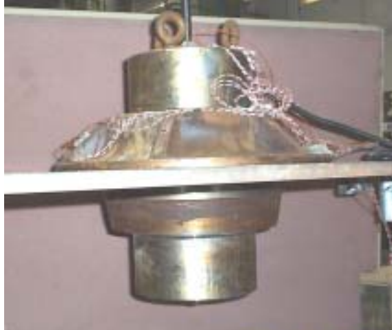
Figure 7.28 THG assembly lifted by the overhead crane.
