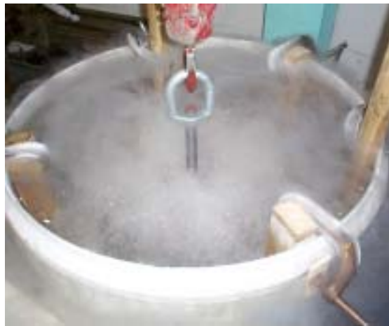
Figure 7.23 Trunnion cooled in the liquid nitrogen dewar.
