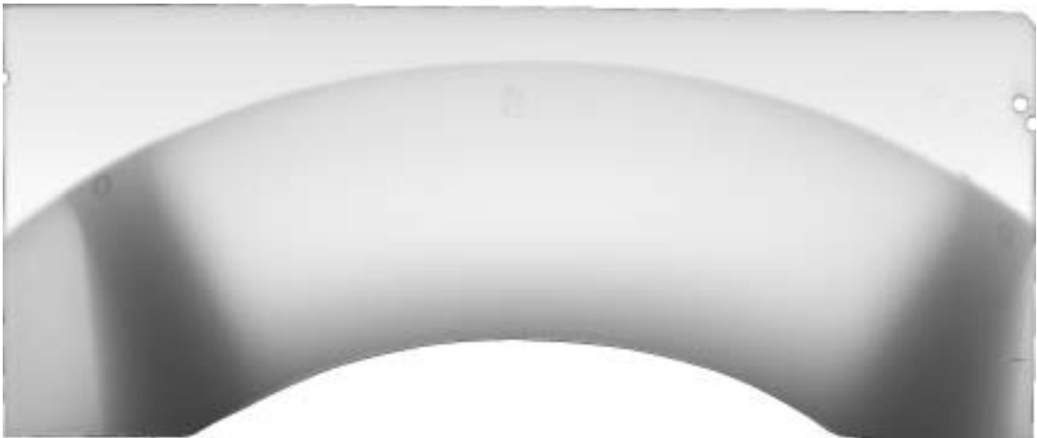
Figure D.2f X-ray of the hub from the web view (5-0).
