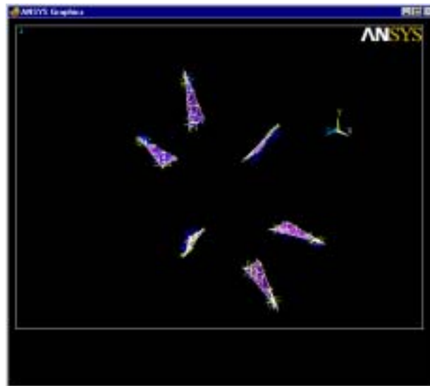
Figure 3.2b Thermal element SHELL57 and structural element SHELL63.
