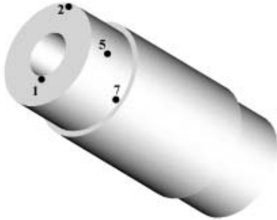
Figure 7.15 Positions of the gages on the trunnion.
