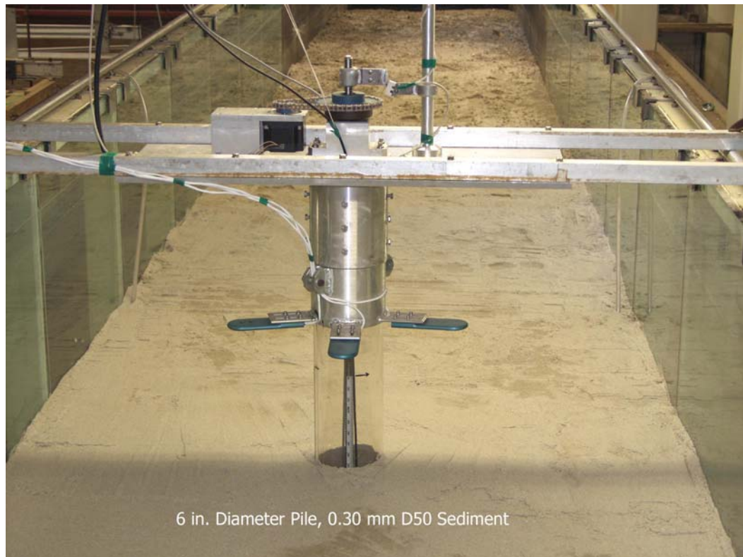
Figure 7. Photograph of the internal video cameras traversing mechanism and the acoustic transponders used to measure scour depth.
