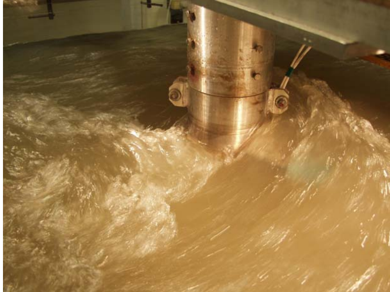
Figure 13. Flow around test pile during a live bed test viewed from down stream.
