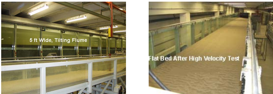
Figure 2. Side and top views of the 5 ft wide, 4 ft deep, 148 ft long flume used for the local scour tests
