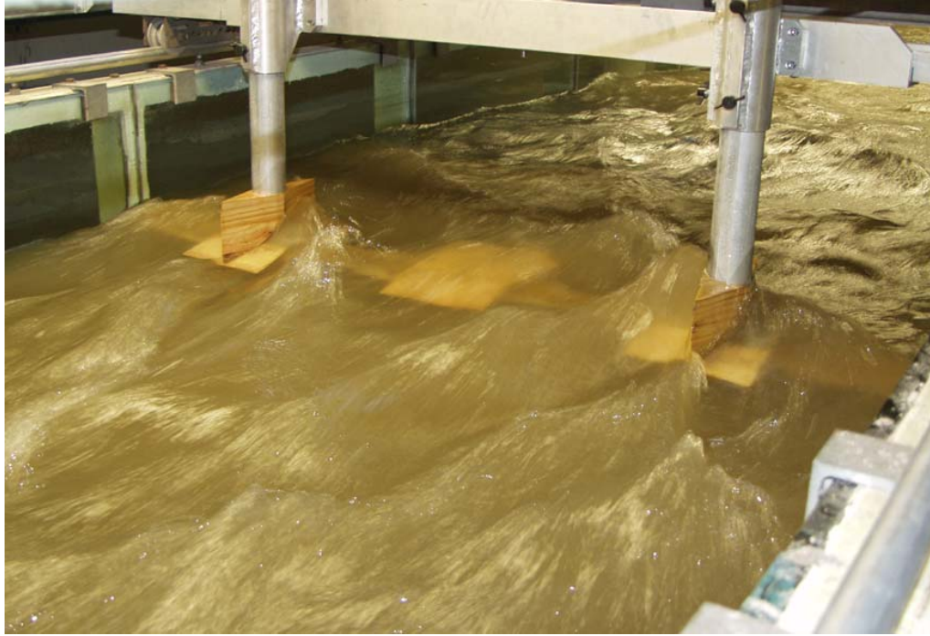
Figure 11. Bed form transducers with drag reducing hydrofoils during a live bed test.
