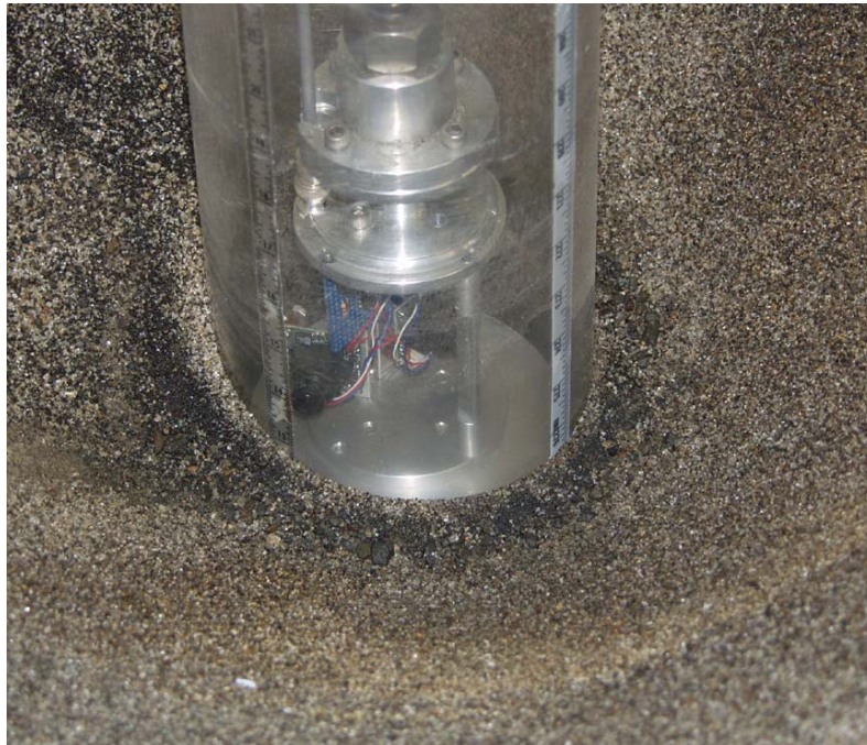
Figure 8. Internal video cameras and housing for the 6 in. diameter test cylinder.
