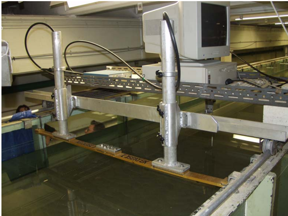
Figure 10. Array of acoustic transducers used to measure bed forms (prior to installing drag reduction hydrofoils).
