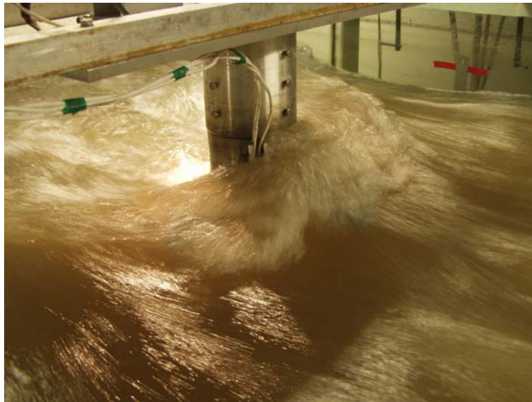
Figure 12. Flow around test pile during a live bed test viewed from upstream.
