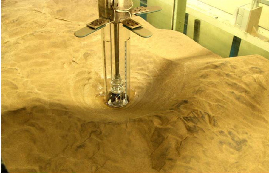
Figure 15. Scour hole after live bed scour test with large bedforms.
