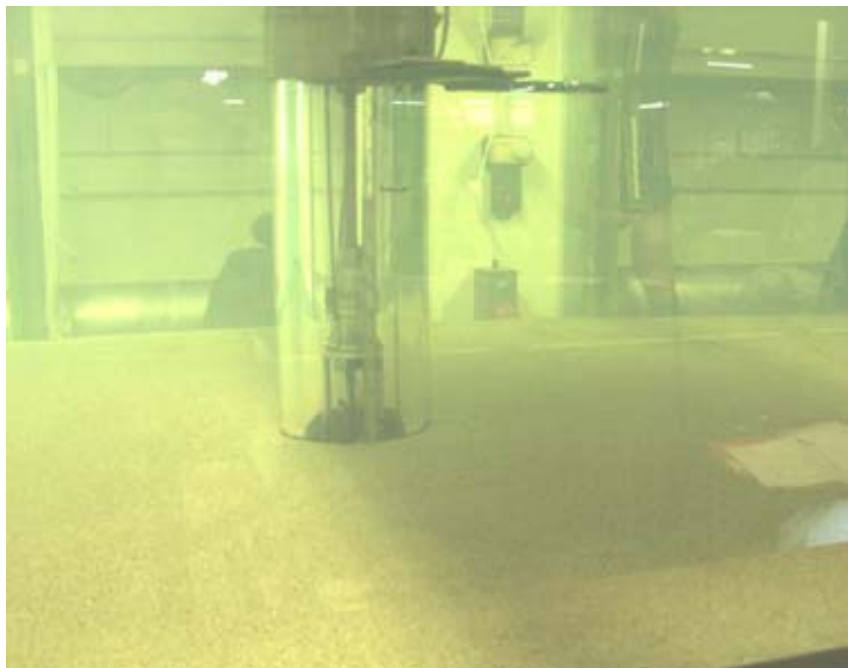
Figure 14. Photograph of test pile prior to live bed scour test taken through the water from outside the flume.
