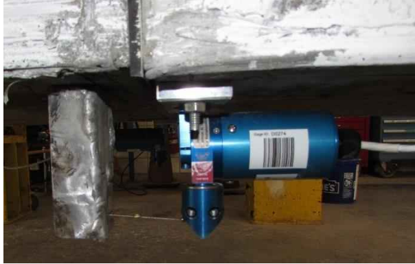
Figure 5-20 Gap displacement gages attached to specimen
