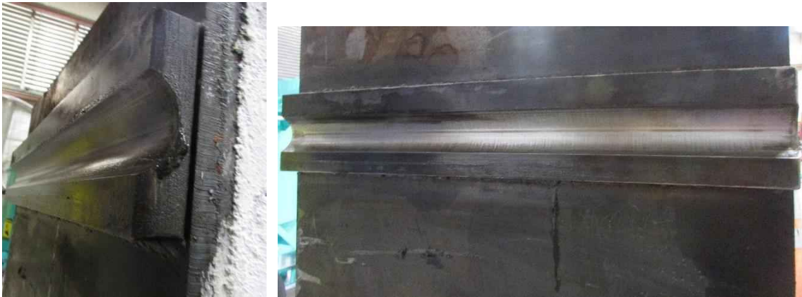
Figure 13-15 Mechanical hinge post-dissection – dead end segment
