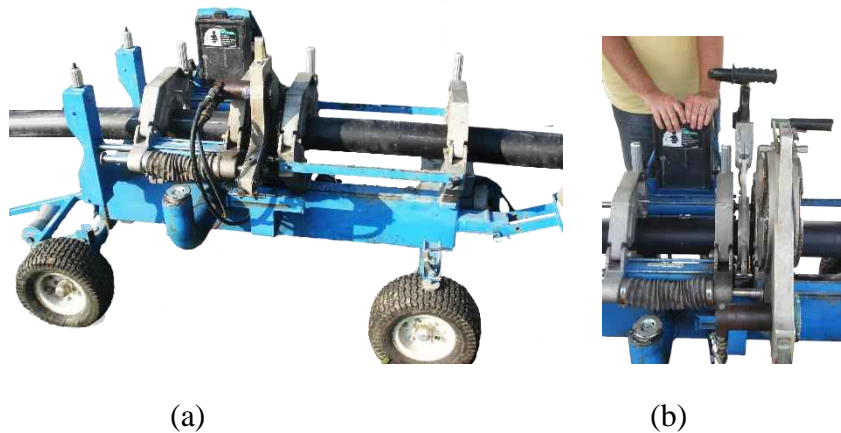
Figure 5-9 (a) McElroy HDPE fusion machine; (b) Duct fusion in progress
