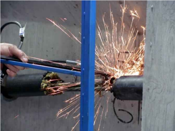
(b) wire cuts with Dremel tool
