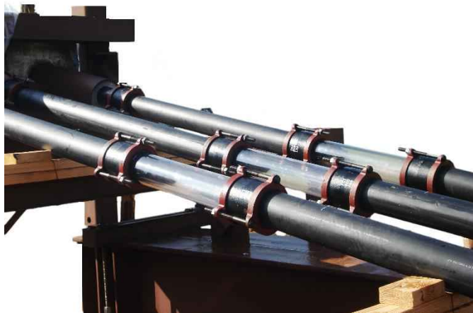
Figure 5-12 Clear windows in duct
