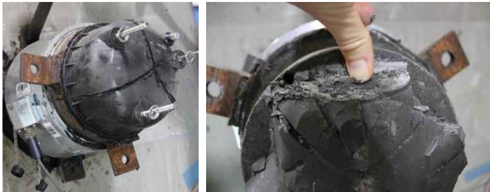
Figure 6-11 IGS Outlet (dead end) prior to and after cap removal
