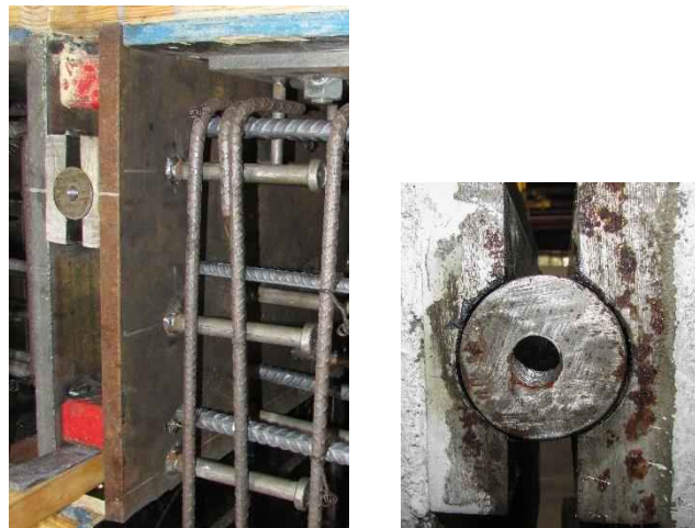
Figure 4-18 Mechanical hinge details
