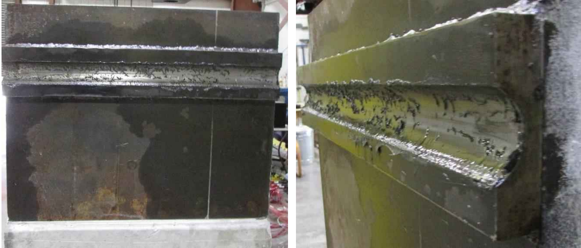
Figure 13-16 Mechanical hinge post-dissection – live end segment
