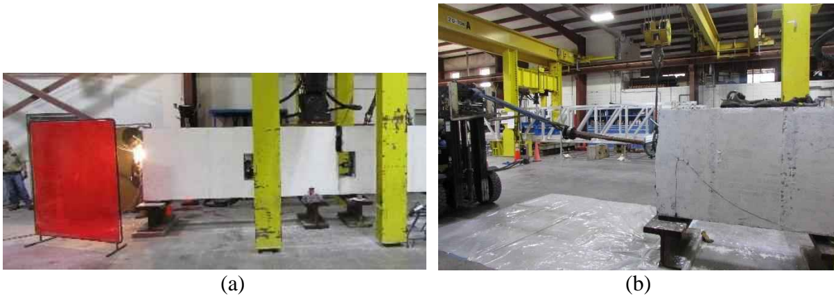
Figure 13-13 Dissection of F1 (a) detensioning and (b) tendon removal
