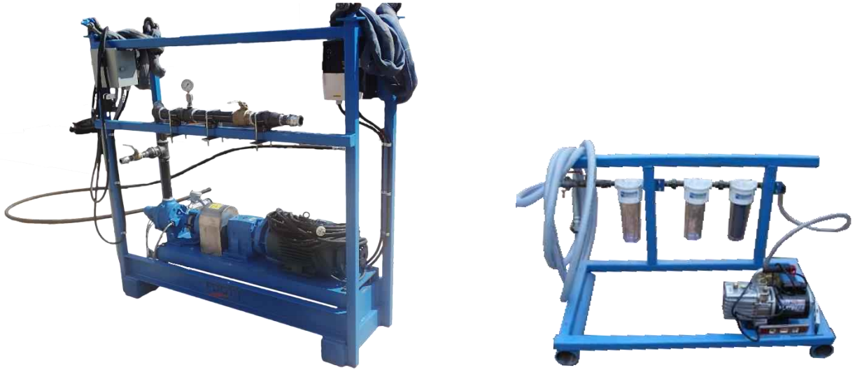
Figure 5-3 Viking pump used for filler injection (left) and vacuum pump and reservoirs (right)
