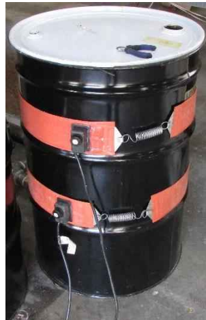
Figure 6-40 Heating barrel containing flexible filler for injection
