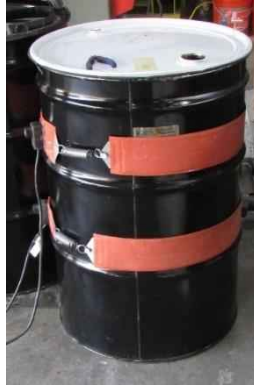
Figure 6-14 Heating flexible filler for injection
