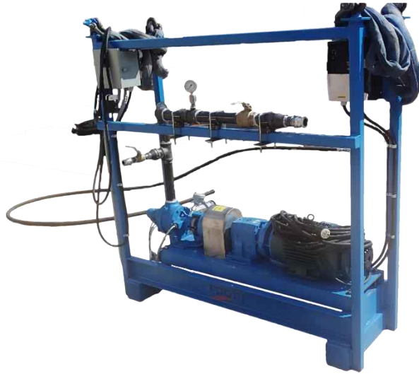
Figure 5-22 Viking pump used for filler injection
