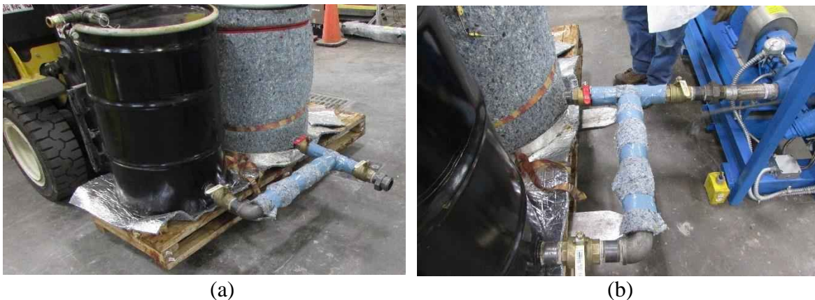
Figure 6-44 Positioning of filler barrels (a) transporting filler barrel and (b) centrifugal pump connection
