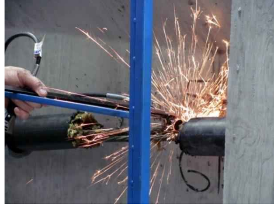
(b) wire cuts with Dremel tool
