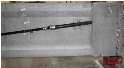
Figure 4-11 Duct exiting end block of external specimen
