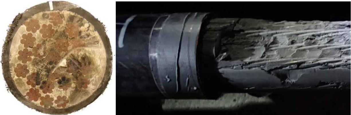
Figure 2-4 External tendons with cementitious grout
