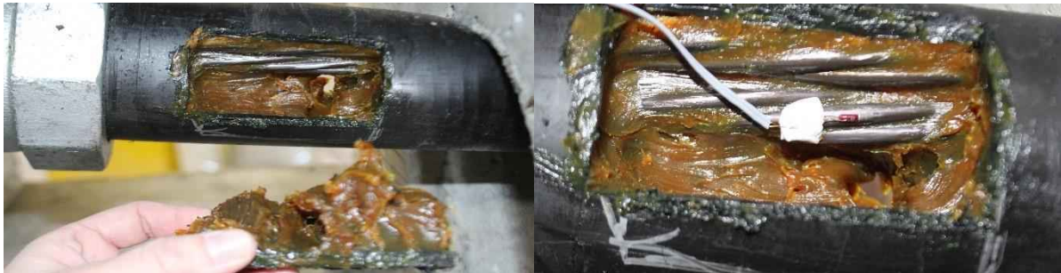
Figure 5-18 Removal of HDPE section to attach strain gage
