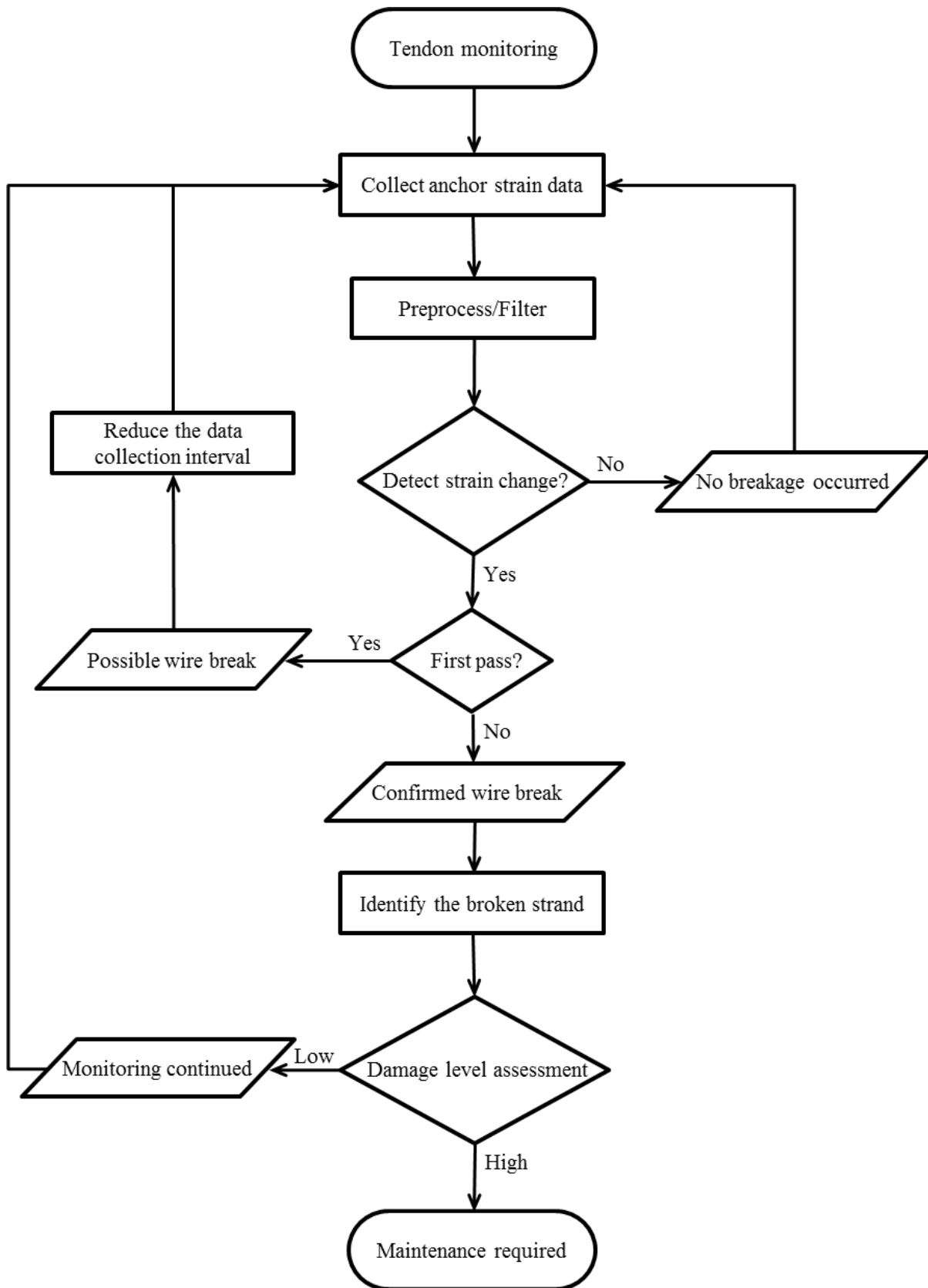
Figure 7-6 Wire breakage identification flowchart
