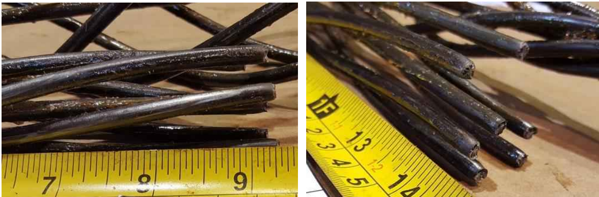
Figure 13-29 Specimen F1 strand ductile failures after tensile tests
