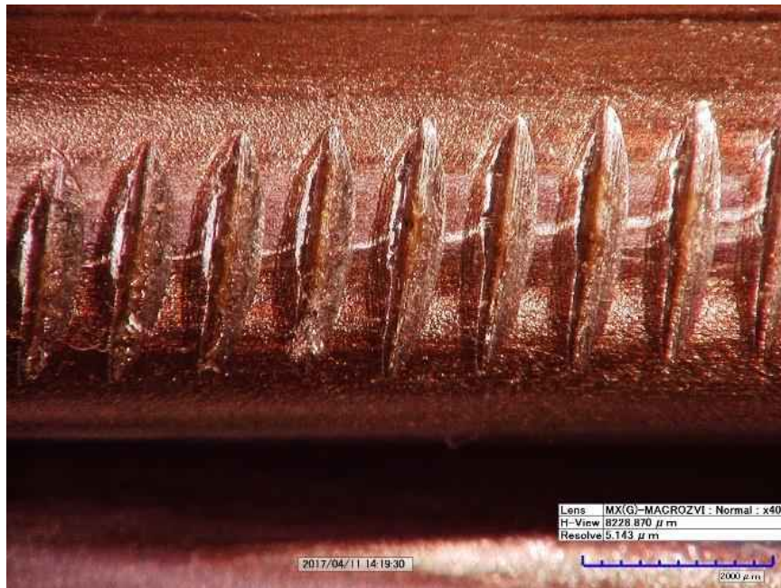
Figure 13-21 Wedge serration impressions on strands following cyclic loading
