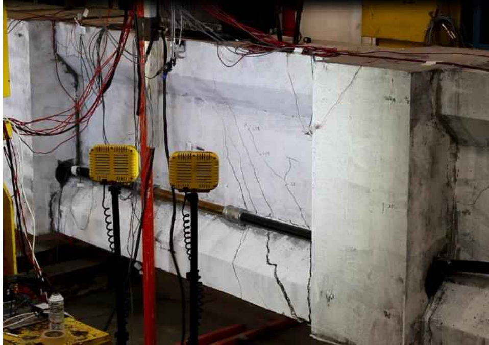
Figure 11-11 EWC near ultimate load
