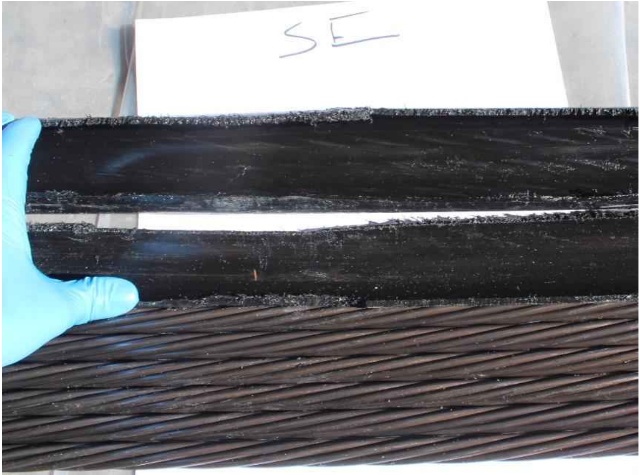
Figure 11-24 EWC: dissection of tendon at SE diablo
