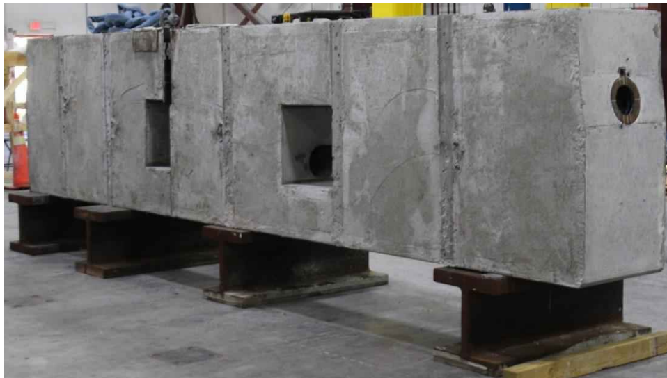
Figure 6-29 Completed fatigue specimen without post-tensioning
