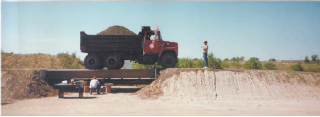
Figure 13. Load testing of No-Name Creek bridge after installation in November 1996.
