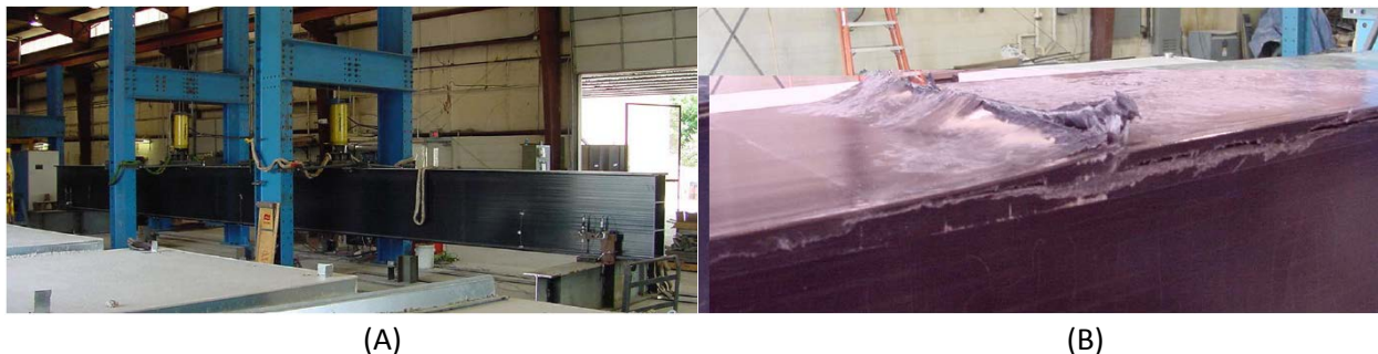
Figure 23. Four-point bending test of 36x18 EXTREN DWB (Note 48, pg. 27). (A) Laboratory setup and (B) failure in compression flange at loading point.
