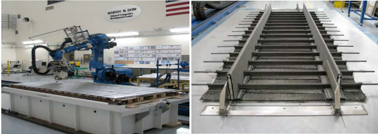
Figure 39. Robot arm performing through-the-thickness stitching [100].
