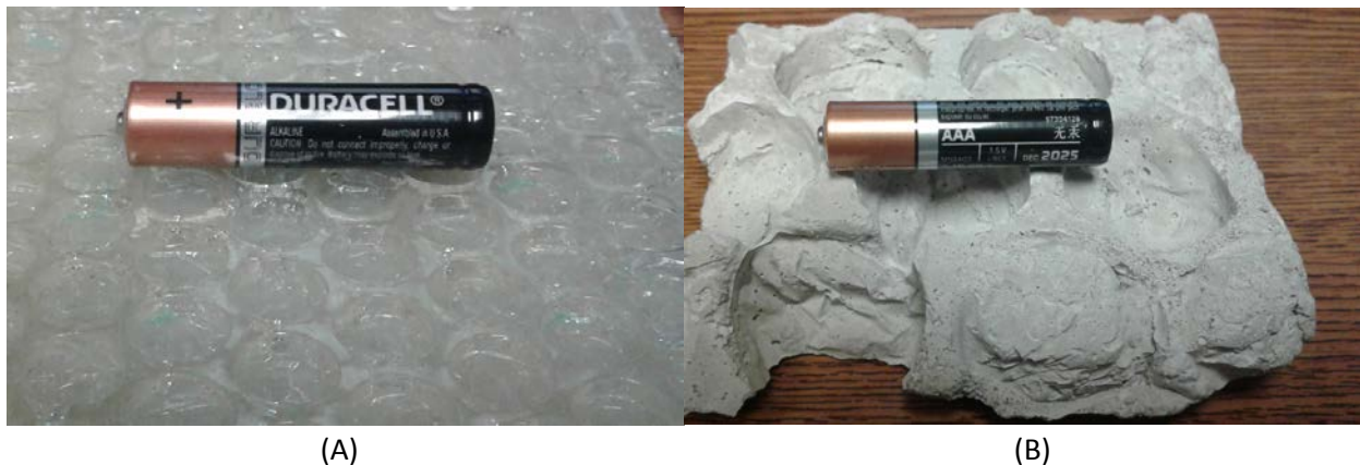
Figure 111. Textured surface to enhance mechanical bond between FRP and concrete. (A) GFRP laminate and (B) levelling grout. AA battery included for size reference.
