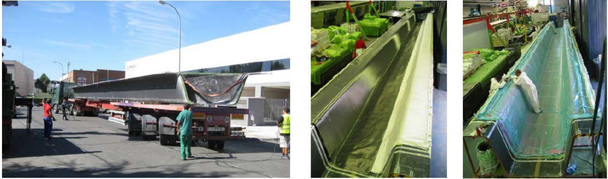
Figure 36. Glass FRP pedestrian bridge girder manufactured in 2010 using the VIP/VARTM method. Photos from 2012 CICE conference paper by Paulotto et al. [26].
