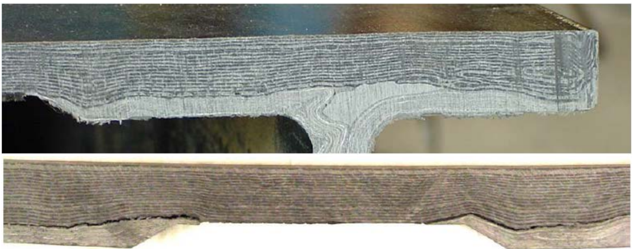
Figure 107. Delamination between quasi-isotropic glass and carbon/CSM laminates during laboratory beam test of 36x18 EXTREN DWB. Section was taken away from rupture zone at midspan.
