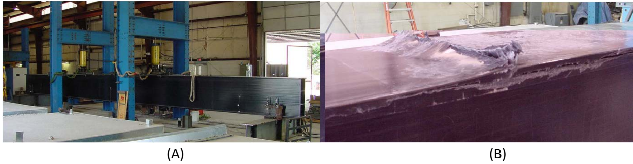
Figure 106. Four-point bending test of DWB 36. (A) Laboratory setup and (B) failure in compression flange at loading point.
