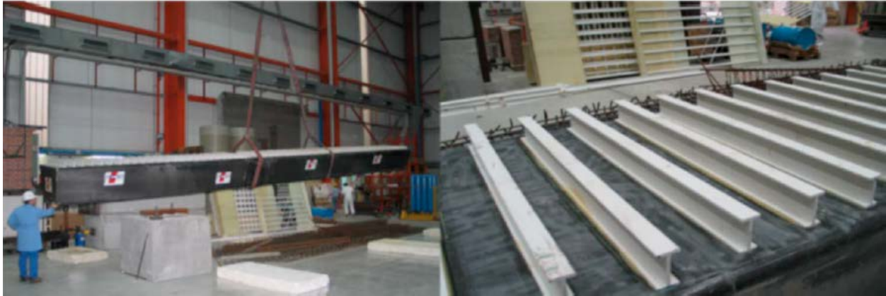
Figure 34. Full scale carbon FRP bridge girder test (European demonstration project). Photo from ASCE Journal of Bridge Engineering paper by Gutierrez et al. [25].
