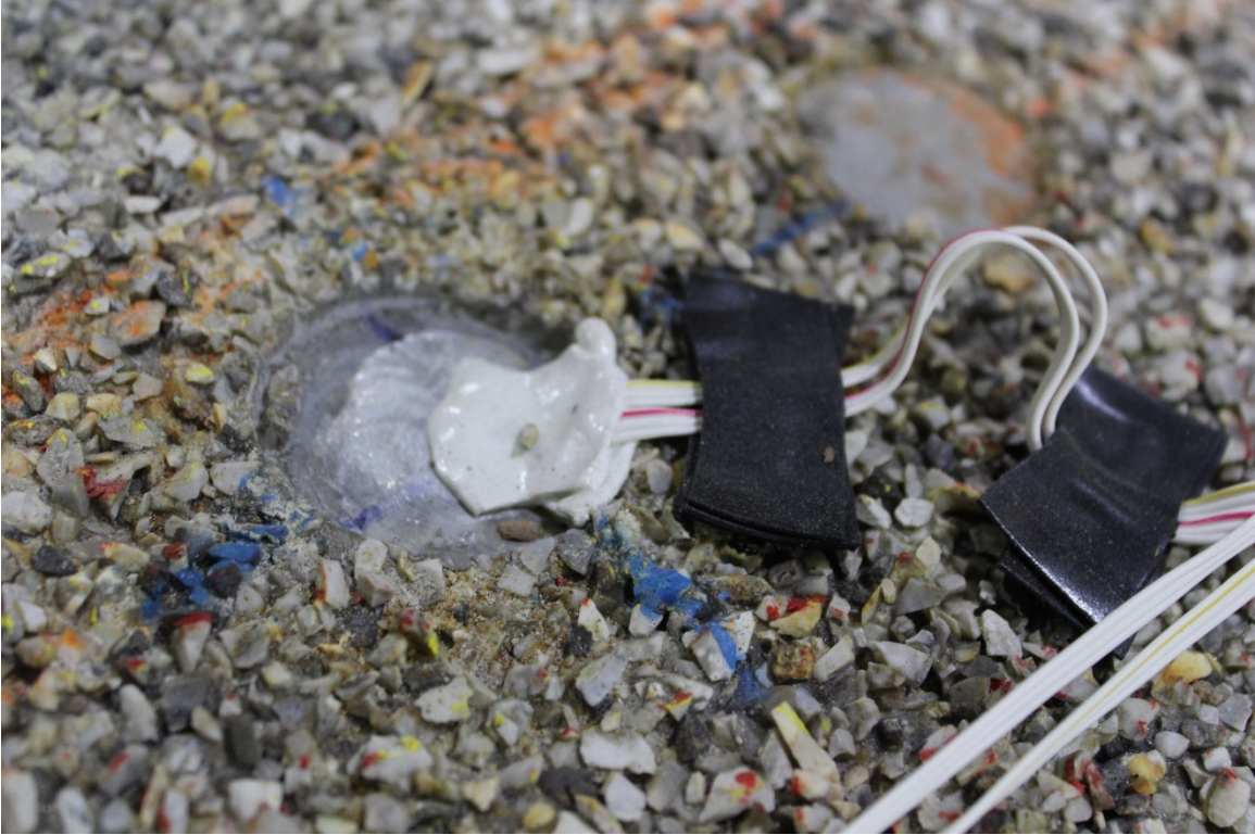
Figure 18: Installed Strain Gage
