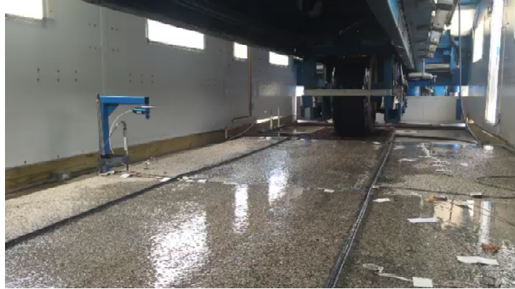
Figure 40: Heavy Vehicle Simulator Water Saturated Test
