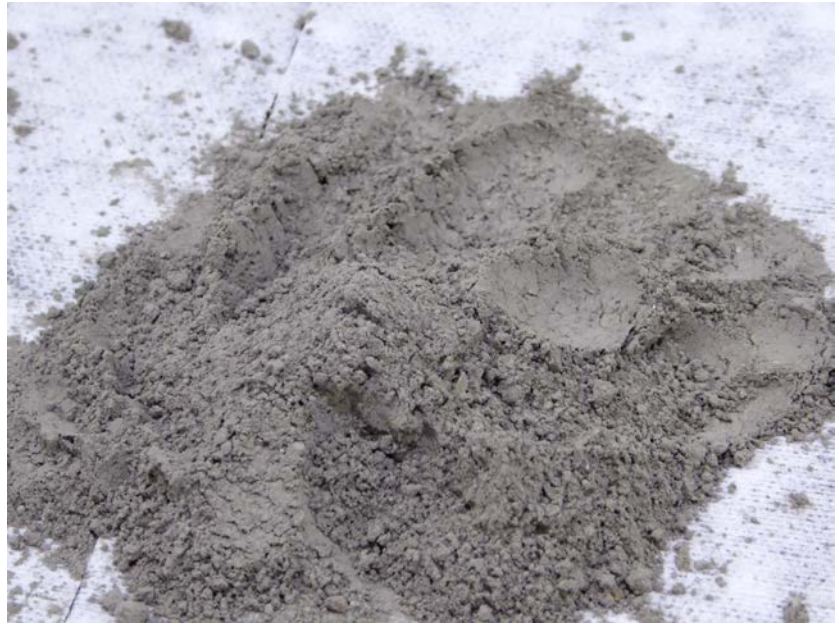
(b) Loose grout powder
