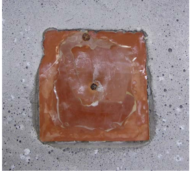
(b) Shim in specimen MU9 — 1.0 in. (25 mm) Taper
