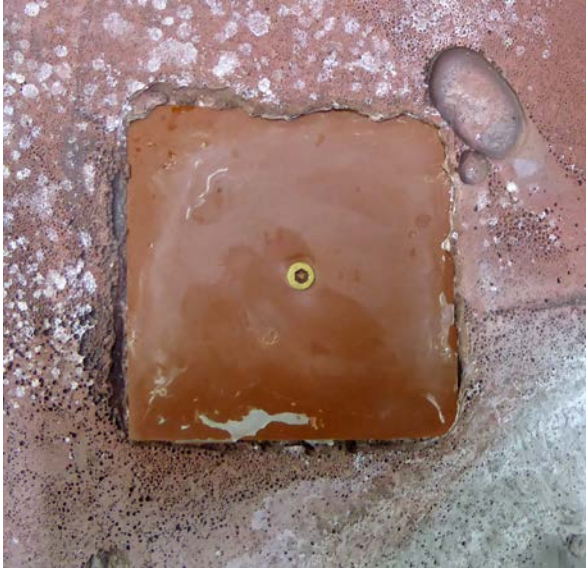
(a) Shim in specimen MU8 — 0.5 in. (12.5 mm) Taper
