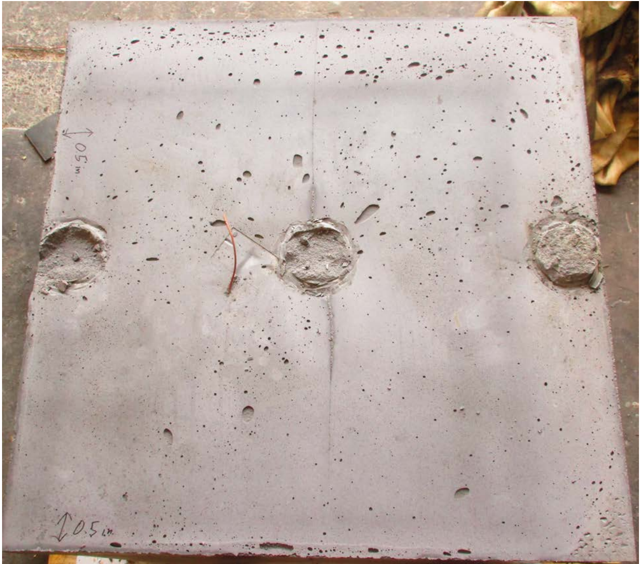
Figure 4.15: Top surface MU6 — representative for specimens with higher water-to-material ratio
