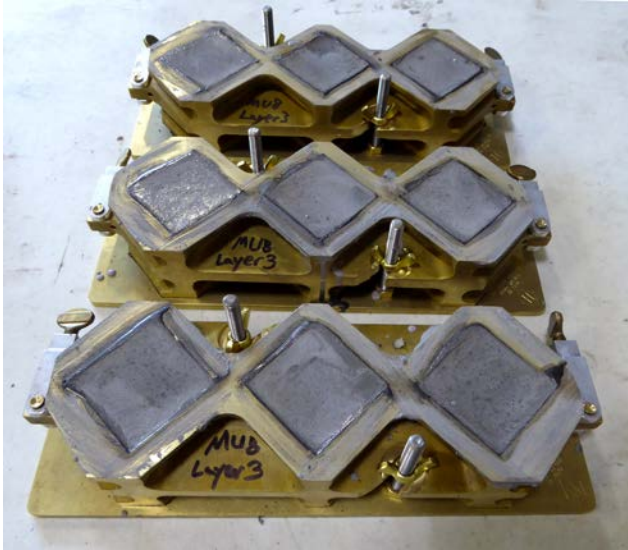
(a) Fresh grout in cube molds
