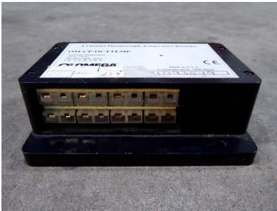
(c) Thermocouple box
