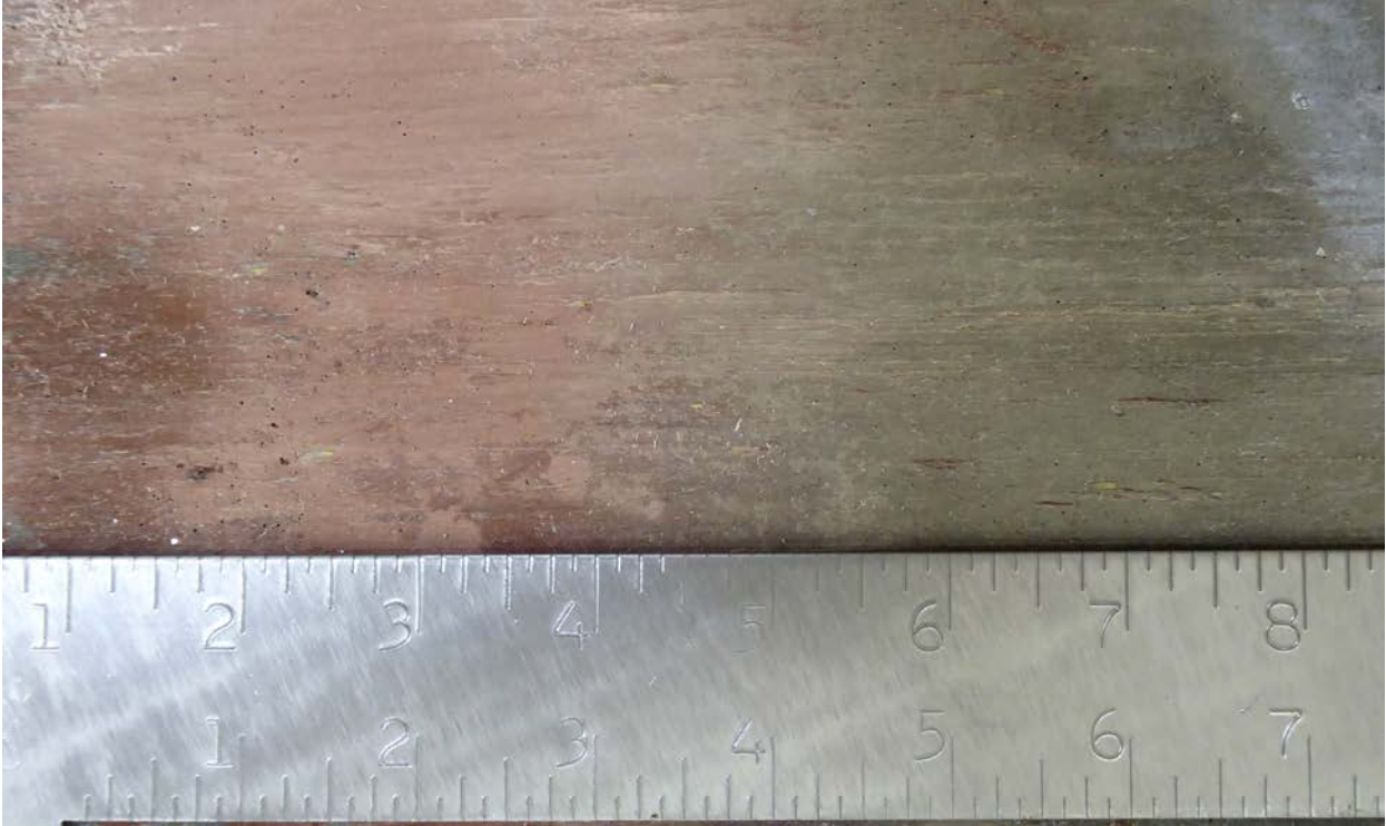
Figure 4.18: Inner top surface for MU11 — maximum grout volume thickness of 1.0 in. (50 mm)
