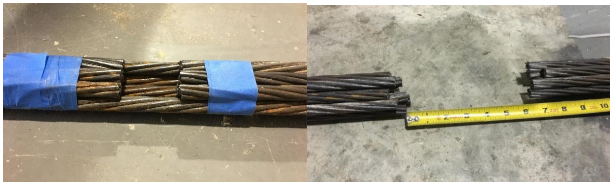
Figure 5-32: Complete and partial physical discontinuity.
