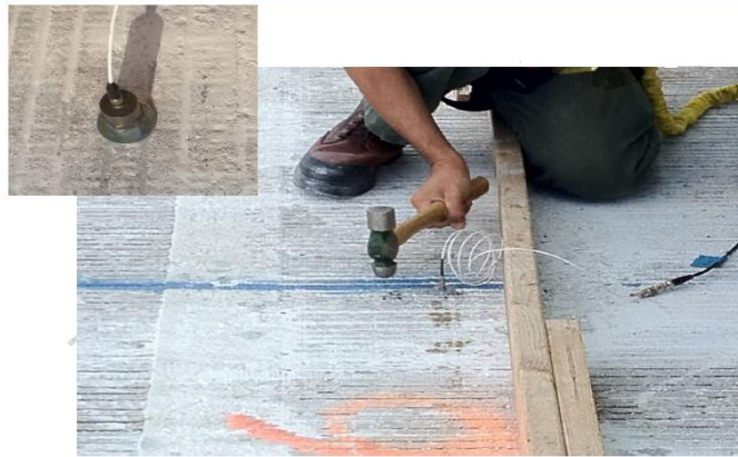
Figure 4-22: Trial source location testing using a metal ball peen hammer.
