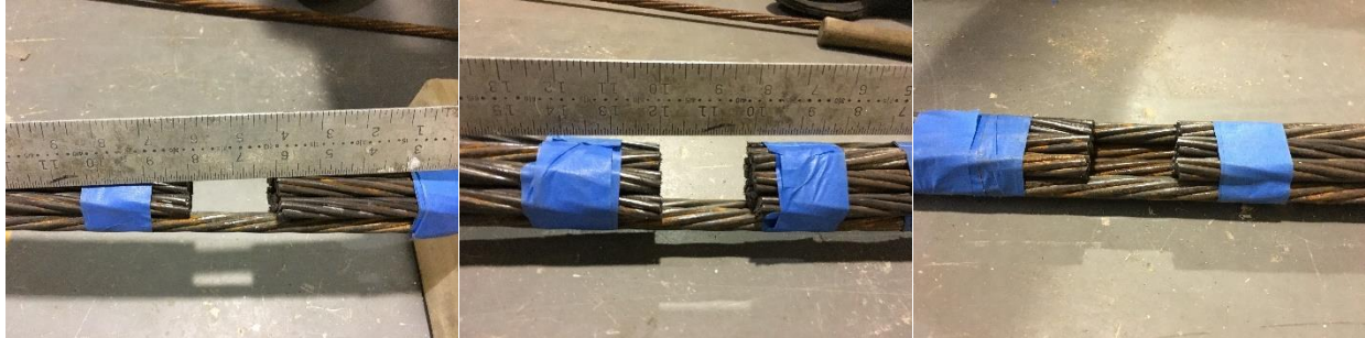
Figure 5-46: Different strand defect percentage 90% (left) 80% (center) and 50% (right).
