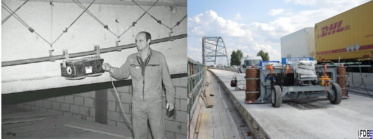
Figure 5-50: Electromagnet application to MFL systems: application of electromagnet for vertical members (left) and surface scanners (right) (photo courtesy Dr. Hillemeier).
