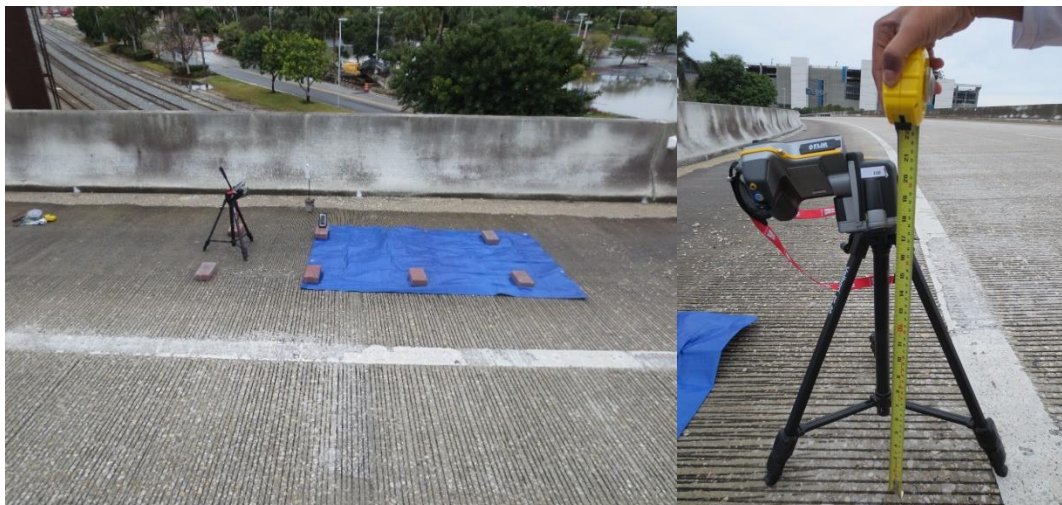
Figure 4-10: Surface infrared testing site (left) and thermal camera setup (right).
