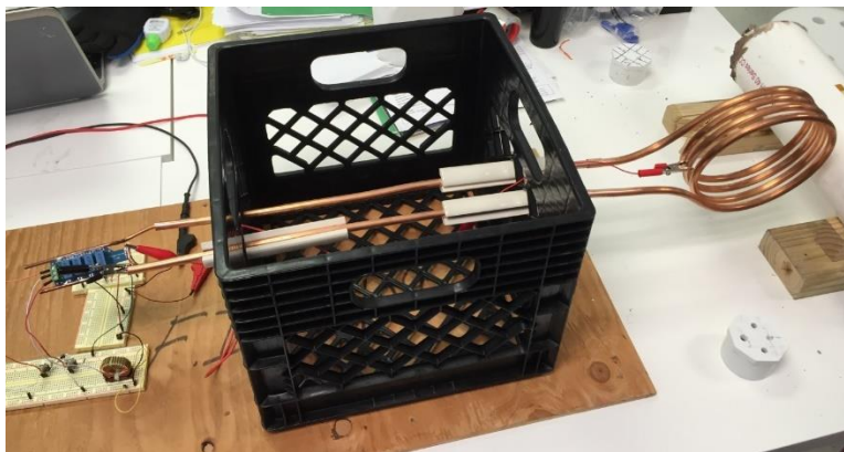
Figure A-1: Induction heater with the copper coil (inductor).
