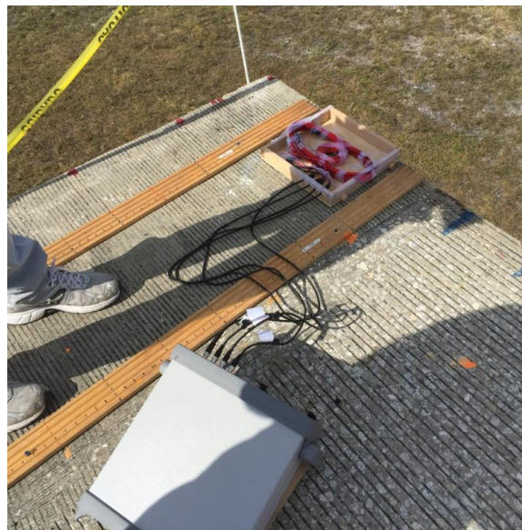
Figure 5-53: Modified second prototype elliptical coil used for inductance testing on the top slab of segment.
