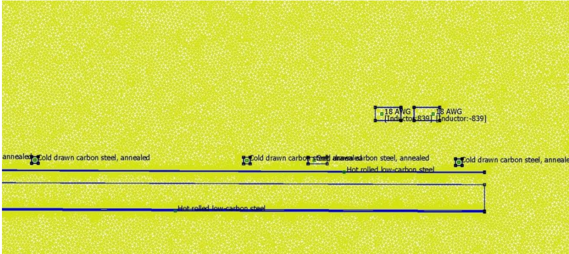
Figure B-3: Partial magnified cross-section elevation view of the finite element mesh of the segment model at the edge of the segment shows the conduit (hot-rolled low carbon steel) longitudinal and transverse strands (cold-drawn carbon steel, annealed) and inductor (839 turns of 18 AWG).
