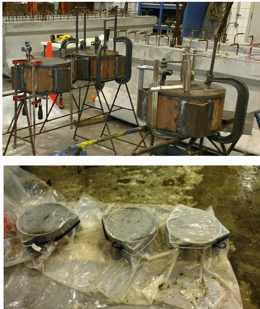
Figure 11 - Confined Specimens (Top) and Unconfined Specimens (Bottom)
