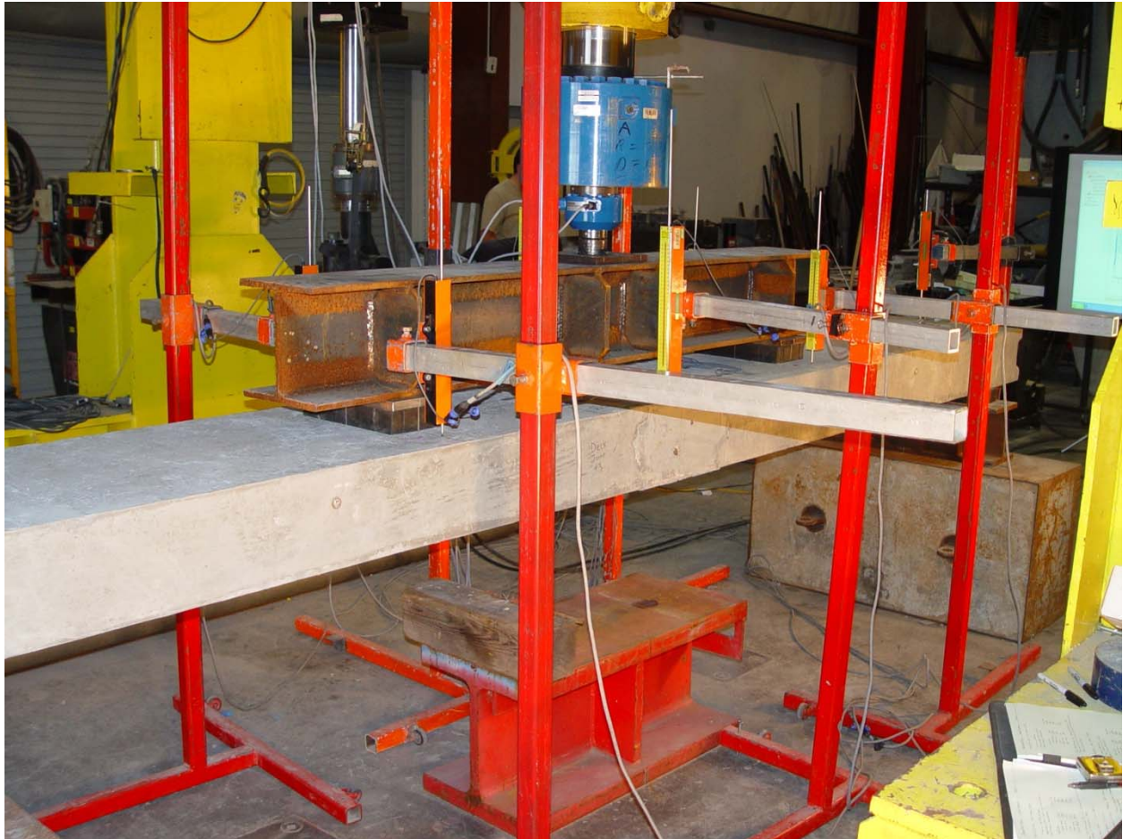
Figure 34 – Load Testing Setup
