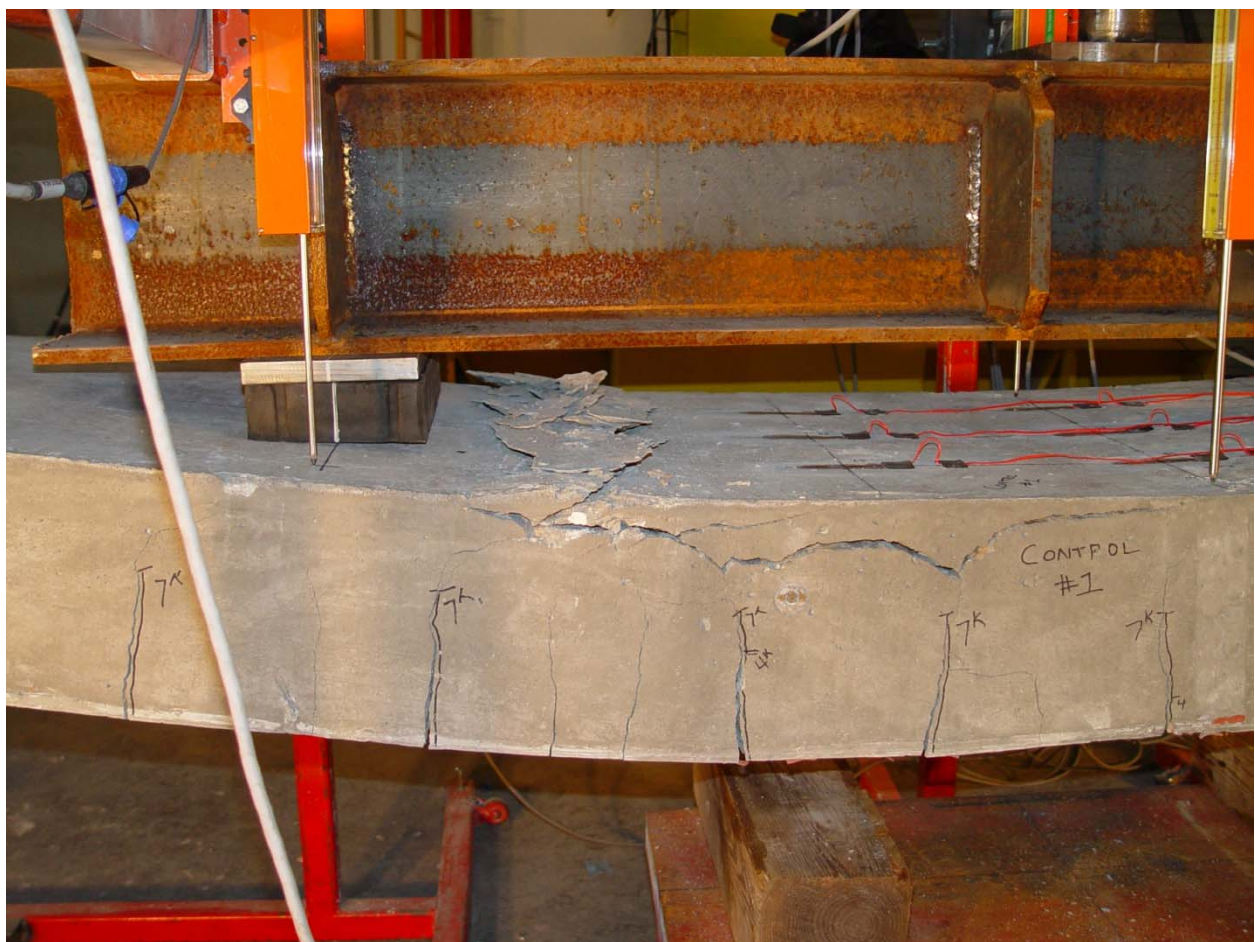
Figure 38 - Failure of Control Specimen #1
