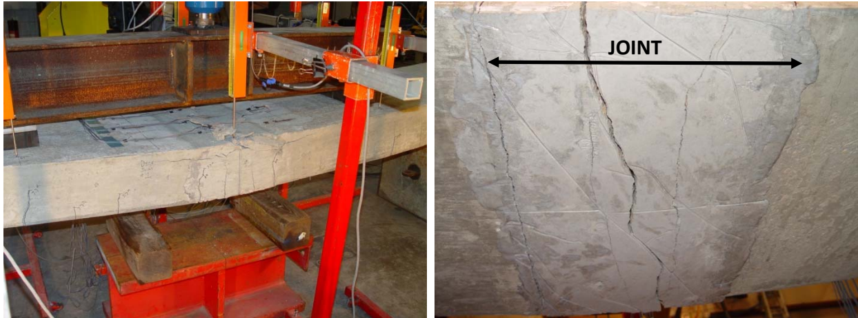
Figure 39 - Failure of Joint Specimens
