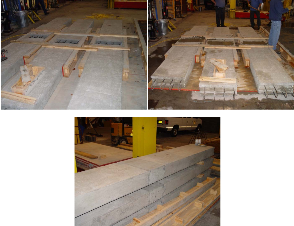
Figure 33 – Joining the Panels using the Lapping Hoop Joint
