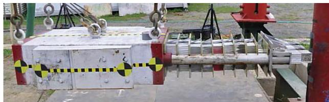
Figure 3.2 NCAC-FOIL 1100C crushable nose impactor
