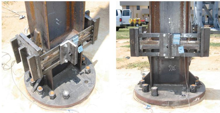
Figure 1.4 High capacity moment collar breakaway connection developed in FDOT project BDK75-977-40
