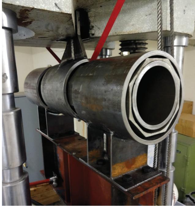
Figure D.2. Static double-shear test setup
