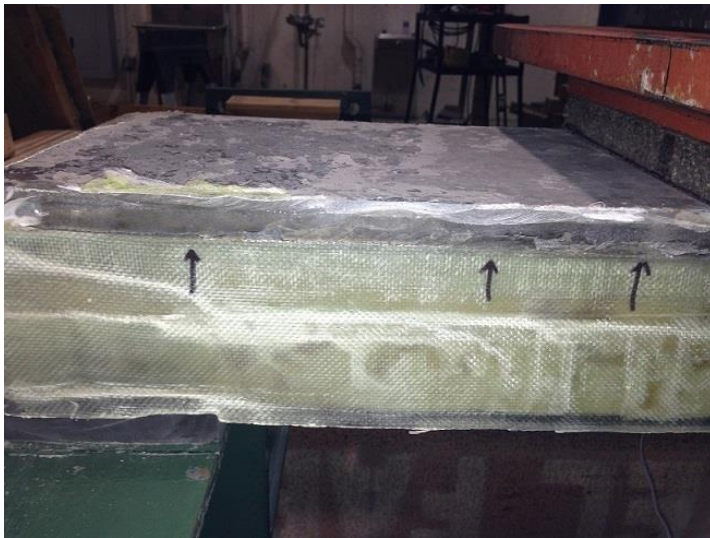
Figure 4.14 The Failure Mode near the End of the Grouted Region
