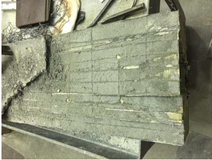
Figure 4.13 Bond between UHPC and Top FRP
