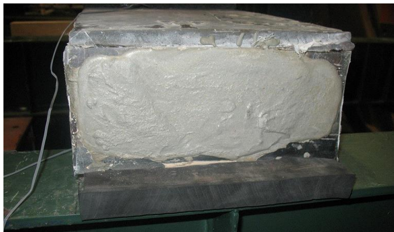
Figure 4.9 End of the Specimen after Grouting
