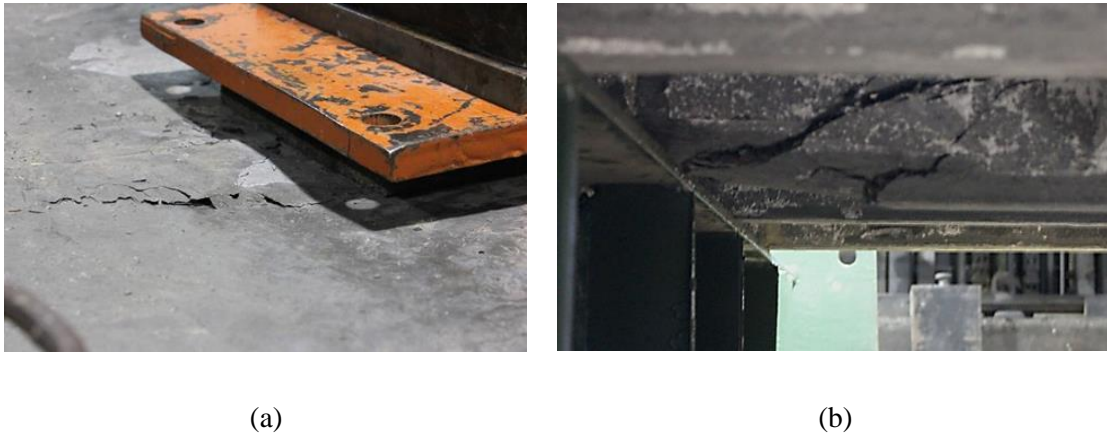
Figure 3.11 Failure Modes in Specimen 4T1S: (a) Top View, and (b) Bottom View
