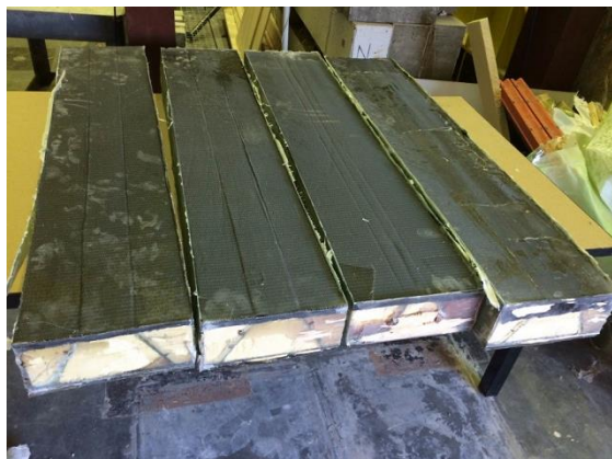
(f) Final deck after demolding
