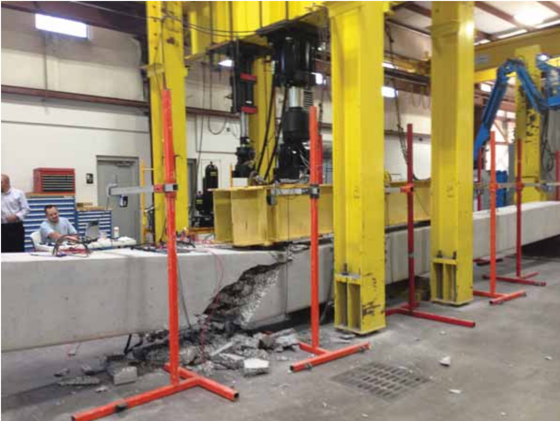
Figure 6.26: Failure under one of the load points
