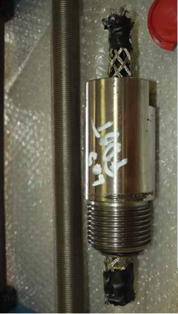
Photos of coupler from practice installation at FDOT on May 18. This coupler held a force of approx. 75% of CFCC ultimate strength.
