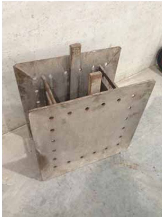
Figure H.2: Steel header used for a conventional steel-prestressed concrete pile (Replaced by wooden header for this research)
