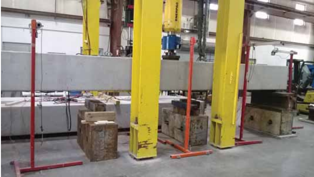
Figure 5.9: A pile being tested for development length
