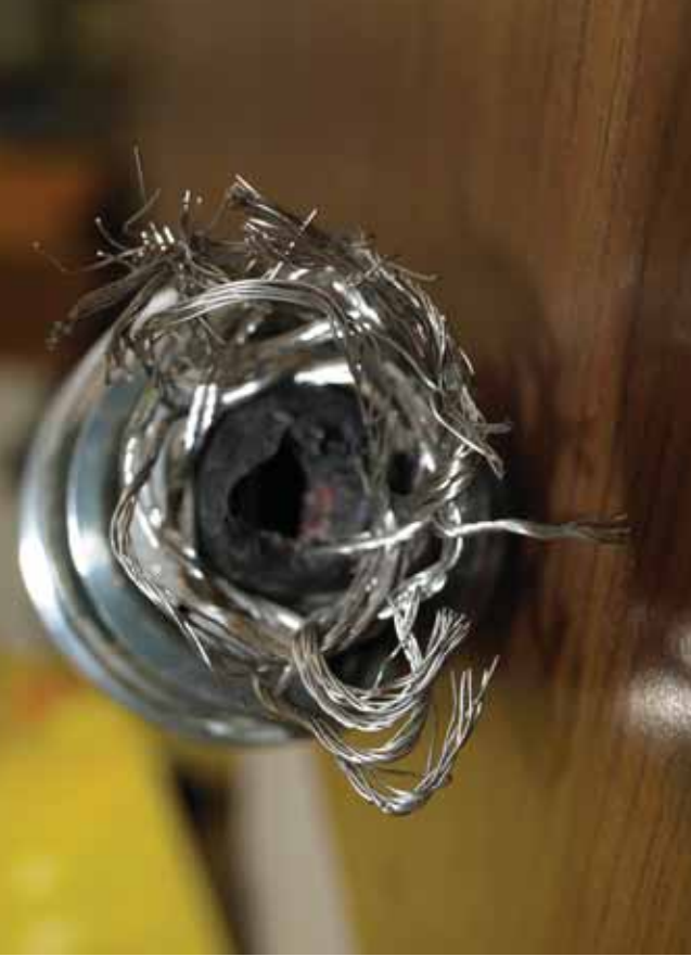
Photos of coupler that slipped under force of 70% of CFCC ultimate strength.
