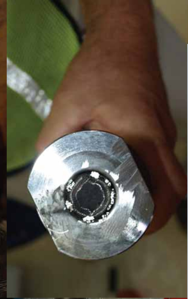
Photos of coupler from practice installation at FDOT on May 18. This coupler held a force of approx. 75% of CFCC ultimate strength.
