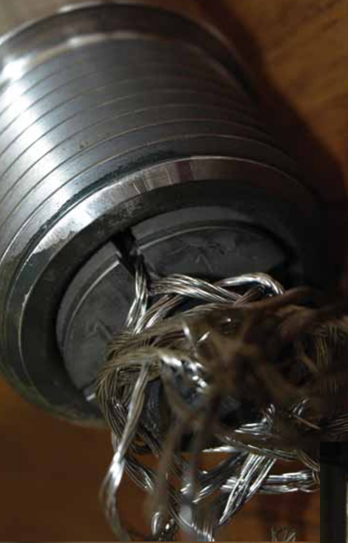
Photos of coupler that slipped under force of 70% of CFCC ultimate strength.
