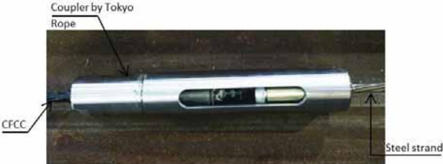
Figure 4.15: CFCC coupled with steel strand
