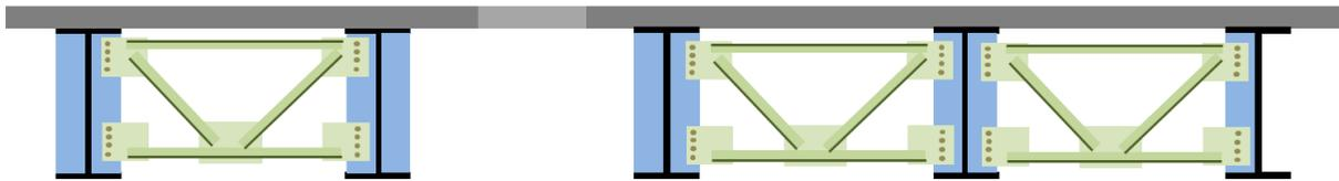
Figure 5-6. Elimination of cross-frames between construction phases
