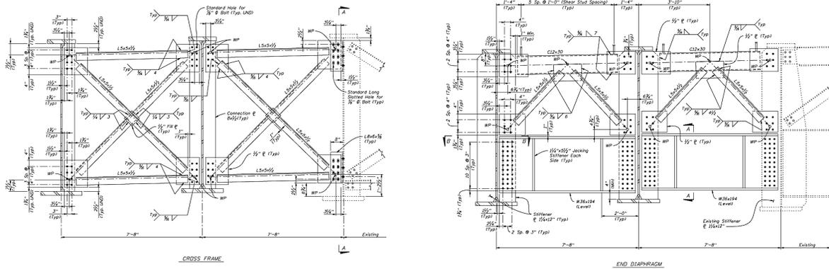
Figure 4-7. Cross-frame details of the bridge SR-589 over Waters Avenue
