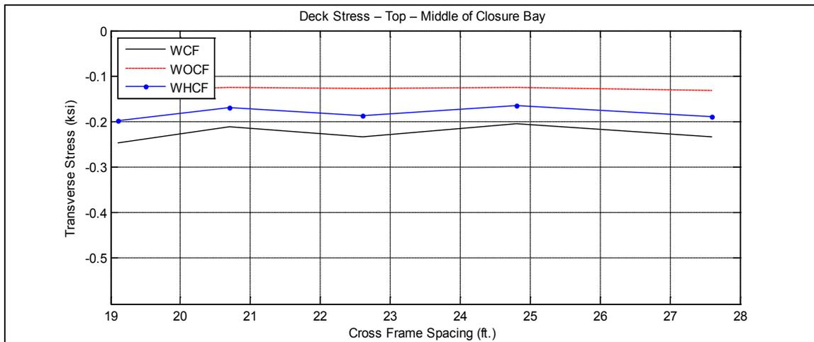
**Figure A-56. Transverse deck stresses at Bottom-middle of closure pour vs. cross-frame spacing for bridge SR-589 over Waters Avenue**
