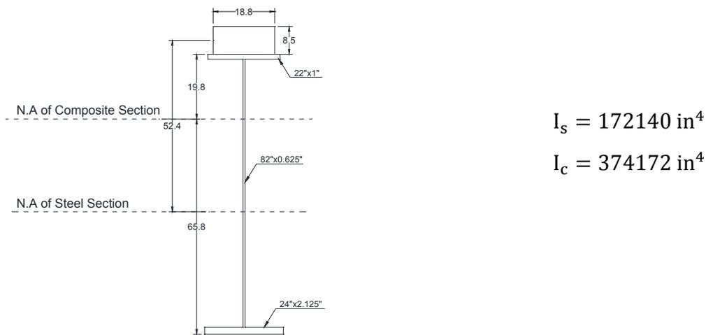
**Figure 6-12. Details of steel and composite cross-section**
