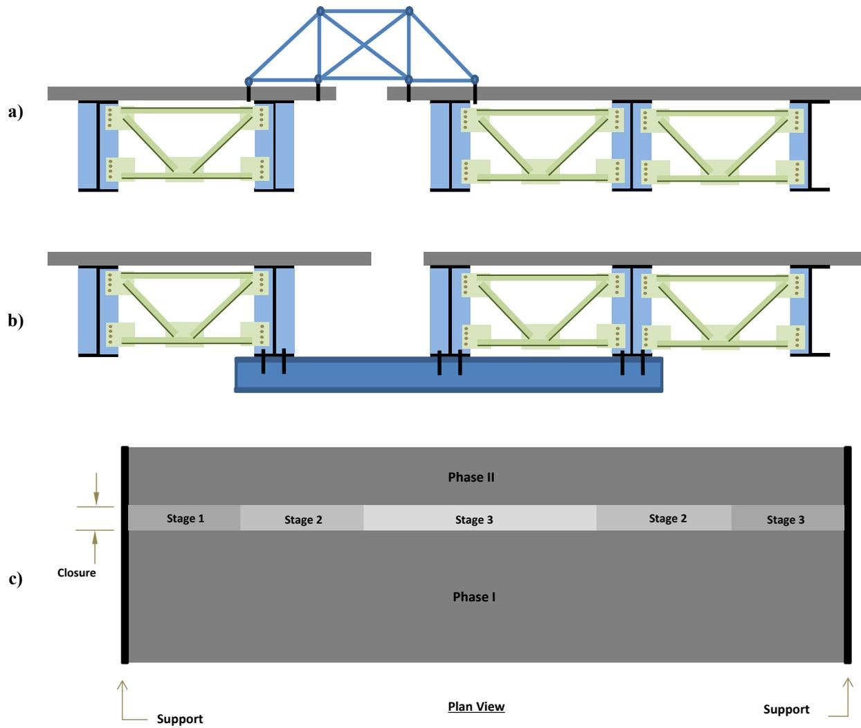
**Figure 5-7. Vibration mitigation methods**
