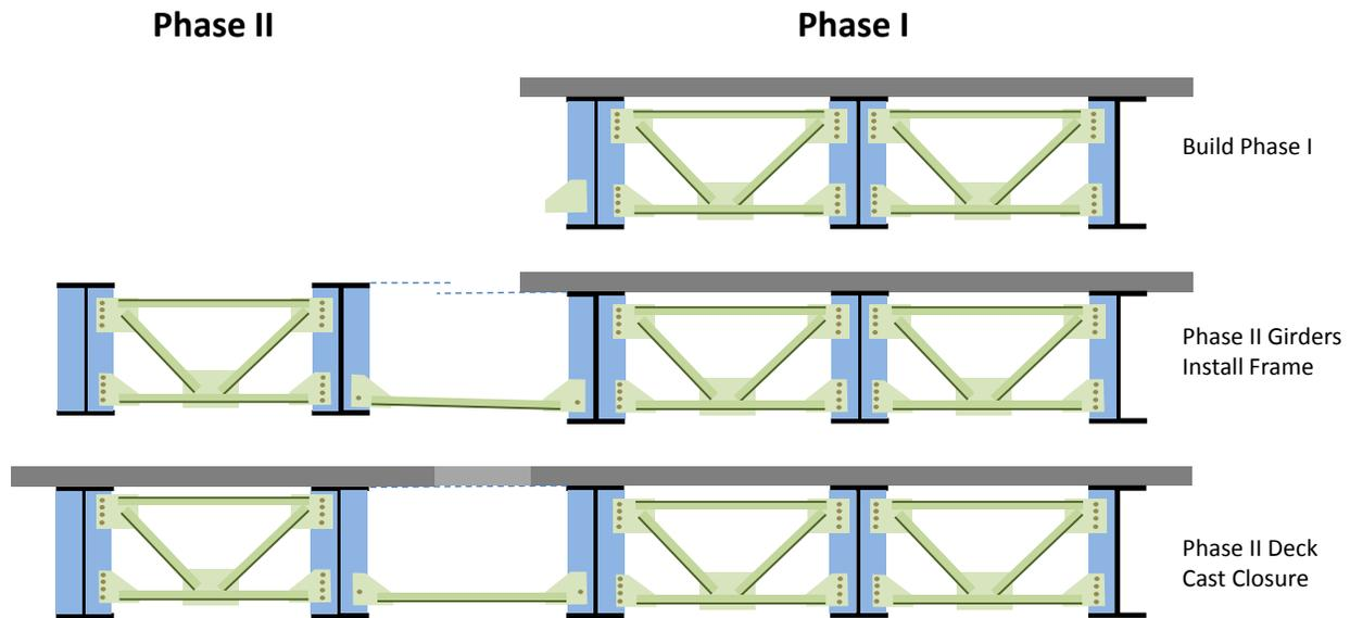
**Figure 5-3. Horizontal struts between construction phases**
