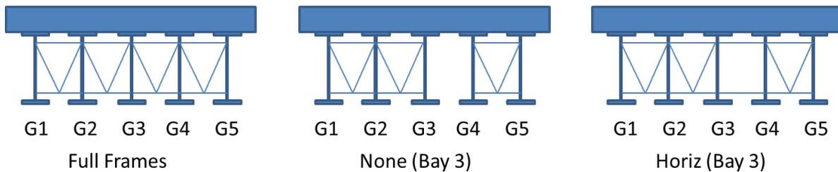
Figure 4-9. Three different investigated cases for bridge I-95 over SR-421
