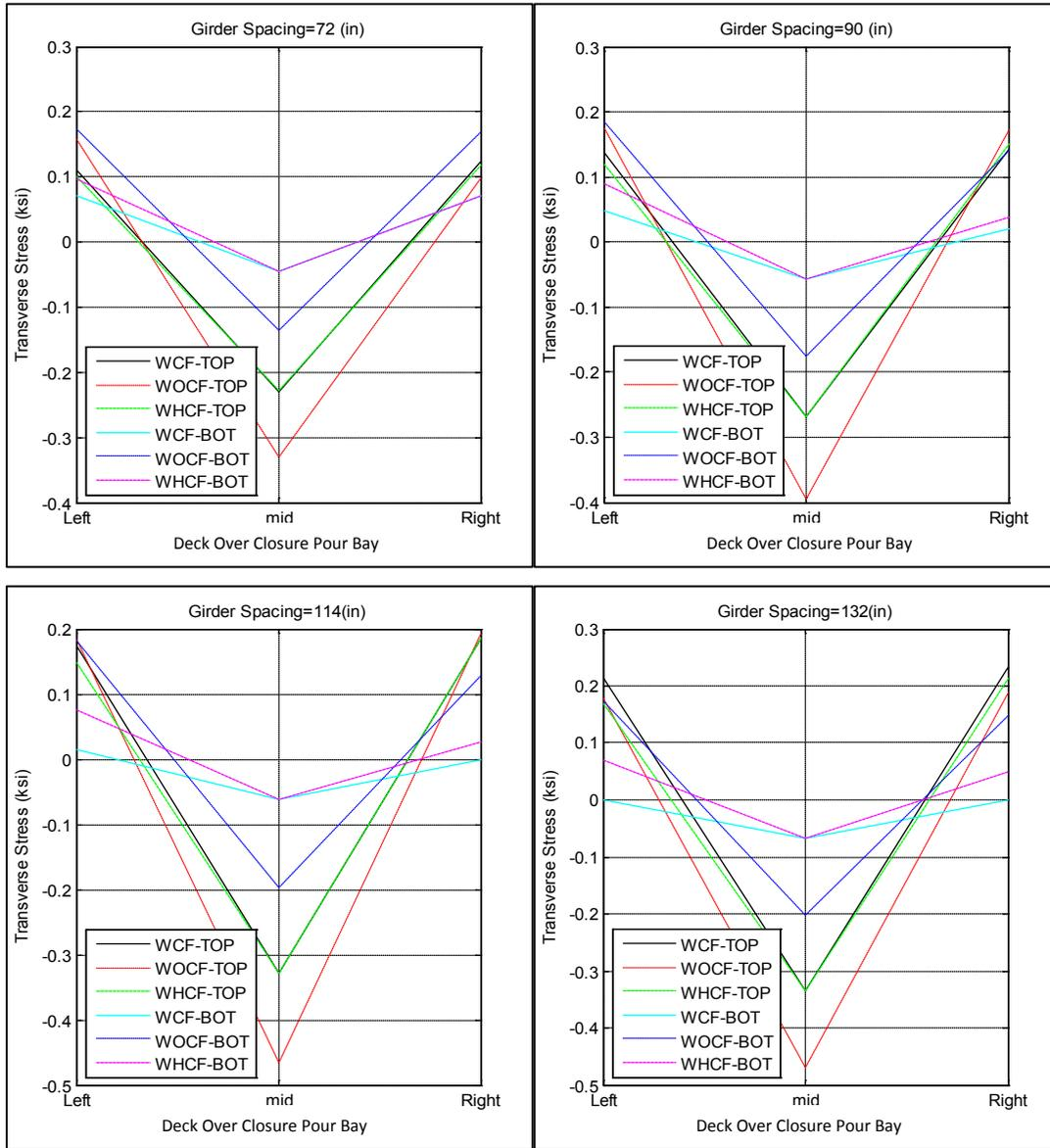
**Figure A-3. Transverse stress at closure pour related t to different girder spacing; 72, 90,114,132 inches for bridge I-95 over SR-421**
