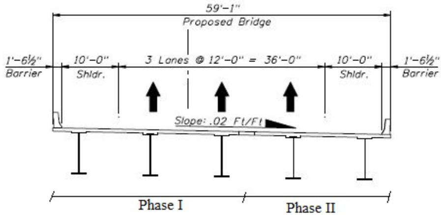
Figure 4-1. Cross-section of the bridge I-95 over SR-421
