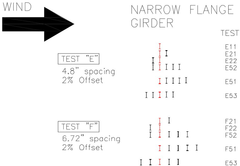
**FIGURE 1.7 TEST CONFIGURATIONS AND DESIGNATIONS – NARROW FLANGE PLATE GIRDERS (1:25 SCALE, RED – TESTED GIRDER)**
