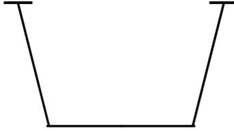
Figure 3.7 Example open-top box girder cross-section for which  $C_p = 1.5$  (per FDOT, 2012e)
