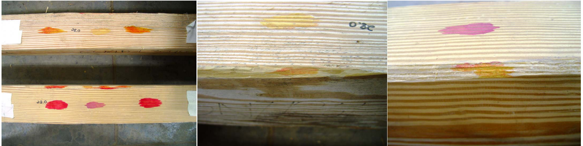
Figure 17: Use of Phenol Red in Identification of TimberSIL Product vs. Regular Wood TimberSIL below regular wood (left), Regular Wood corner view (middle), TimberSIL corner view (right)
