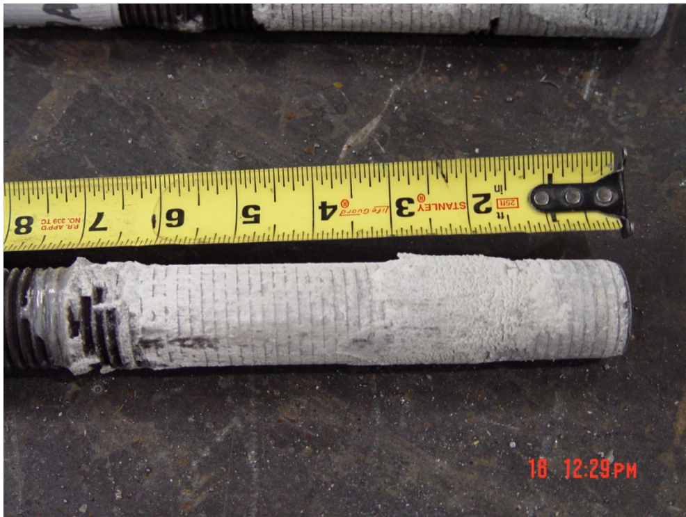
Figure 14: Combination of Mechanical and Bond Failure – Non-Wrapped
