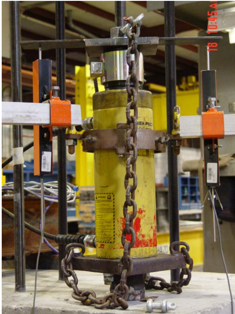
Figure 2: Confined Tension Test
