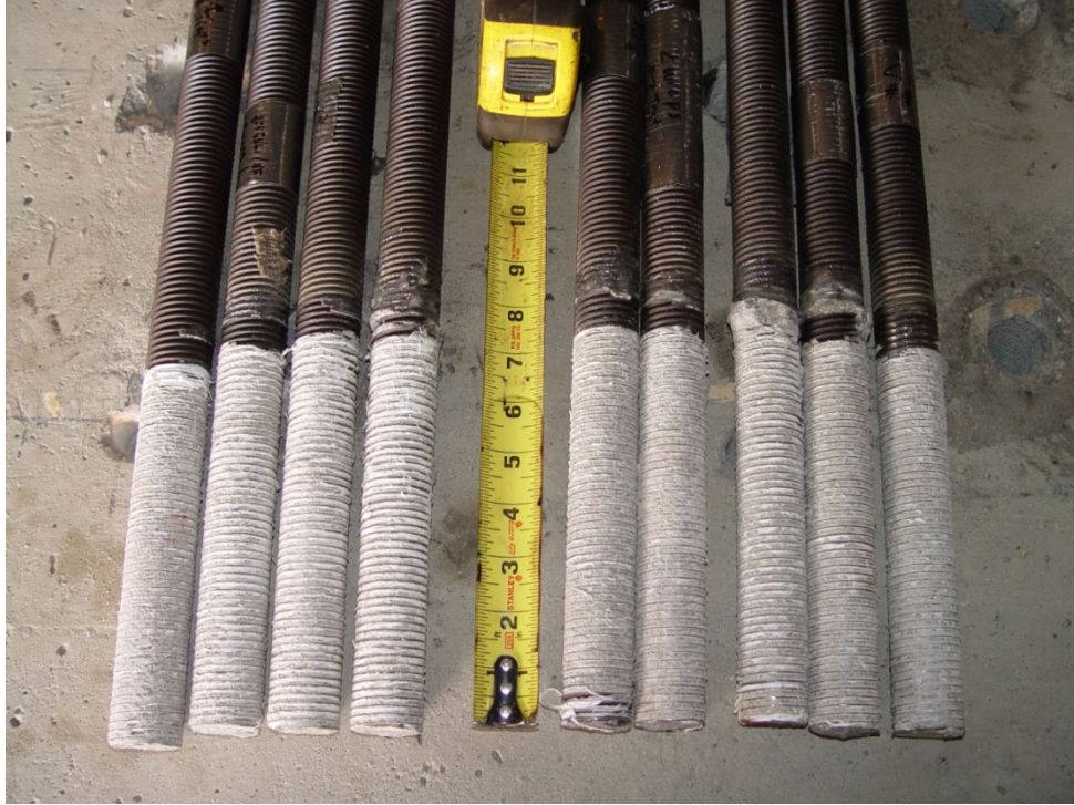
Figure 13: Mechanical Failure – Wrapped Specimens
