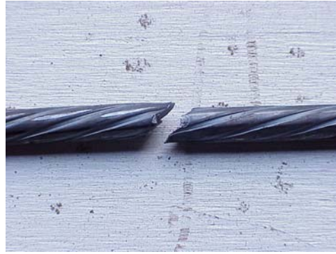
Figure 10 – Angled Fracture of Bar
