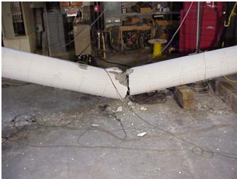
Figure 16 – Fatigue Specimen at Failure
