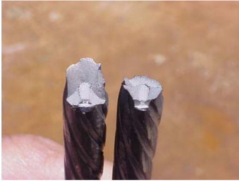
Figure 9 – Close-up View of Failure Plane Showing Depth of Heat Penetration
