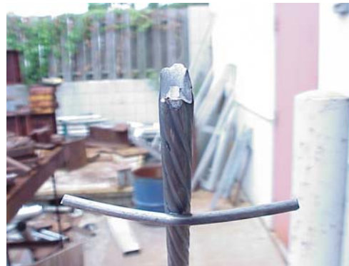
Figure 8 – Fracture Through Weld With Spiral Reinforcement Shown
