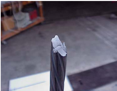
Figure 7 – Fracture Through Weld
