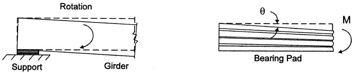
Figure 3.6: Rotational Forces on Girder and Bearing Pad
