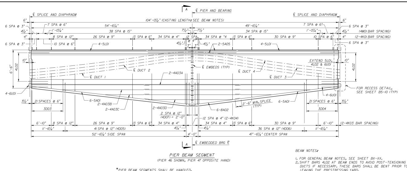
\*PIER BEAM SEGMENTS SHALL BE HANDLED. STORED AND TRANSPORTED BY THESE POINTS.
