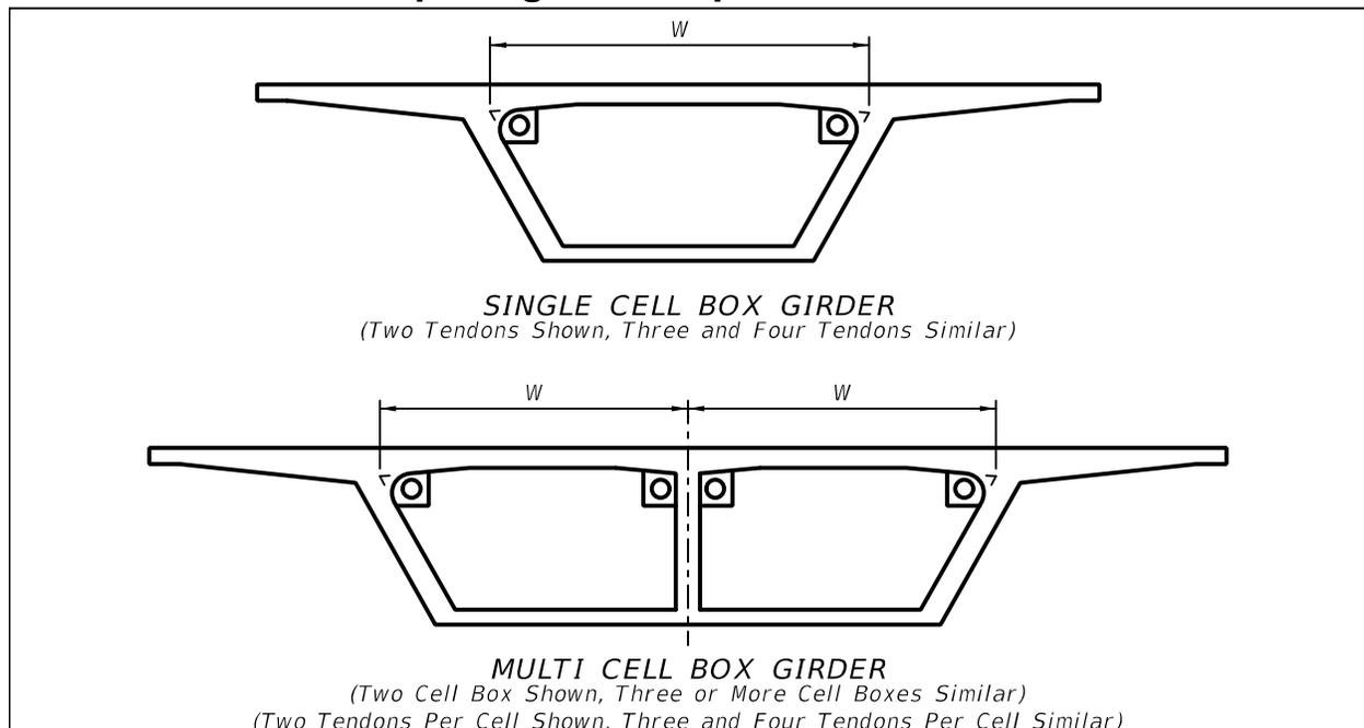
*Commentary: This is a minimum requirement and is not to be added to those required by the longitudinal analysis, i.e. if the number and size of top slab tendons across closure pours required by the longitudinal analysis exceeds these minimums, no additional tendons are required.*
