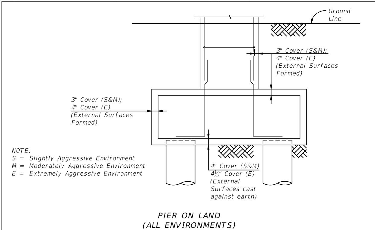
**Figure 1.4.2-5 Pier Cap and Intermediate Bent (All Environments)**
