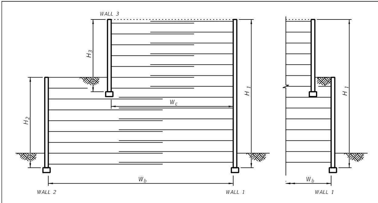
P. For stacked walls to be considered separately for internal stability, determine the minimum offset distance "D" as shown in Figure 3.13.2-9 using the following equation:
