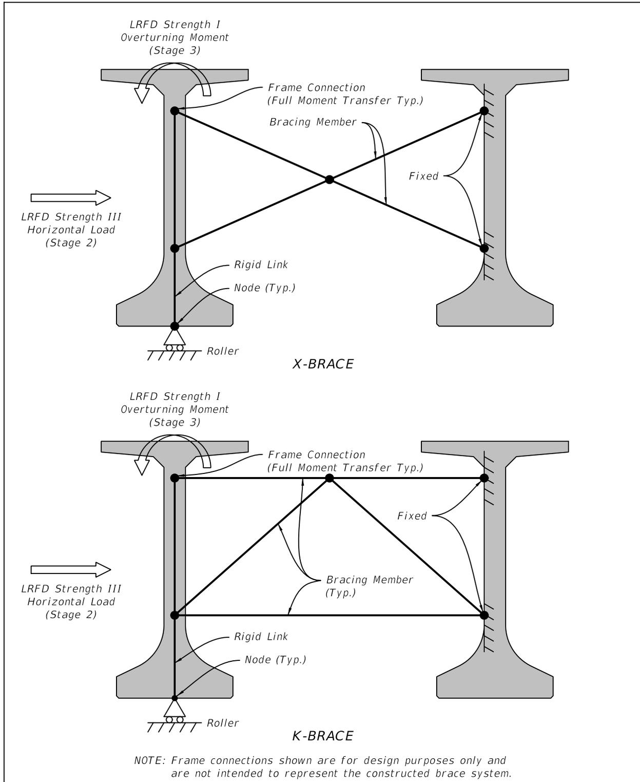
C. In addition to designing individual brace members based on the member forces, check the final brace system capacity  $C \geq 1.0$  of FIB beams using the following equations (not required for AASHTO Type II beams):
