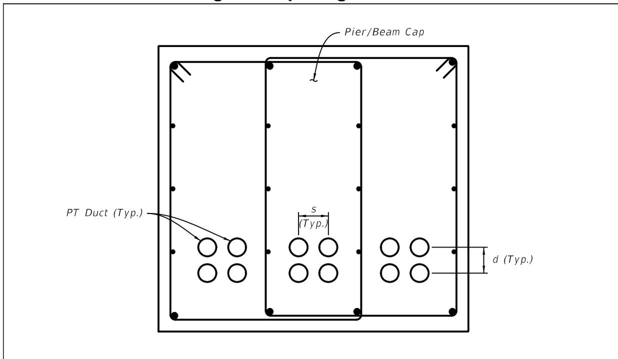
**Figure 3.11.1-2 Section Through Post-Tensioned Columns Showing Duct Spacings**
