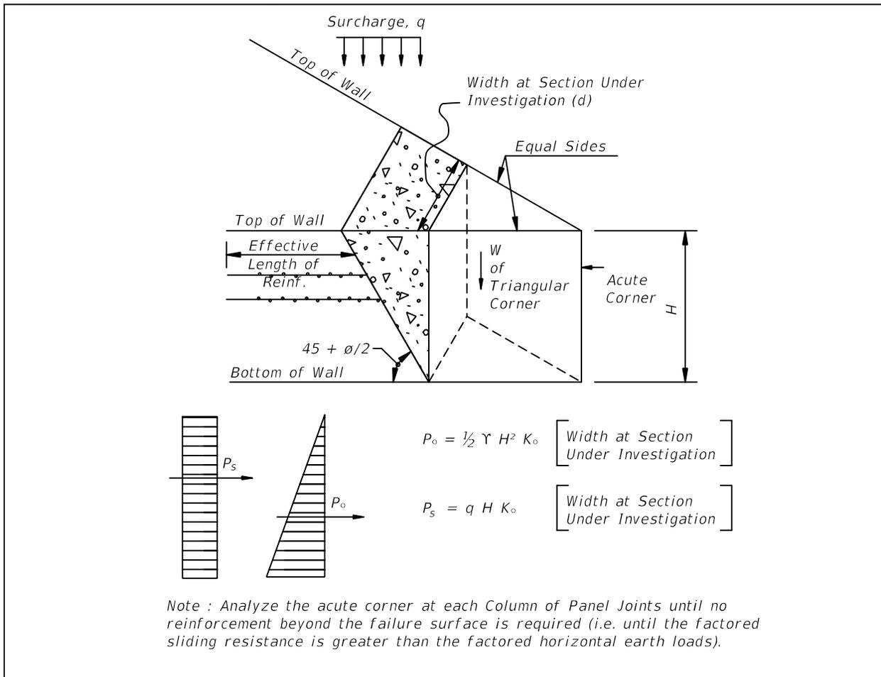
**E. Minimum Length of Soil Reinforcement [11.10.2.1]**
