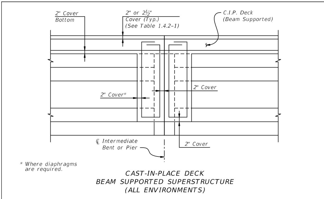
B. When deformed reinforcing bars are in contact with other embedded items such as post-tensioning ducts, the actual bar diameter, including deformations, must be taken into account in determining the design dimensions of concrete members and in applying the design covers of Table 1.4.2-1.
