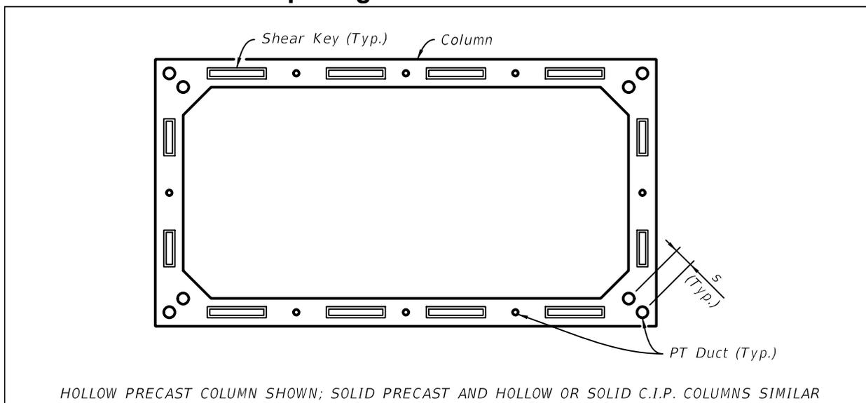
**Table 3.11.1-3 Minimum Dimensions for Substructure Elements Containing Post-Tensioning Tendons**
