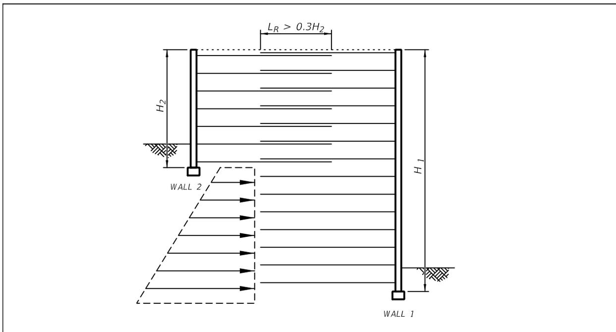
For Case 2 geometries where the horizontal earth pressure acting on Wall 2 is assumed to be zero for external stability:
