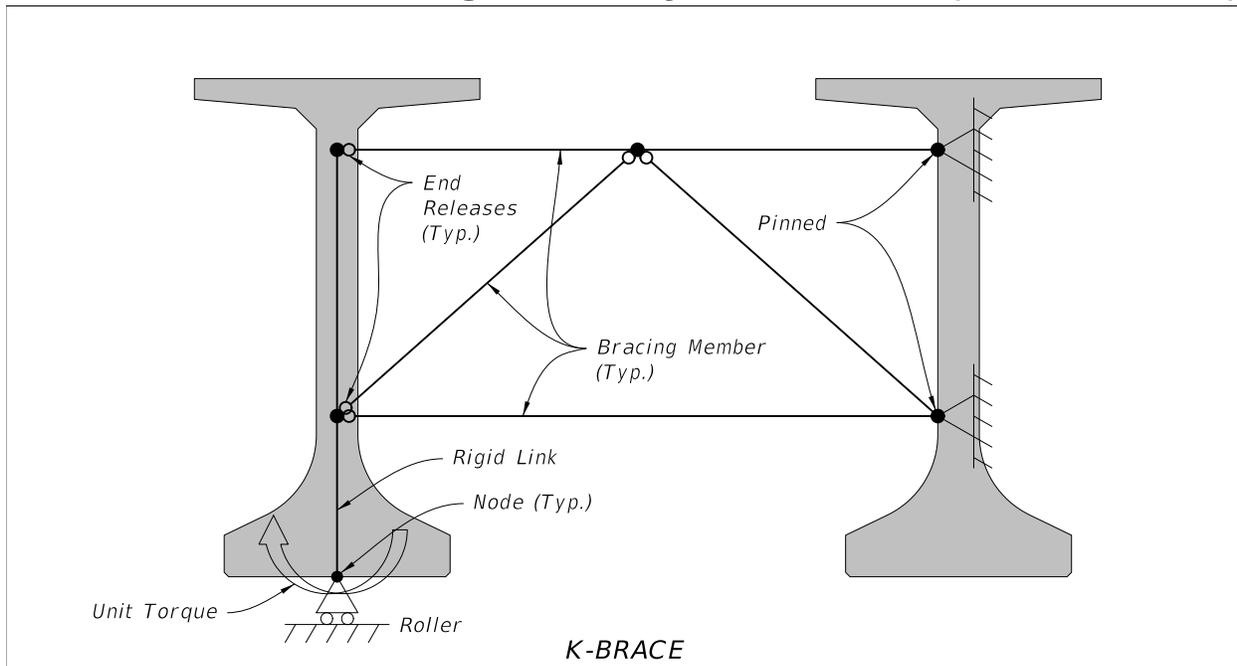
D. Additional analysis methods for bracing design can be found in References 1 and 2. For braced beams during Stage 3, a data base method generated from 3D finite element models to calculate K-brace or X-brace forces directly is available (see Reference 2).
