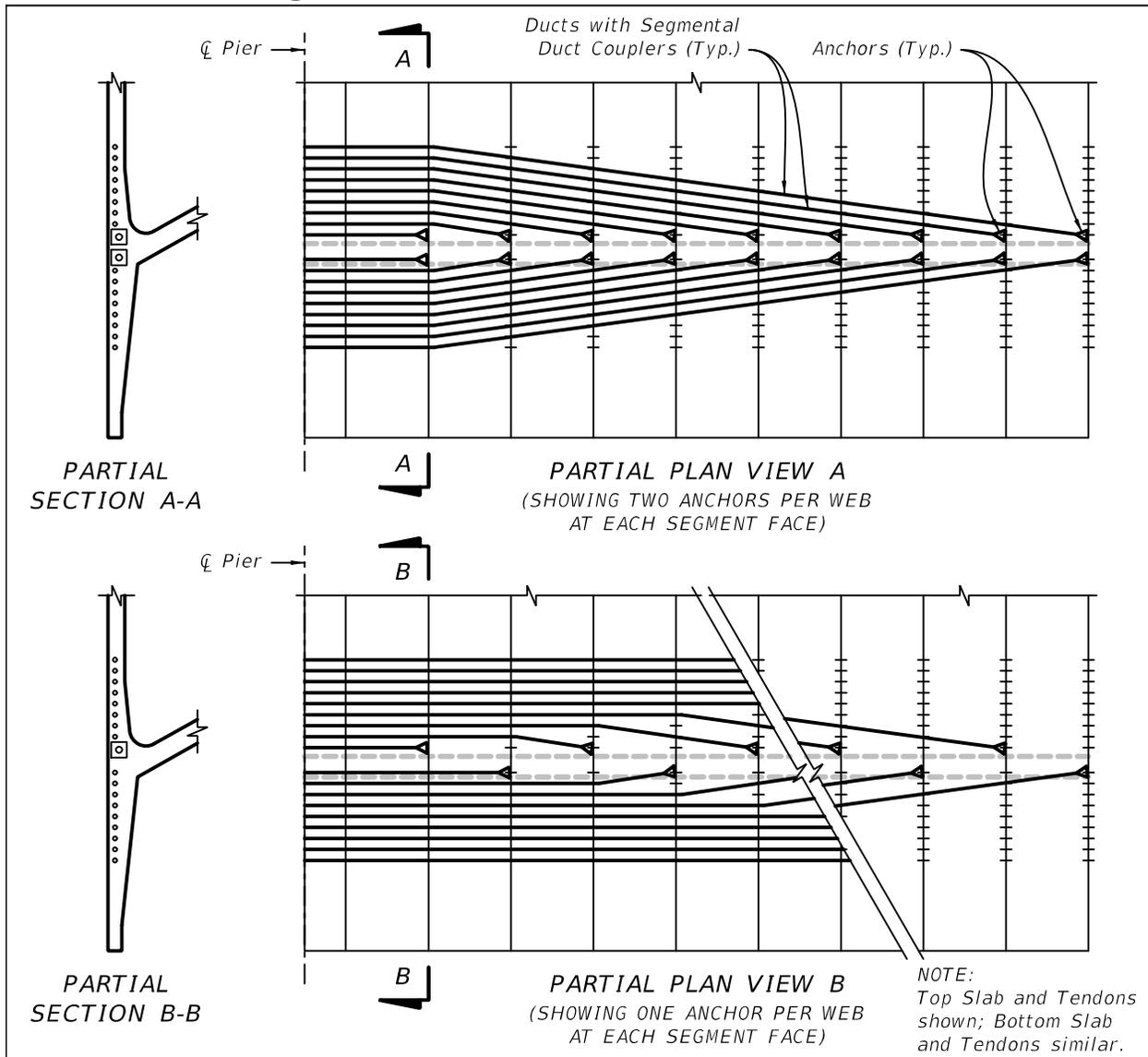
**Figure 4.6.3-2 Cantilever Tendon Layout Schematic for Cast-In-Place Box Girders**
