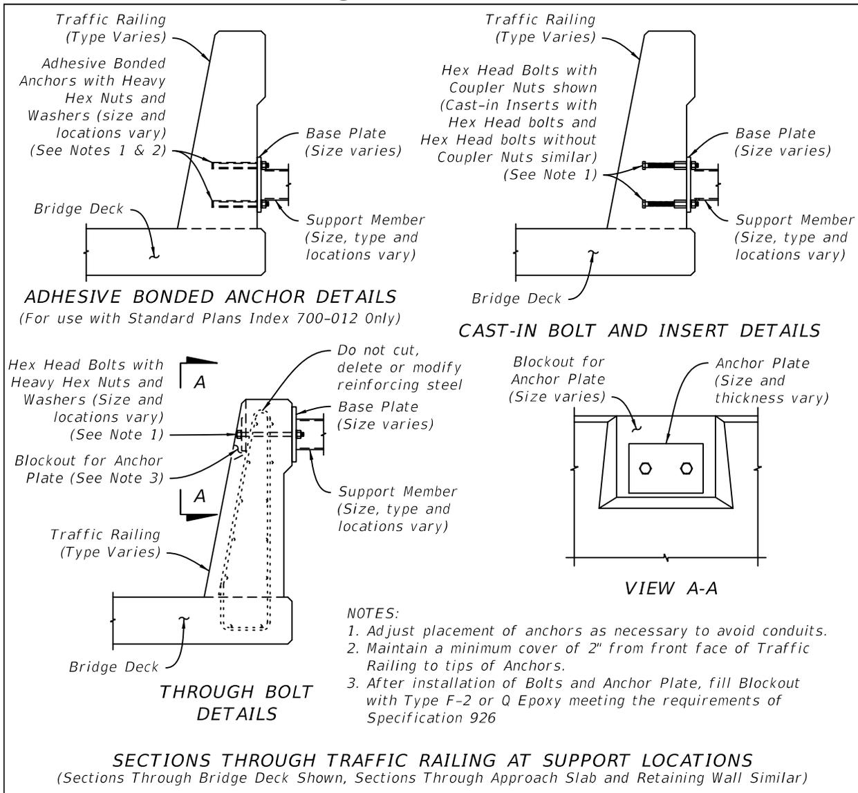
E. When field drilling of existing structures at locations shown in [Appendix 1A](#) is permitted by the DSDE, include plan notes and/or develop Technical Special Provisions to address special requirements, e.g. locating reinforcing steel, prestressing steel and/or post-tensioning tendons in existing concrete structures prior to field drilling, drilling into any steel members, etc.
