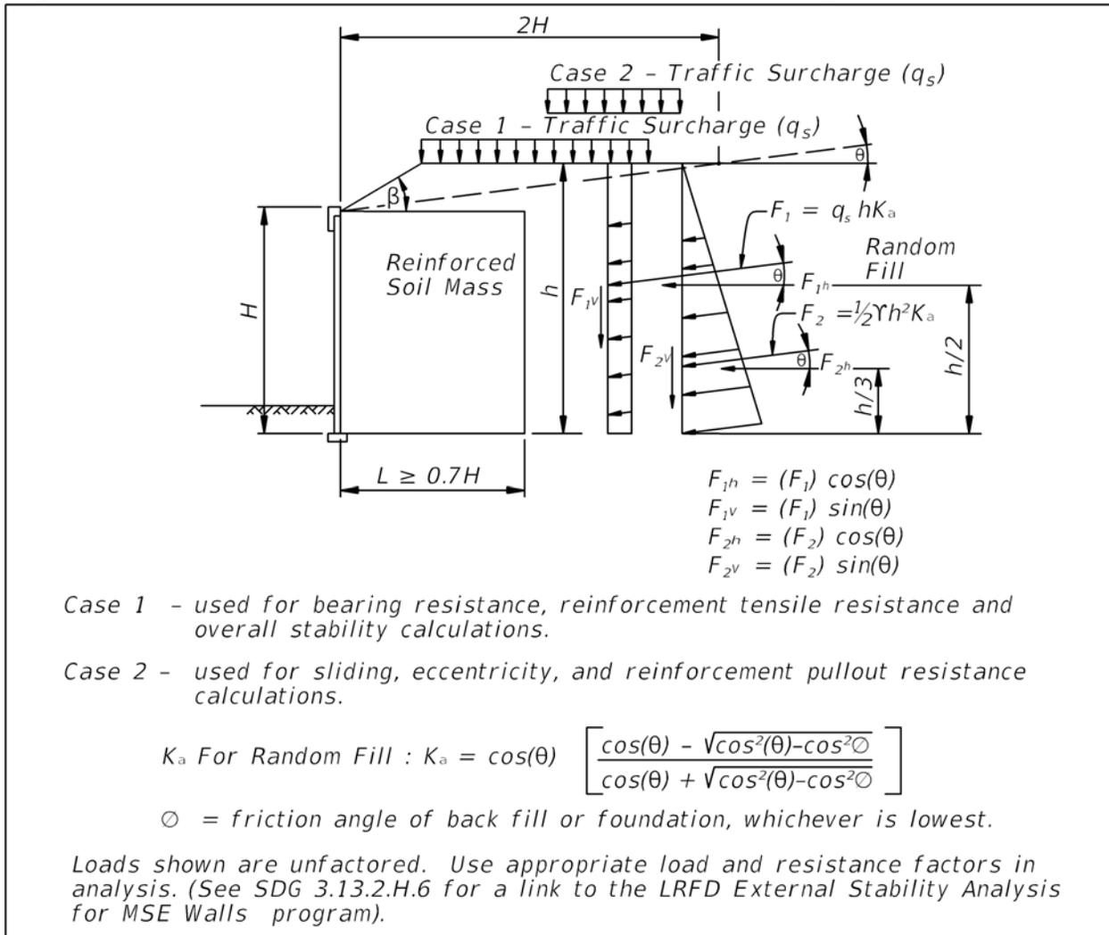
**Figure 3.13.2-4 Broken Backfill without Traffic Surcharge**
