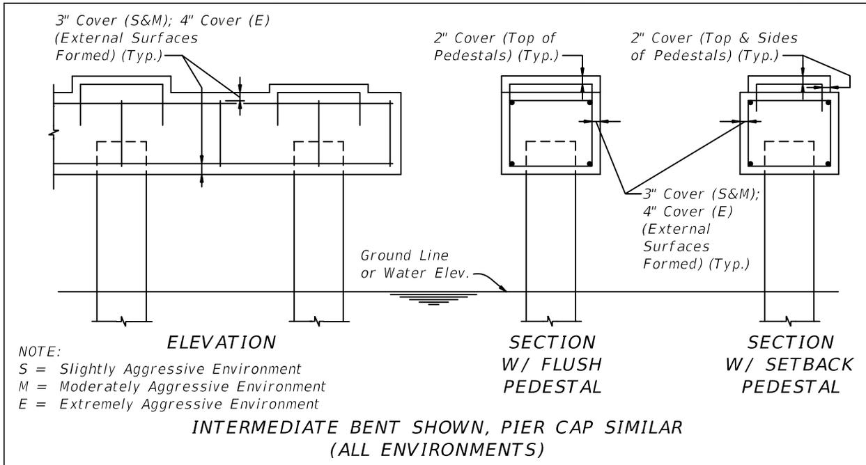
**Figure 1.4.2-6 Cast-in-Place Deck / Beam Supported Superstructure (All environments)**
