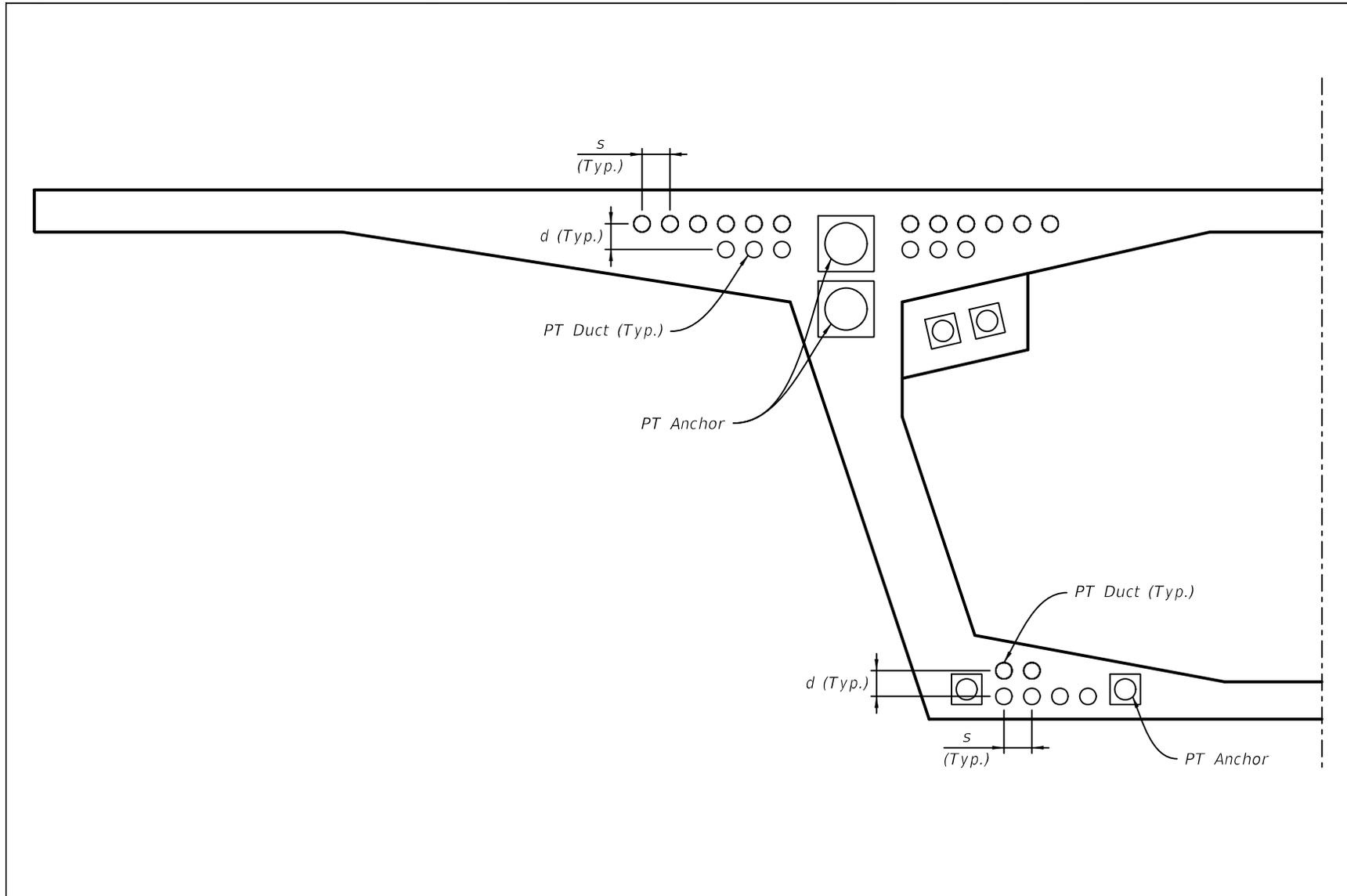
**Figure 4.5.3-2 Section Through Post-Tensioned I-Girder Showing Duct Spacings**
