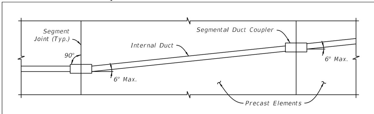
*Commentary: Segmental duct couplers shall be made normal to joints to allow stripping of the bulkhead forms. Theoretically, the tendon must pass through the coupler without touching the duct or coupler. Over-sizing couplers allows for standardized bulkheads and avoids the use of curved tendons.*
