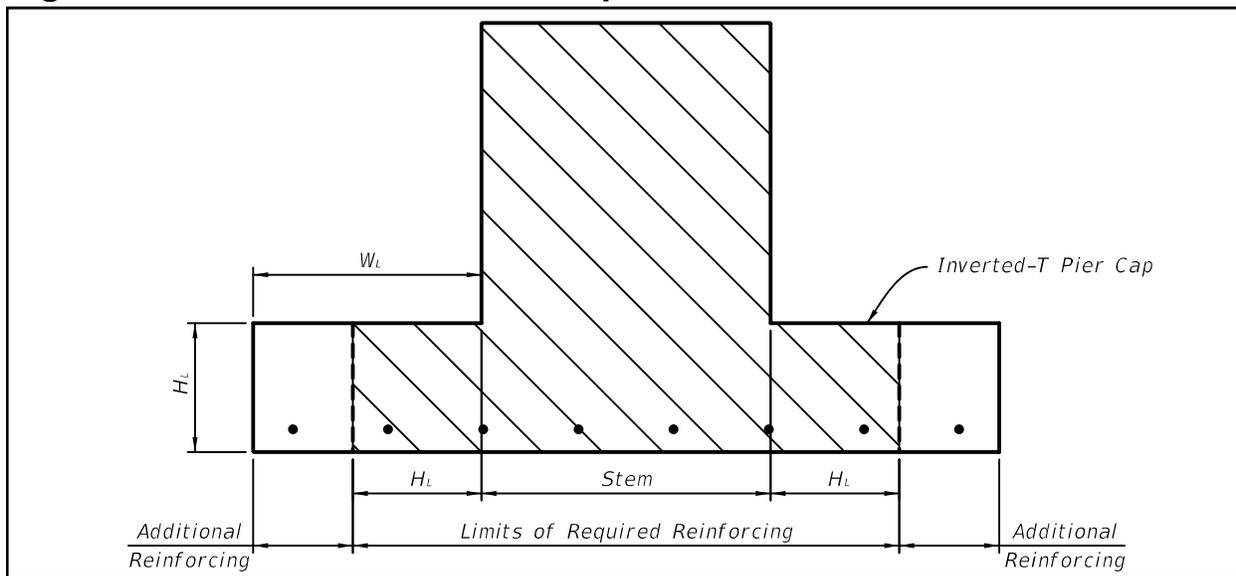
**Figure 3.11.4-2 Inverted-T Pier Cap Supplementary Reinforcement Details**
