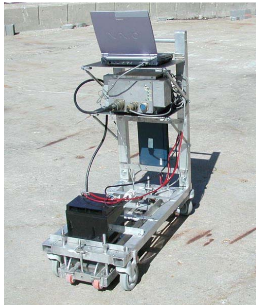
Figure 5.3 – Photograph of the MFL equipment as configured for testing internal P-T tendons in a bridge deck
