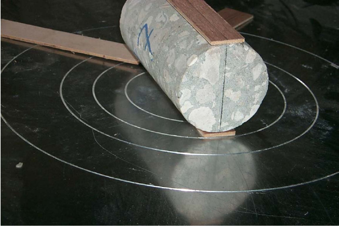
Picture 22 – Split Tensile Test on Core #7. Joint Vertical
