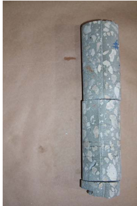
Picture 8 – Core#6 Split Cylinder Cut from Middle
