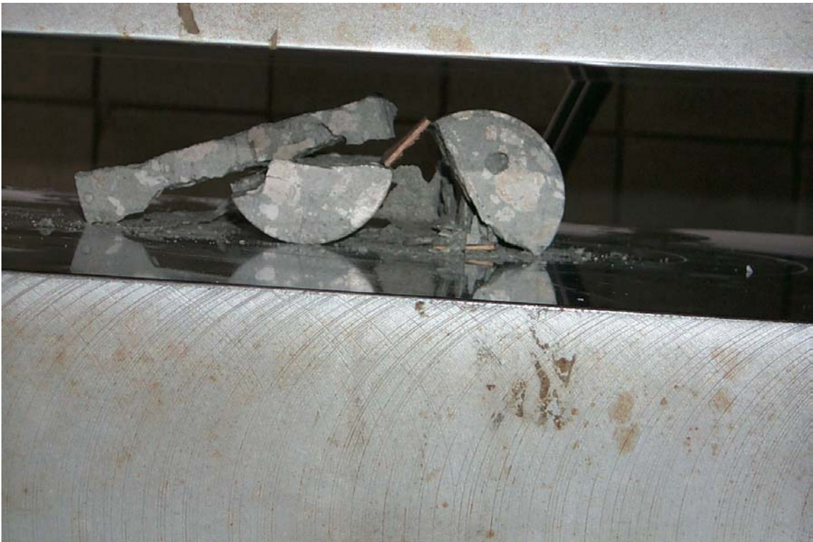
Picture 19 – Split Tensile Test on Core 6
