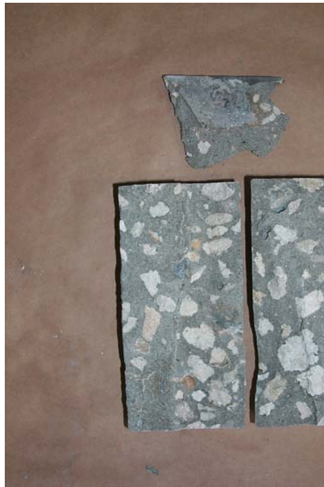
Picture 25 – Split Tensile Test on Core #2.
