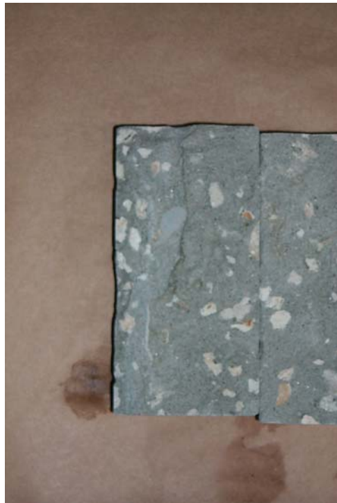
Picture 21 – Split Tensile Test on Core 6
