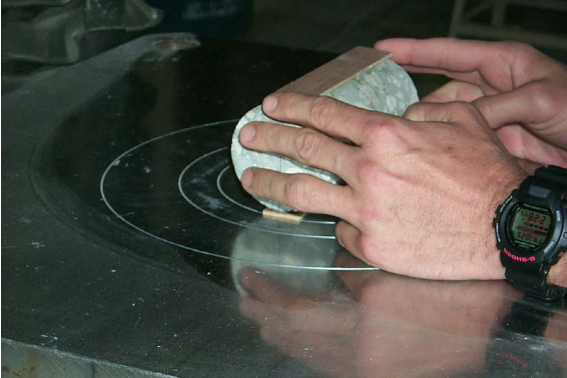
Picture 16 – Split Tensile Test on Core #6
