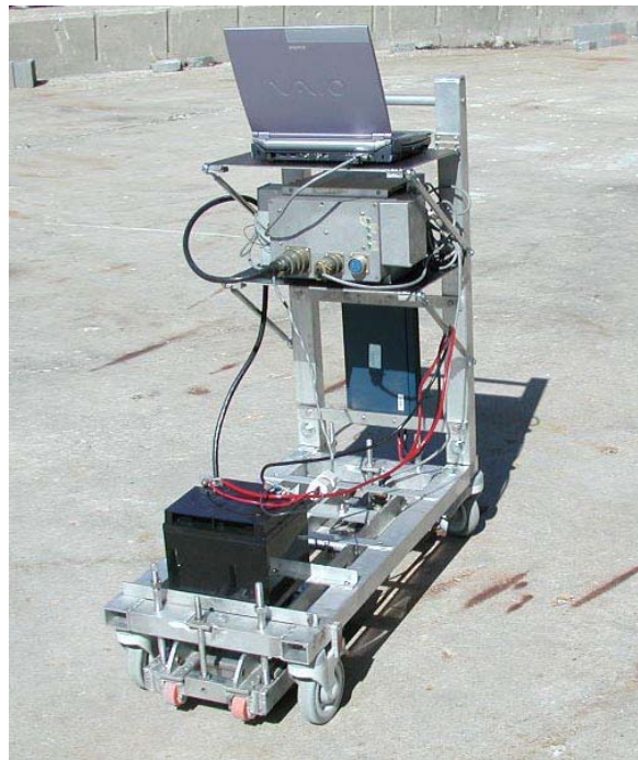
Figure 2 – Photograph of the MFL equipment as configured for testing internal P-T tendons in a bridge deck
