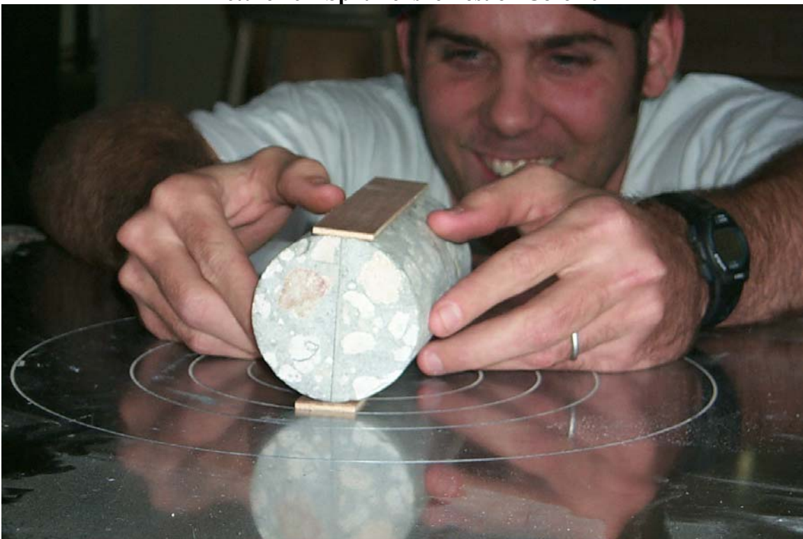
Picture 17 – Split Tensile Test on Core 6. Joint Vertical
