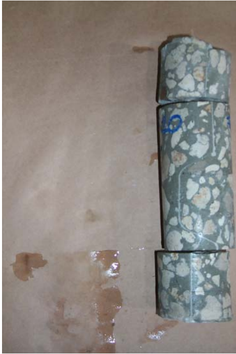
Picture 9 – Core #19 Split Cylinder Cut from Middle
