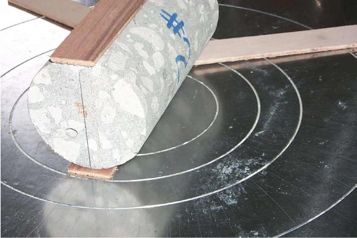
Picture 24 – Split Tensile Test on Core #2. Joint Vertical
