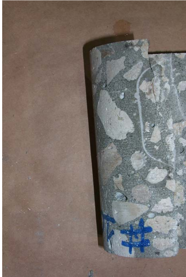
Picture 28 – Split Tensile Test on Core #10
