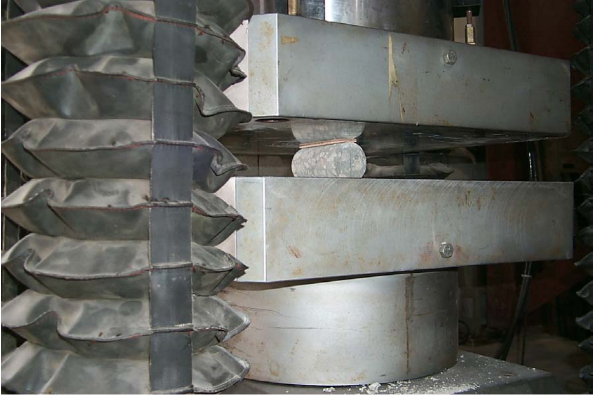
Picture 18 – Split Tensile Test on Core 6
