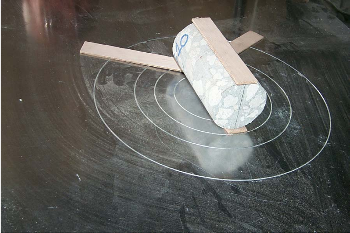
Picture 26 – Split Tensile Test on Core #10. Joint Vertical
