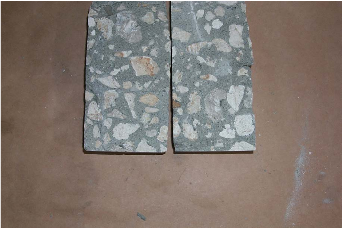
Picture 27 – Split Tensile Test on Core #10
