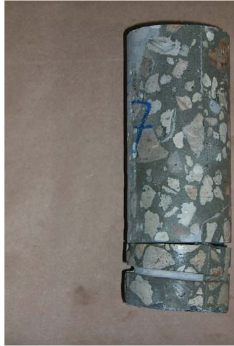
Picture 10 – Core #7 Split Cylinder Cut from Middle
