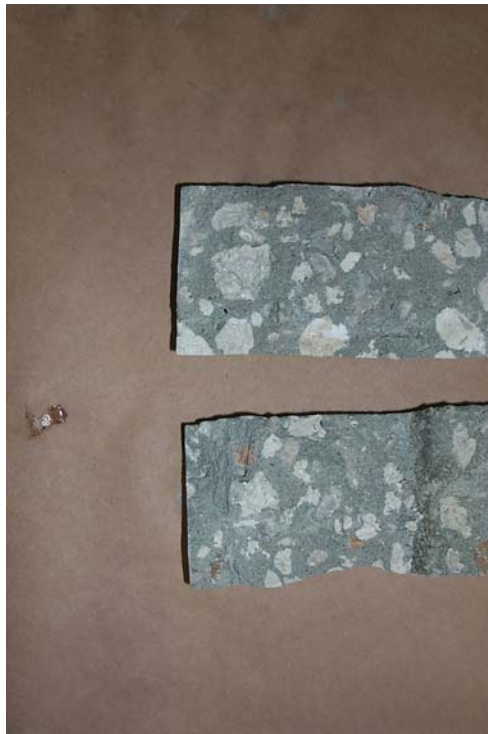
Picture 23 – Split tensile Test on Core #7
