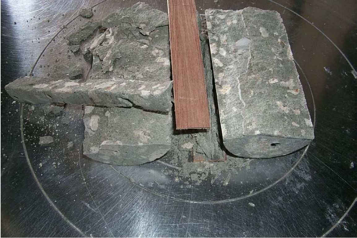
Picture 20 –Split Tensile Test on Core 6
