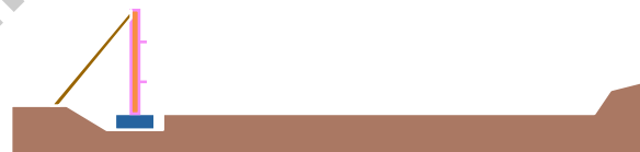
Figure 34, Install & Brace 1st Row of Panels
