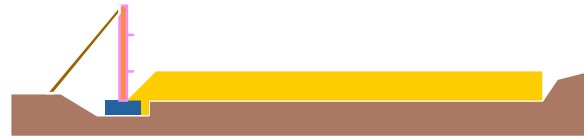
Figure 36, Fill in 6" Lifts to Reinforcement
