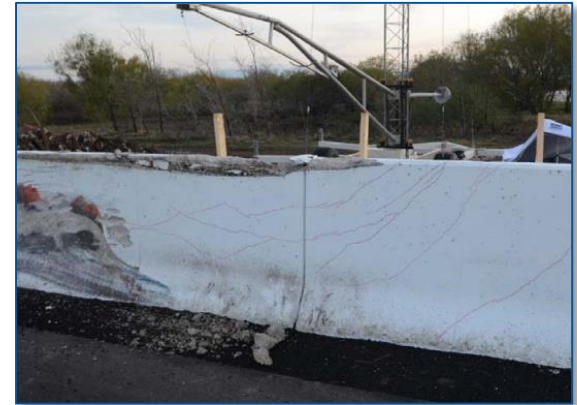
Photograph: GFRP reinforced traffic railing from successful TL-5 crash test (Pultrall)
