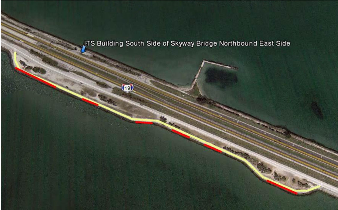
Recommended Limits of West Seawall Cap Repair
