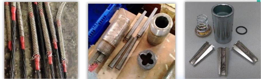
(a) & (b) Tensioning apparatus for CFRP; versus (c) standard steel HSCS chucks, for GFRP.
