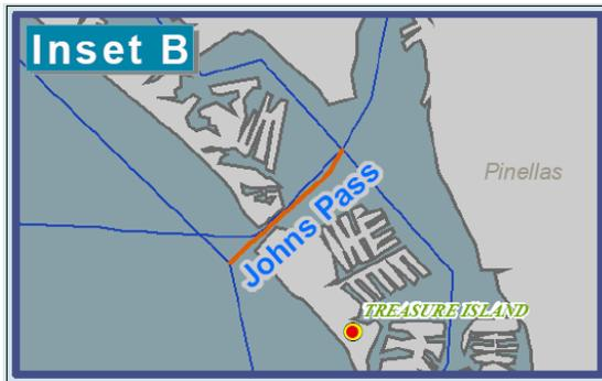
Johns Pass is a natural pass created after a hurricane split Madeira Beach in 1848 and is located in Pinellas County. The pass connects the GIWW to the Gulf of Mexico. It is two miles long and has an authorized depth of 13 feet.
