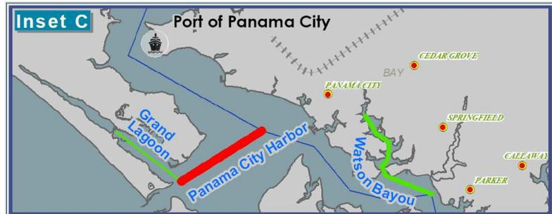
Watson Bayou flows in to St. Andrews Bay in Bay County. The bayou is home to many boat slips and marinas due to its recognition of being one of the safest harbors in Northwest Florida. This bayou is three miles long and has an authorized depth of 10 feet. In 2006, it carried 14,000 tons of cargo and the top commodity was hydrocarbon and petrol gases.
