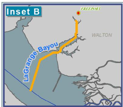
LaGrange Bayou is a natural water body located near the Choctawhatchee Bay in Walton County. It connects the city of Freeport with the GIWW. It is seven miles long and has an authorized depth of 12 feet. In 2006, it reported 553,000 tons of cargo and the top commodity was petroleum and petroleum products.
