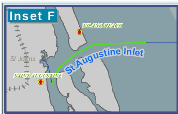
St. Augustine Inlet was originally a natural inlet that was relocated to its current location in 1940. The inlet is located in St. Johns County and connects the Tolomata and Matanzas Rivers and the AIWW to the Atlantic Ocean. The inlet is the entrance channel to the St. Augustine Port. It is four miles long and has an authorized depth of 16 feet.
