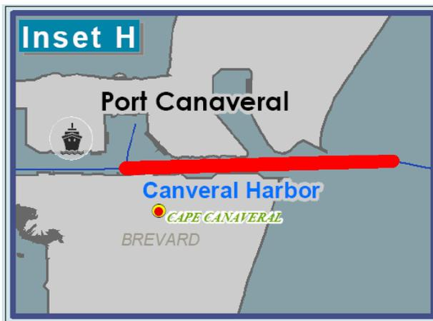
Canaveral Harbor is a man-made harbor located mid way between Jacksonville and Miami on the Atlantic Coast. This harbor is home to Port Canaveral. It is accessed via the Canaveral Inlet. Its channel is two miles long and has an authorized depth of 44 feet. The harbor was initially created to provide a turning basin in the Banana River. The harbor contains the largest navigation lock in Florida built to secure safe passage of vessels to the Canaveral Barge Canal (detailed on page 2-28). In
