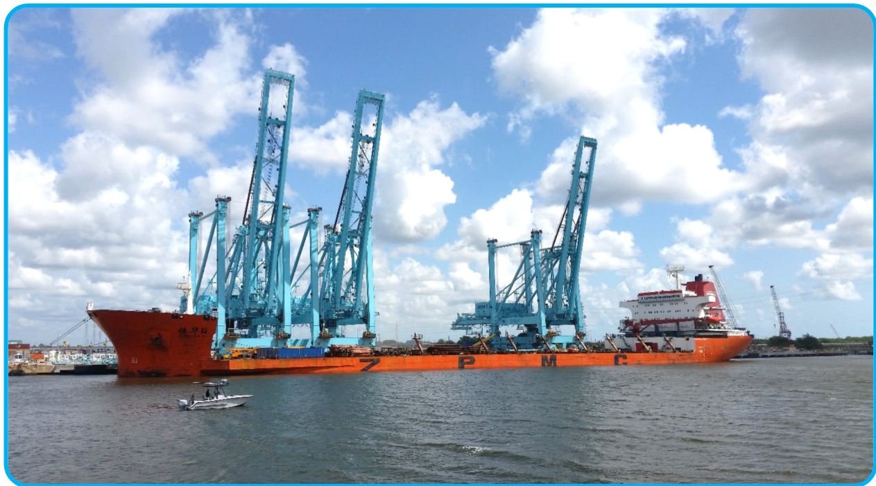
Source: FDOT, Seaport Office Photo (August 24, 2016). Three new Post Panamax cranes delivered at Jacksonville Port Authority.
