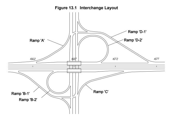
A topographic worksheet for all interchanges is required and will be considered as the preliminary layout of the interchange. This worksheet shall be prepared on a standard plan format on a scale not smaller than 1" = 400'. The following information shall be shown:
