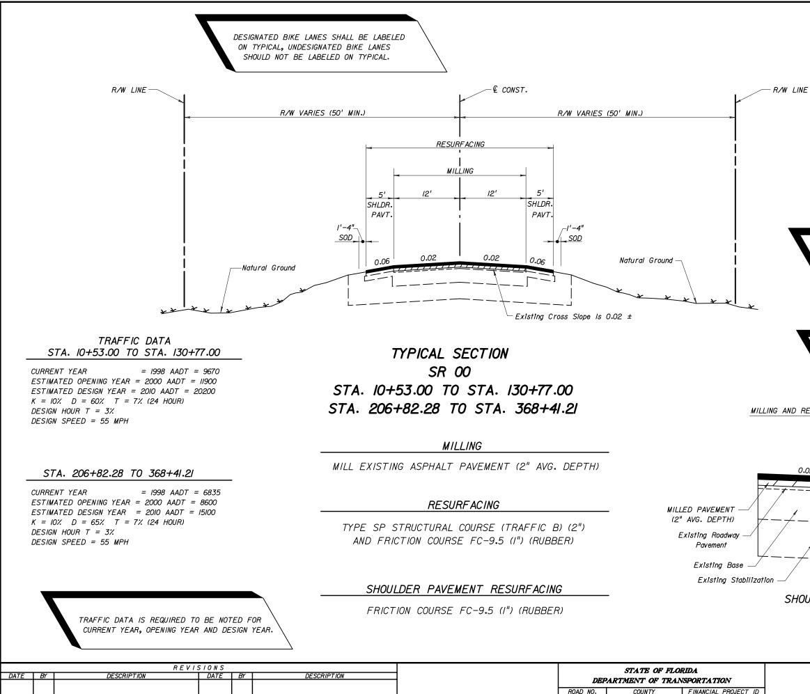
EXISTING 2-LANE (2-WAY) ARTERIAL/COLLECTOR MILLING AND RESURFACING NO CROSS SLOPE CORRECTION REQUIRED UNDIVIDED RURAL (WITH DESIGNATED OR UNDESIGNATED BIKE LANE EXISTING) WITH PROJECTED 20 YR. AADT OF 1500 OR GREATER
