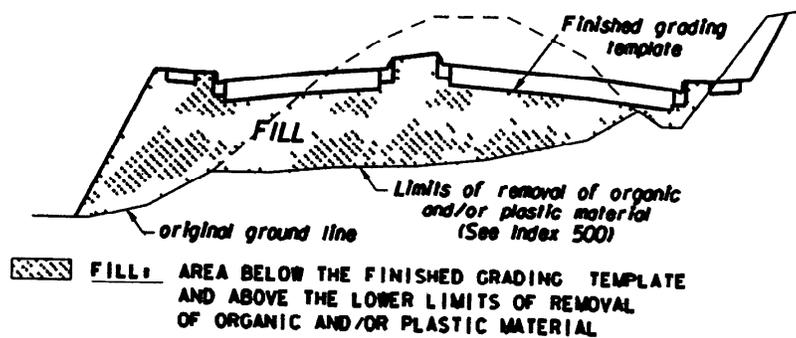
**CUT & FILL DETAILS WITH SUBSOIL EXCAVATION**
