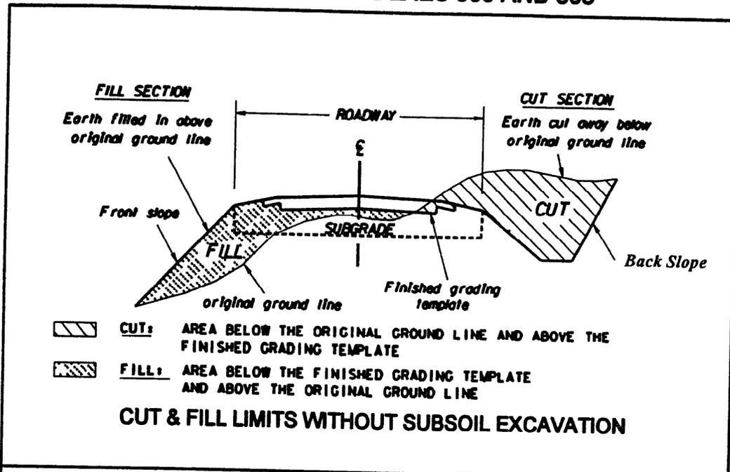
**CUT & FILL LIMITS WITHOUT SUBSOIL EXCAVATION**
