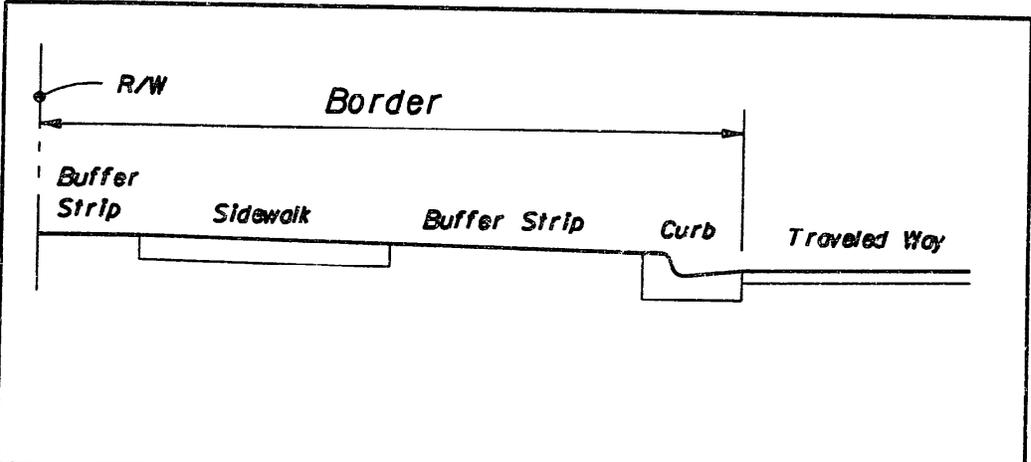
The diagram illustrates the cross-section of a highway border. From left to right, it shows the Right-of-Way (R/W) boundary, a Buffer Strip, a Sidewalk, another Buffer Strip, a Curb, and the Traveled Way. The Buffer Strips are shown as shaded areas between the R/W and Sidewalk, and between the Sidewalk and Curb. The Curb is a raised edge between the Buffer Strip and the Traveled Way.
