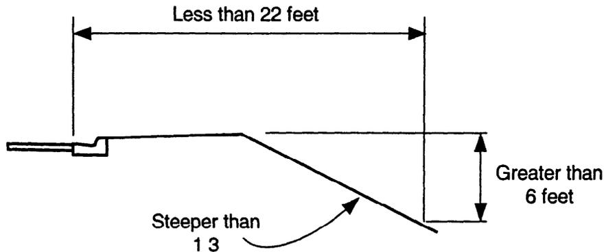
In determining if shielding a drop-off hazard would be feasible for protecting vehicle occupants, the following should be considered:
