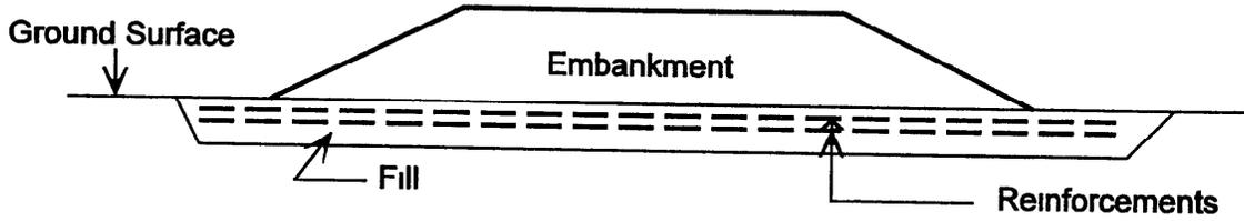
The minimum spacing between two reinforcements shall be 6 inches
