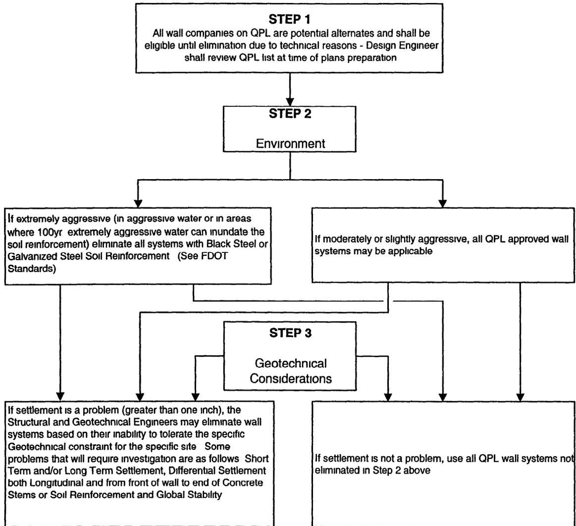
All wall systems not eliminated due to technical reasons shall be noted on the "Control Plans" as appropriate for the site.
