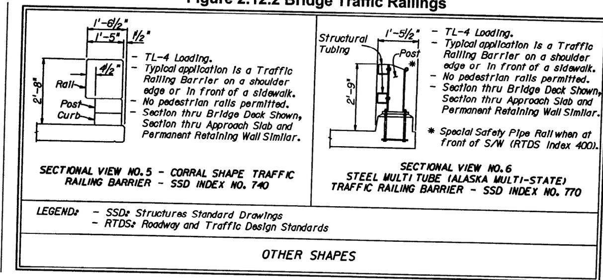
**NOTE:** The steel multi tube railing barrier is only to be used when approved by the District Structures Design Engineer and the District Maintenance Engineer
