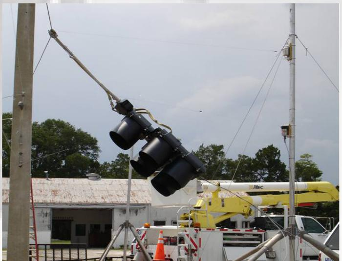
Signals were subjected to wind load testing at the University of Florida.
