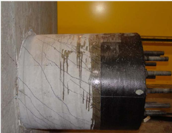
Torsion cracks formed along the length of the test shaft.
