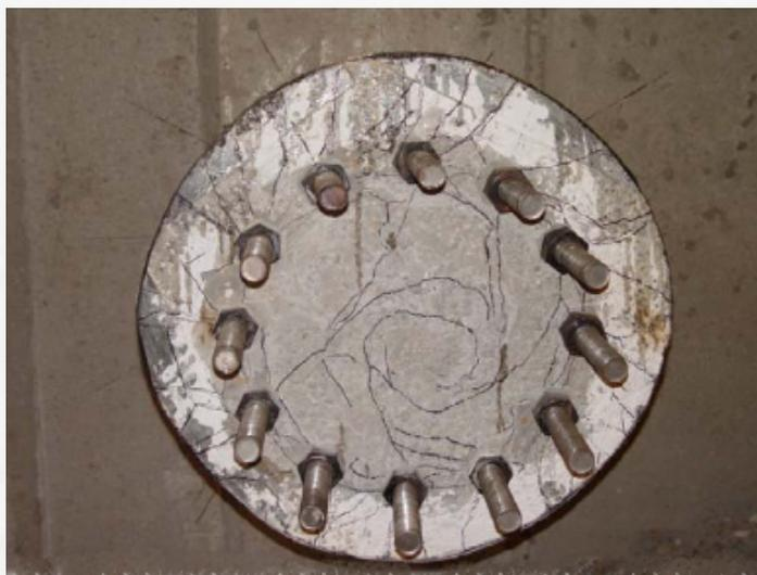
The face of this test shaft illustrates the yielding of bolts, breakout cracks around perimeter, and torsion cracks in center.
