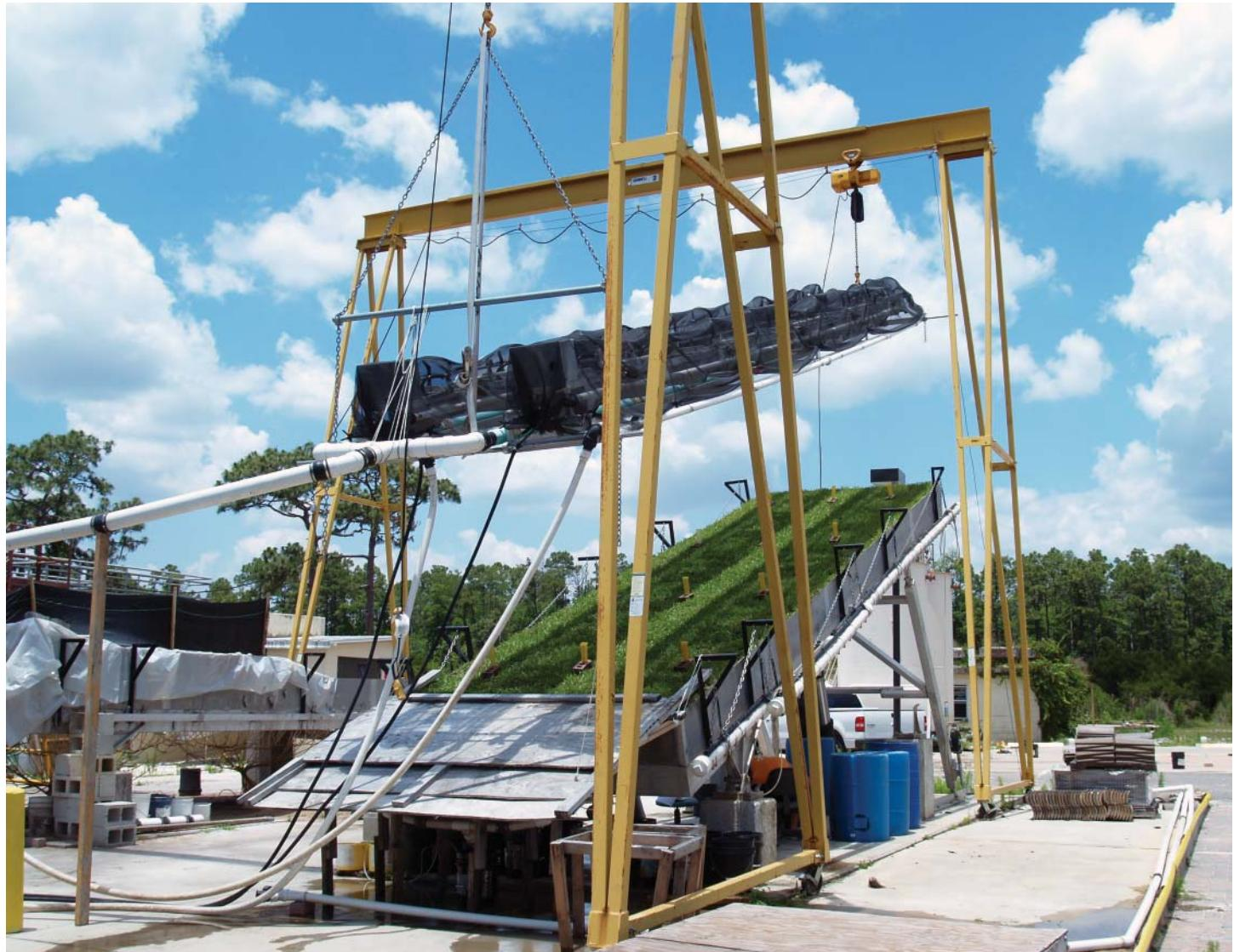
The outdoor rainfall simulator at the Stormwater Management Academy, University of Central Florida in Orlando is the largest in the world and part of the UCF Stormwater Management Academy lab. It consists of an 8-foot-wide by 30-foot-long arrangement of pipes that are connected to a 1,500-gallon water tank. The simulator sprays water onto a bed of sod or soil that can be set at different slopes to study runoff.
