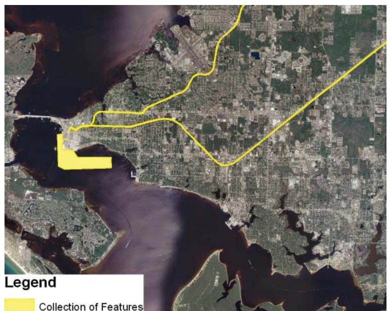
The above screen shot depicts each type of facility (waterway connector, roadway, and railroad) being combined into a single project (pulling lines and polygons into a single layer), which is then analyzed as a whole, resulting in a more accurate estimate of potential impacts at the point where the port, the roadway, and the railroad converge.
