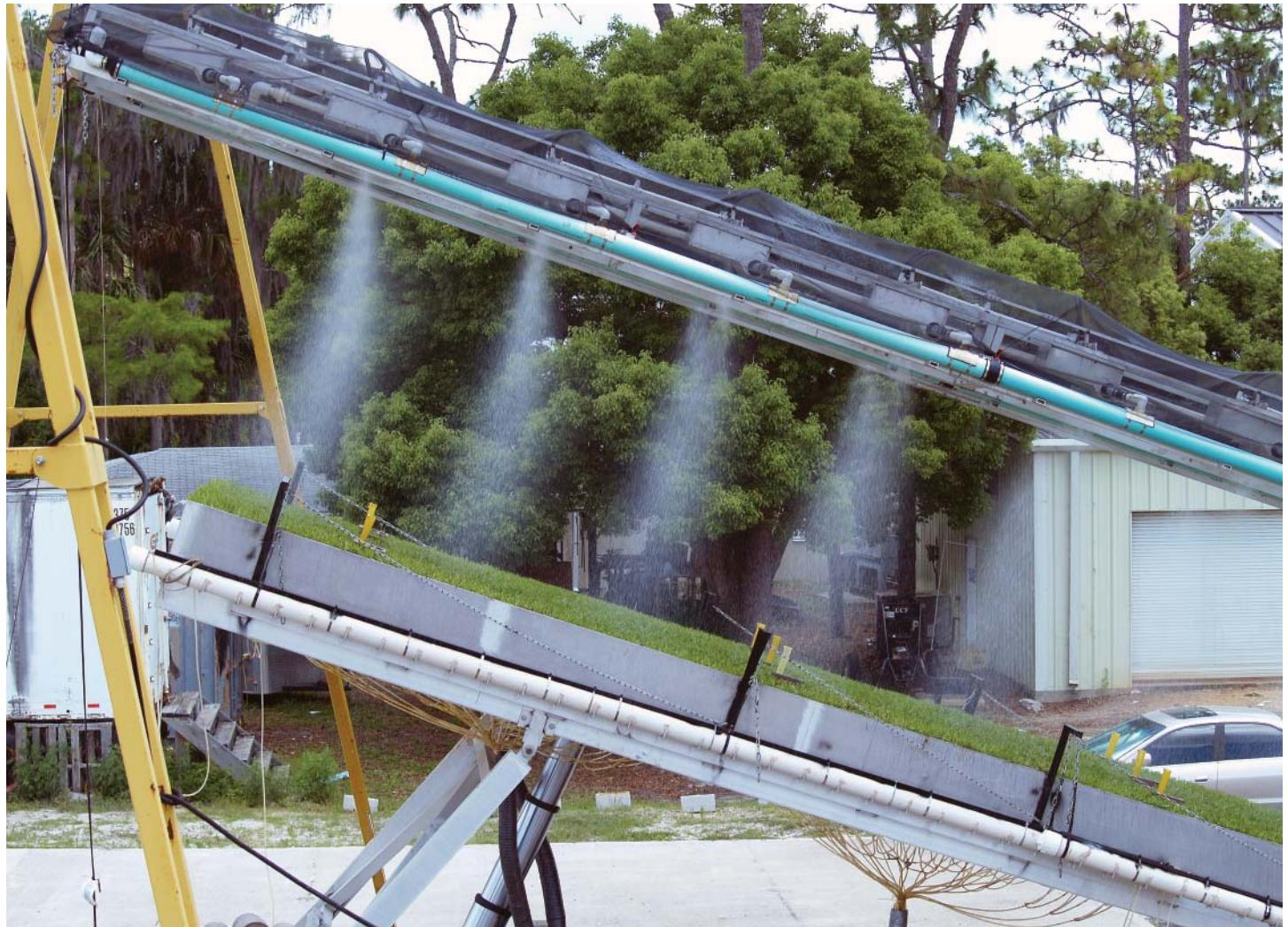
The UCF Stormwater Management Academy rainfall simulator can release up to the equivalent of 20 inches of rain an hour and produce the drop size and intensity of rainfall common to semitropical areas and also northern rainfall. It allows researchers to study how water falls on different surfaces, and how it runs off and dislodges particles that can become sediment, clogging drains and polluting surface and ground waters.
