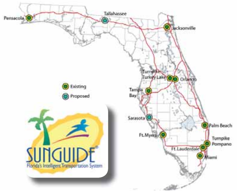
SunGuide®, FDOT's unified software system, enables all ITS devices to communicate with FDOT's regional traffic management centers.
