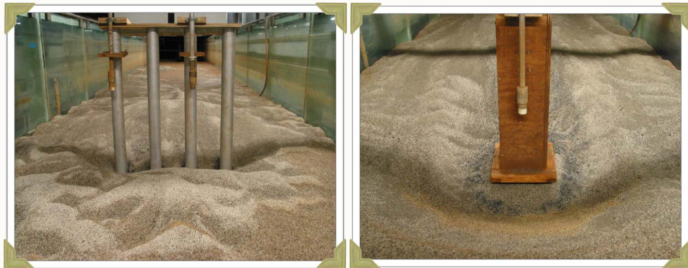
Photos from past research projects show varying levels of scour around both a simple and complex bridge pier structure. (BD545-34)
