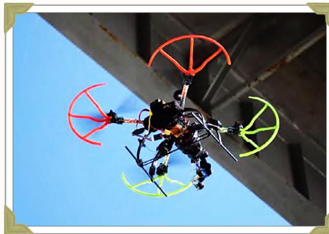
**2014:** Unmanned Aerial Vehicles (UAV) for bridge and high mast luminary inspection bring autonomous and automated technology to the maintenance work of FDOT. (BDV28 977-02)
