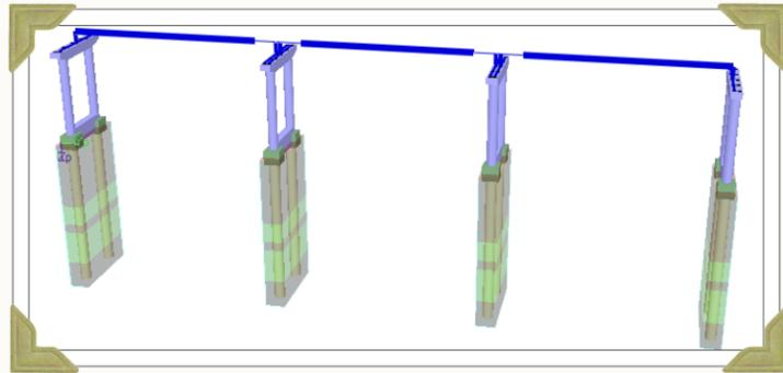
**2014:** FB-MultiPier continues to be improved by FDOT-funded research. This photo shows a multiple-pier bridge model used for a demonstration of dynamic relaxation. (BDV31 977-17)
