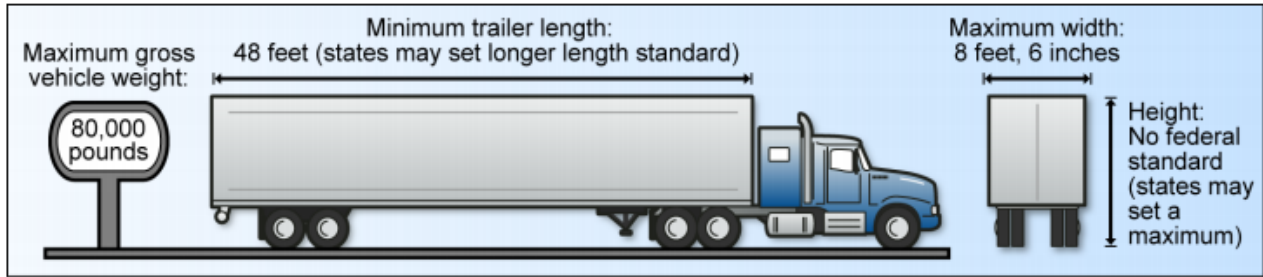
Figure 2-24: Federal Vehicle Size and Weight Standards
