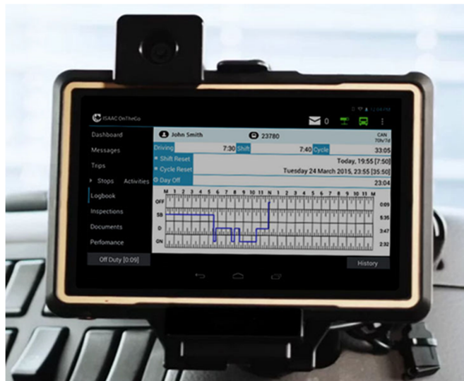
Figure 2-7: An example of an Electronic On-Board Recorder
