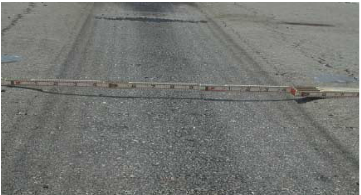
Figure 7.11 Photo of Section 5B (Unmodified Mixture Tested at 50° C)
