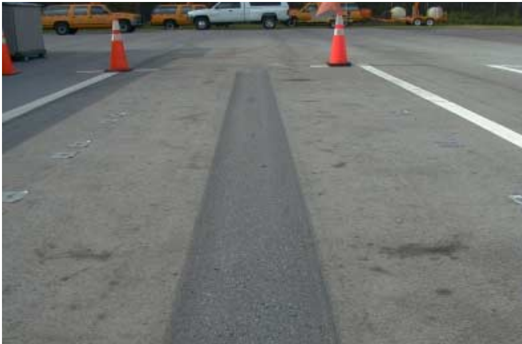
Figure 6.5 Section 2C (SBS-Modified Mixture) after HVS Testing
