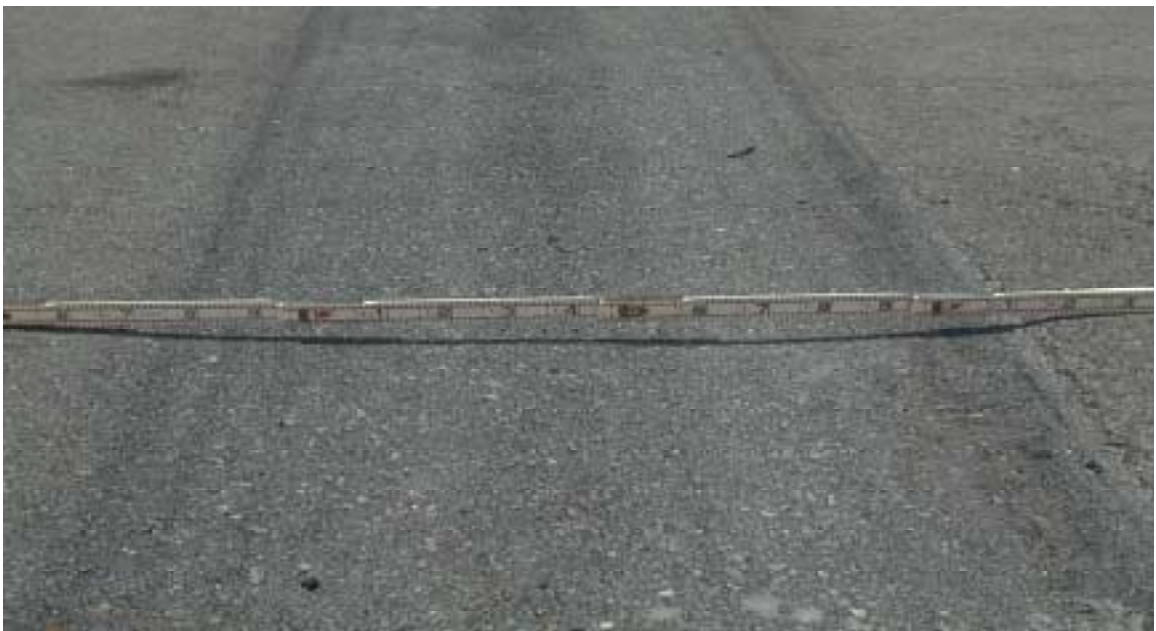
Figure 7.5 Photo of Section 2B (SBS-Modified Mixture Tested at 50° C)
