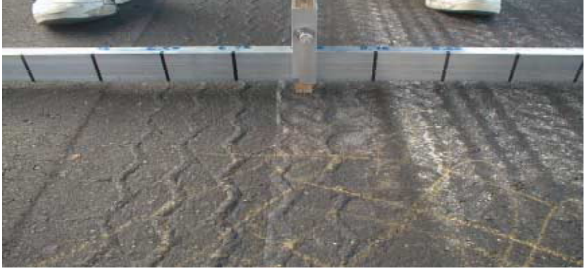
Figure 5.1 Photo of Straight Edge Used for Measuring Rut Depth
