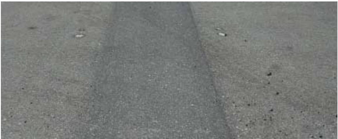
Figure 7.13 Photo of Section 2A (SBS-Modified Mixture Tested at 65° C)
