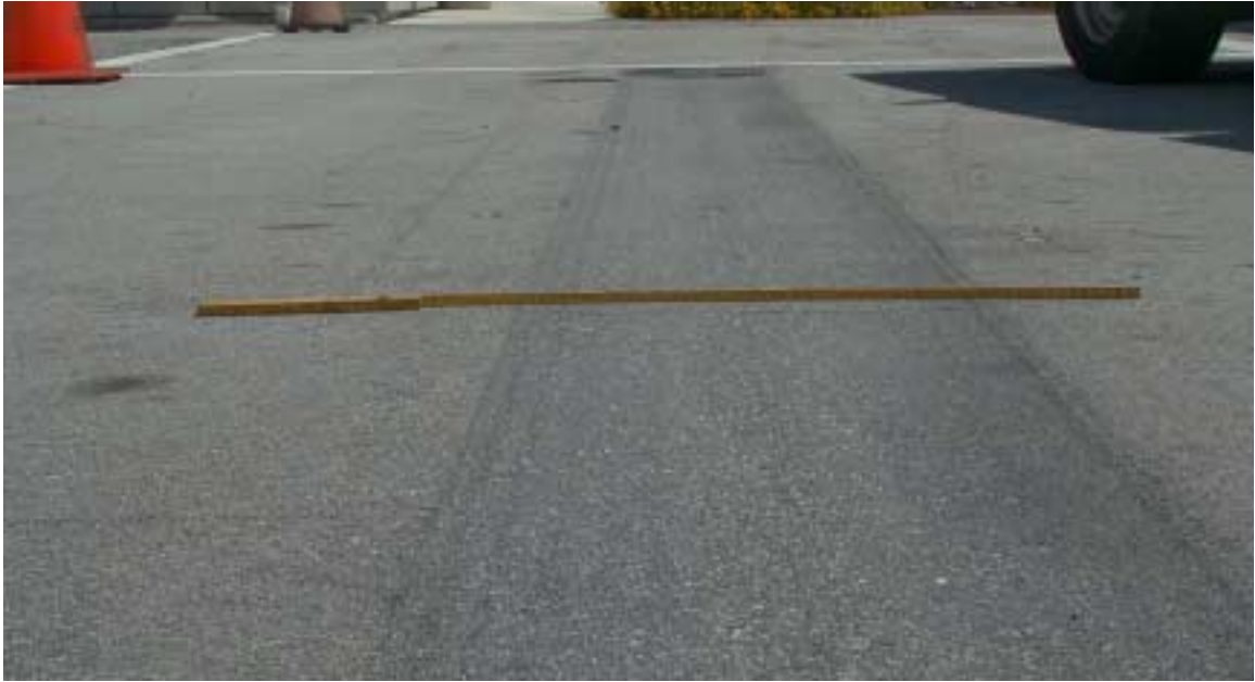
Figure 7.12 Photo of Section 1A (SBS-Modified Mixture Tested at 65° C)
