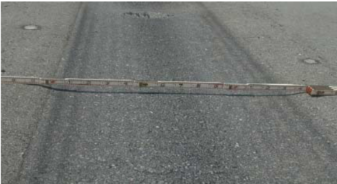
Figure 7.9 Photo of Section 4B (Unmodified Mixture Tested at 50° C)
