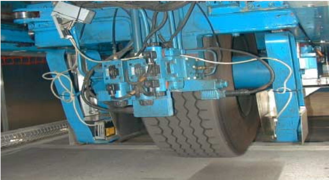
Figure 2.10 Photo of Lasers Mounted onto Two Sides of the Test Carriage
