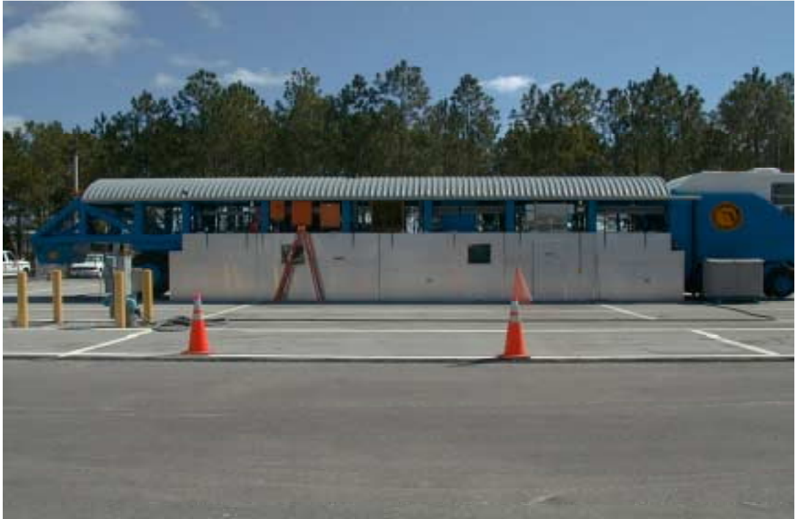
Figure 2.4 Photo of Sidewall-Paneled HVS
