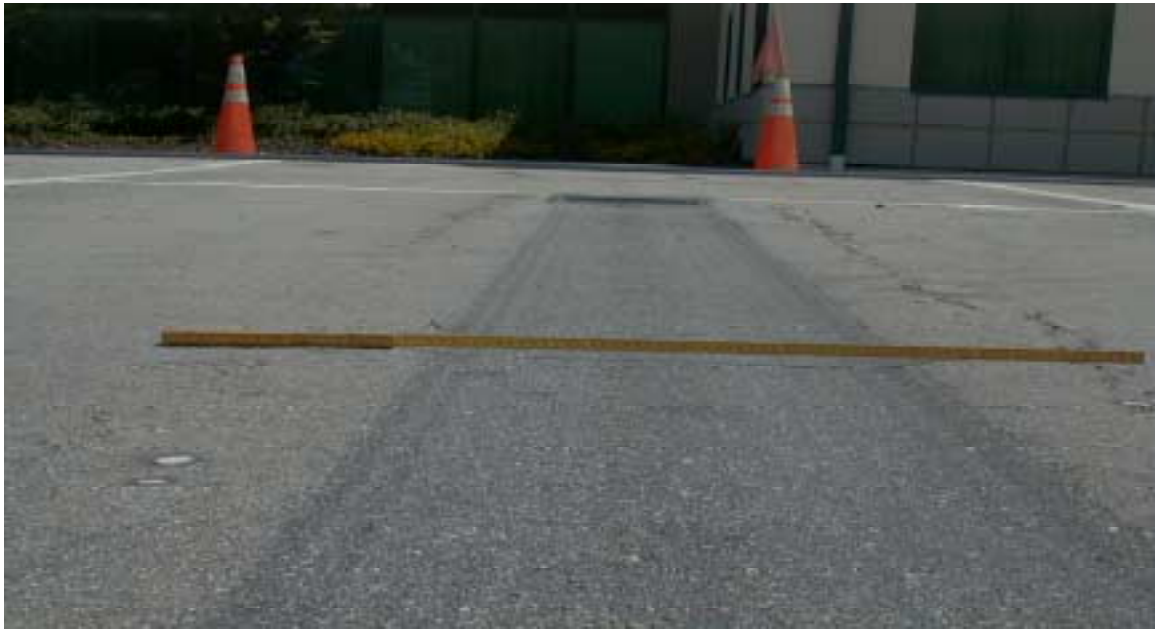
Figure 7.8 Photo of Section 4A (Unmodified Mixture Tested at 50° C)
