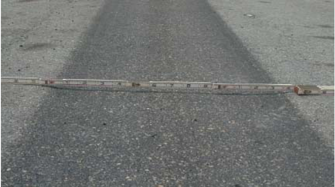
Figure 7.6 Photo of Section 3A (SBS-Modified Mixture over Unmodified Mixture Tested at 50° C)
