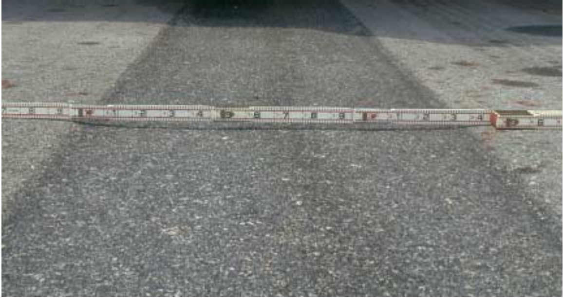
Figure 7.4 Photo of Section 1B (SBS-Modified Mixture Tested at 50° C)
