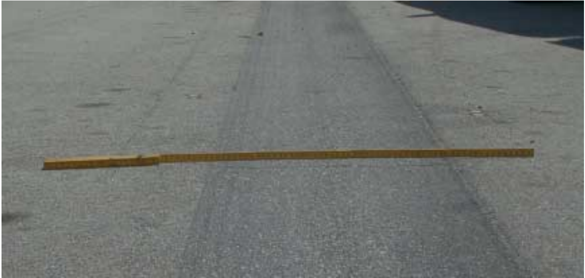
Figure 7.10 Photo of Section 5A (Unmodified Mixture Tested at 50° C)
