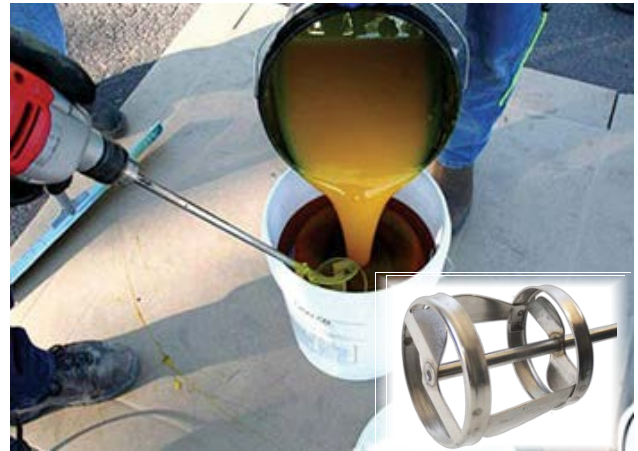
FIGURE 10 – Electric mixer with “Jiffy Mixer” attachment.
