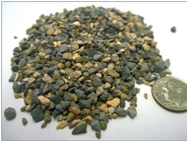
FIGURE 4 – Calcined bauxite, crushed and graded.
