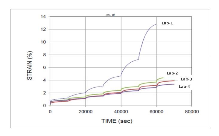
Lab-1 used load cell to control the applied force. Others used dead load to apply the force to the specimen
