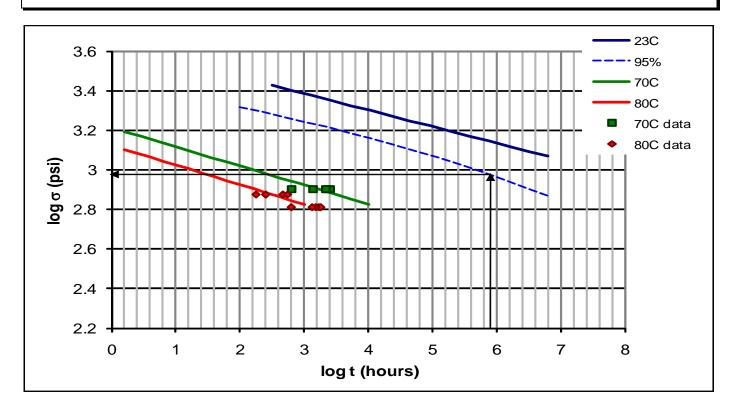
The 100-year tensile strength for corrugated HDPE pipe is predicted to be 800 psi.
