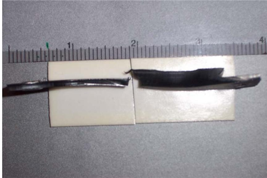
Fig. 2.7 – Failure of junction-specimen from pipe P-2
