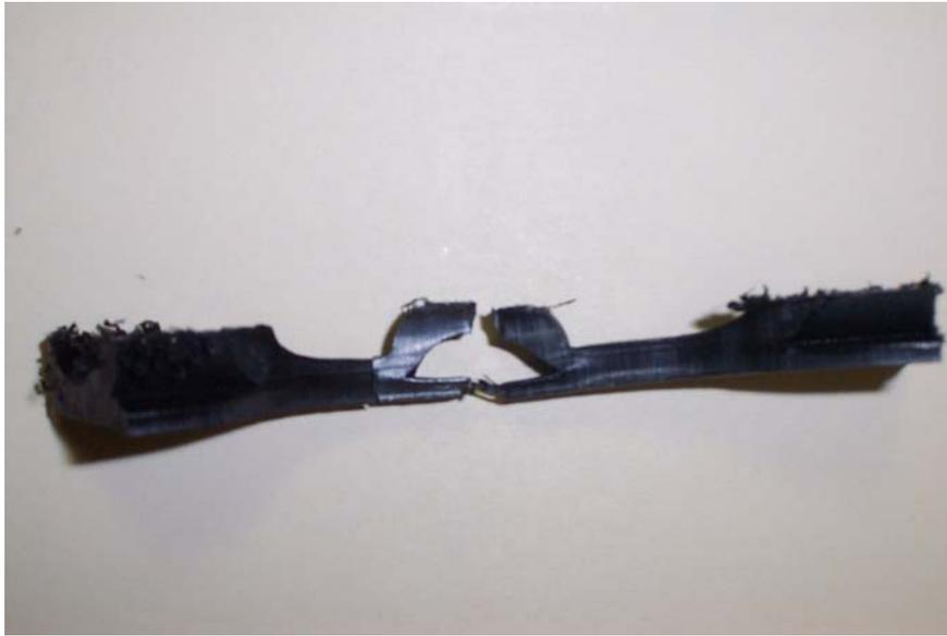
Fig. 2.9 – Failed longitudinal profile (vent hole) specimen
