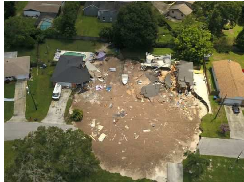
Massive sinkhole (250 x 220 x 50 ft) damaged 2 homes in Land O'Lakes, FL (July 14, 2017)
