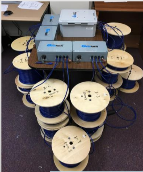
Step 1: Checking sensors and dataloggers in lab
