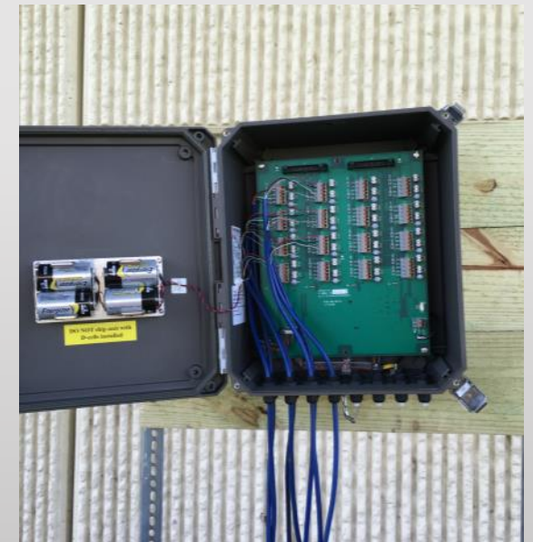
Step 4: Connect sensors to datalogger and start logging
