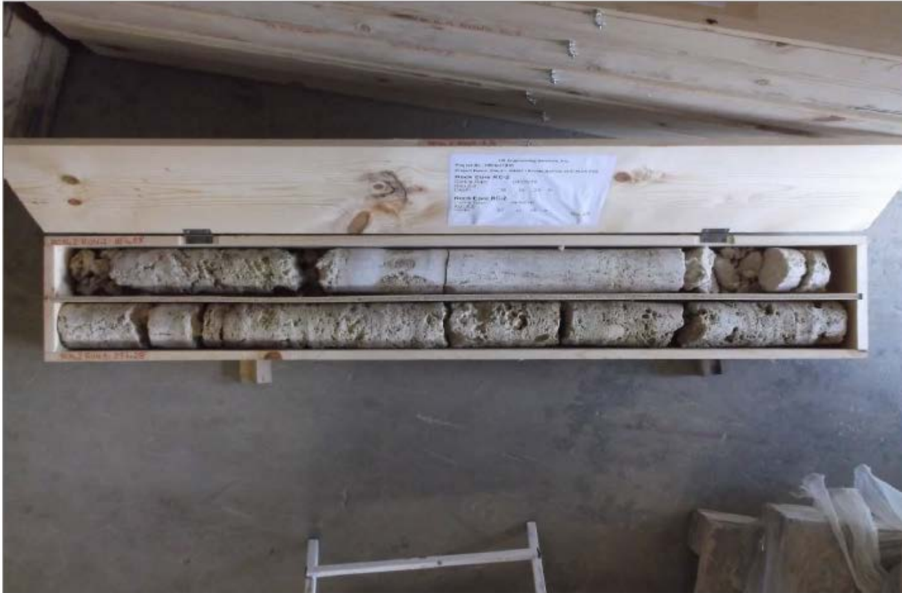
Rock Core No. RC-2 Runs No. 4 and No. 5
