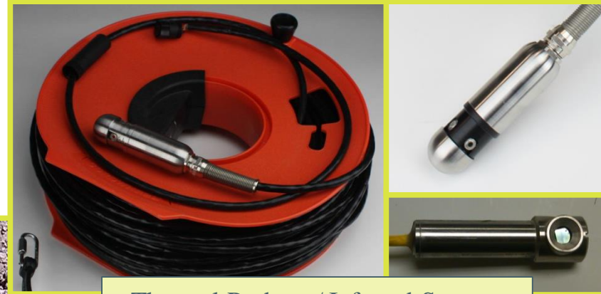
Thermal Probe w/ Infrared Sensors
