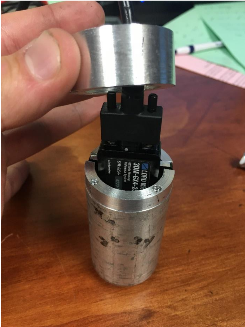
Specially fabricated probe body to house IMU sensor
